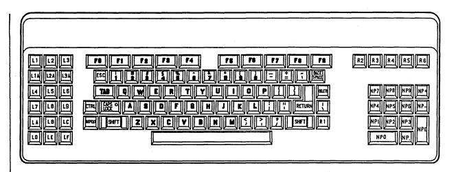
Figure 1-1. The Low-Profile Model II Keyboard Map
