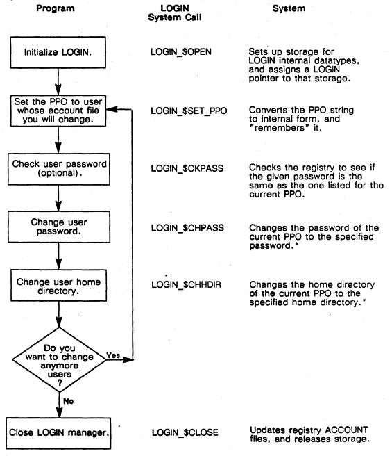
\* Note that changes are not finalized until LOGIN\_\$CLOSE closes successfully. Figure 3-1. Using LOGIN System Calls in Proper Sequence
