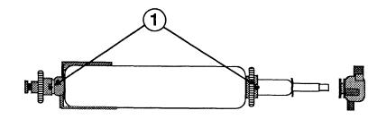
*Note:* There is no paper-empty frame (Figure 36, #1) when an optical paper-out sensor is installed.
