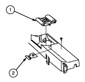
Reassembly – Part 1 Optical Assembly
