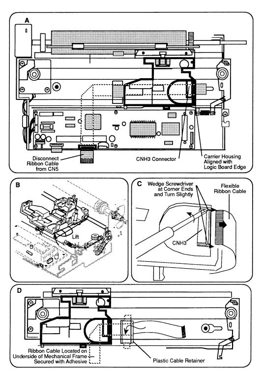
Figure 2-13 Flexible Ribbon Cable
