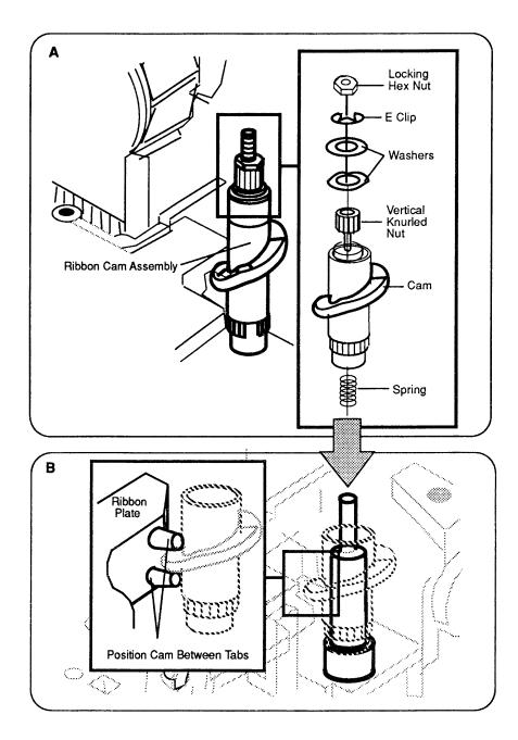
Figure 2-7 Ribbon Cam Assembly
