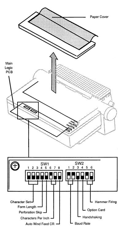
Figure 1-9 DIP Switches
