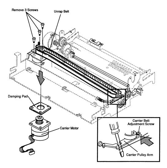
Figure 2-18 Carrier Motor
