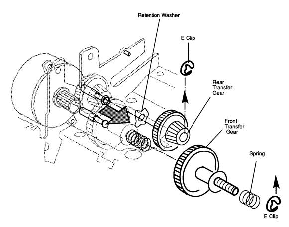
Figure 2-24 Transfer Gears
