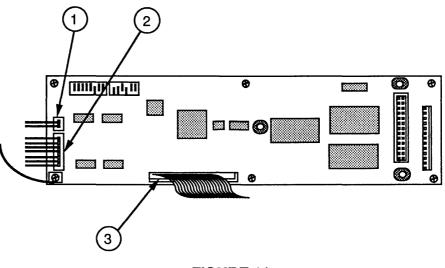
12. Remove the old mechanical paper-sensor ground screw (Figure 12, #1) from the left platen bushing plate and discard the screw.
