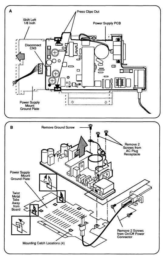
Figure 2-15 Power Supply Board
