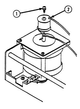
14. Use a Phillips screwdriver to remove the screw (Figure 23, #1) from the top of the motor pulley.
