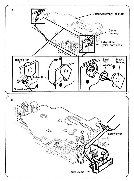
Figure 2-8 Carrier Assembly Top Plate
