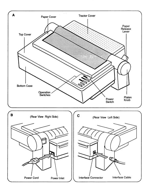
Figure 1-1 Unit ID, Power/Interface Cables
