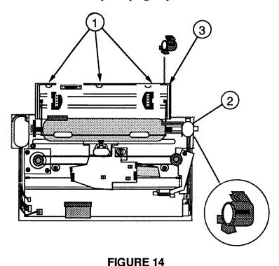
17. Pull off the black plastic friction/tractor adjustment piece (Figure 14, #2) from the right side of the platen and place it between the frame and the printer case just above the transformer (Figure 14, #3). This piece will act as a wedge and will support the mechanical assembly at the height necessary to perform the remaining steps of this procedure. The long leg that fits down into the paper friction gears will rest on the back side of the plastic case.
