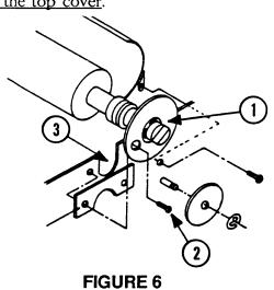
On the right side of the platen, rotate the paper feed gear (Figure 6, #1) until the hole in it lines up with the platen shaft holder screw (Figure 6, #2). Remove the screw and the platen shaft holder.
