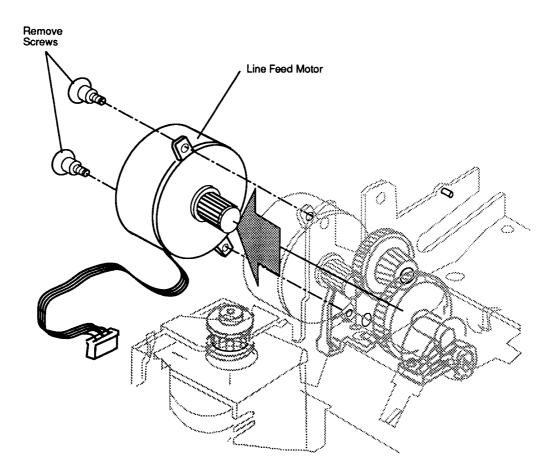
Figure 2-17 Line Feed Motor
