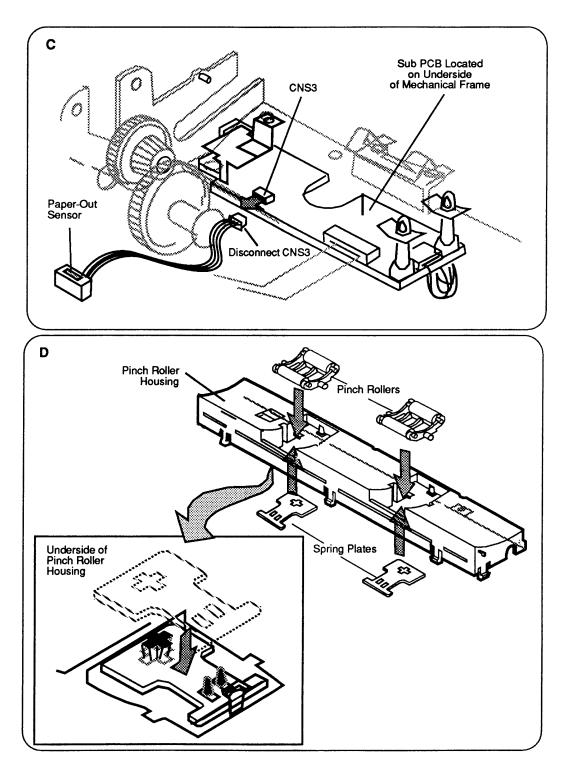
Figure 2-22 Pinch Roller Assembly (Continued)
