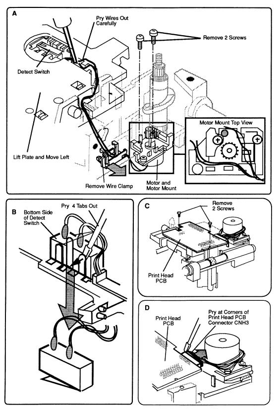
Figure 2-28 Ribbon Motor and Detect Switch
