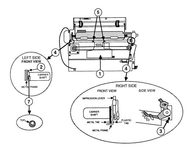
6. Place the carrier cam on the left side of the carrier shaft. Be sure to position it as shown in Figure 33, #7, with the smaller section as the top of the cam. The wrong position will produce uneven printing.
