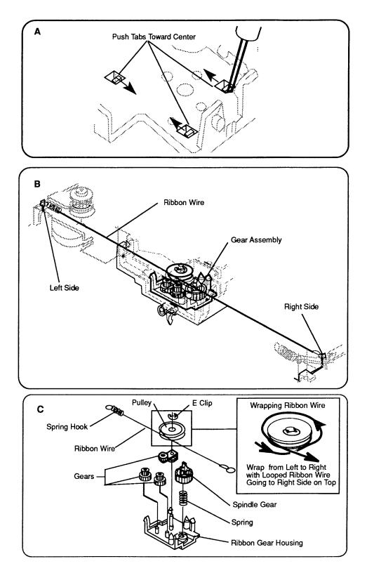
Figure 2-9 Ribbon Wire and Gear Assembly
