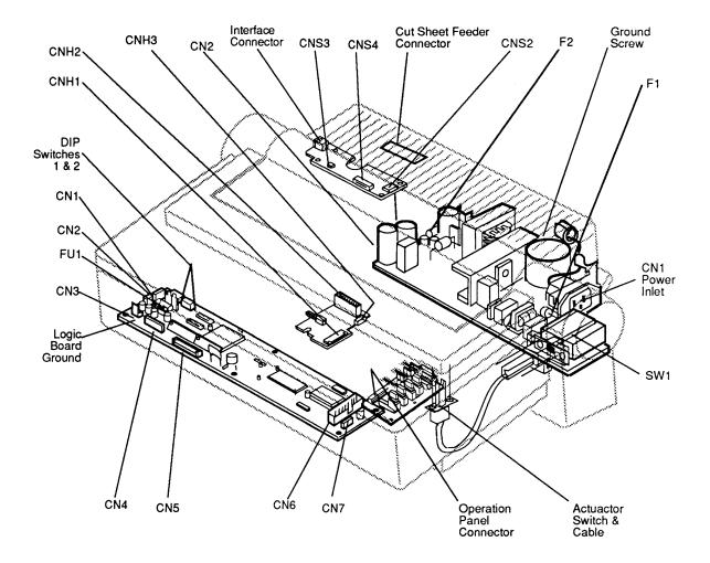
Figure 1-4 Connector and Fuse Locations
