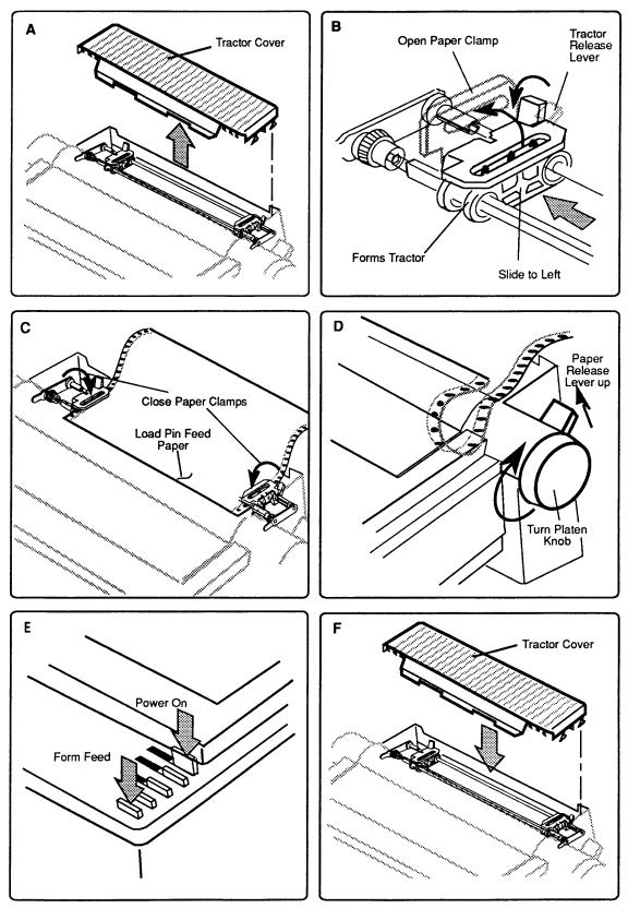
Figure 1-6 Loading Pin-Feed Paper
