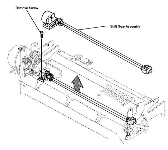
Figure 2-23 Shift Gear Assembly
