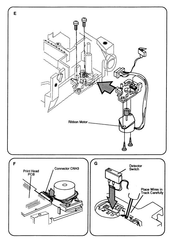
Figure 2-28 Ribbon Motor and Detect Switch (Continued)
