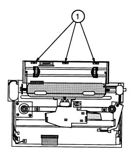
8. On later models, lift up the front of the frame and pull it toward you until it is completely out of the plastic portion of the bottom cover. If the frame does not clear the top rear of the bottom cover, push slightly at the top of the back edge above each of the three molded plastic frame holders (Figure 47, #1) of the bottom cover.
