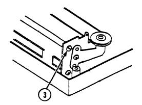
11. Remove the screw (Figure 22, #3) on the right end of the shaft.
