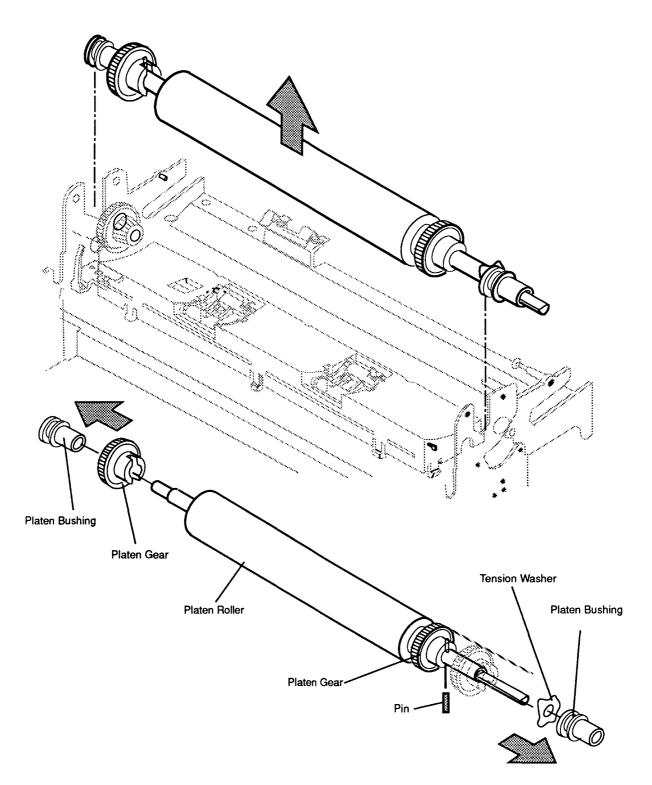
Figure 2-20 Platen Roller and Gears
