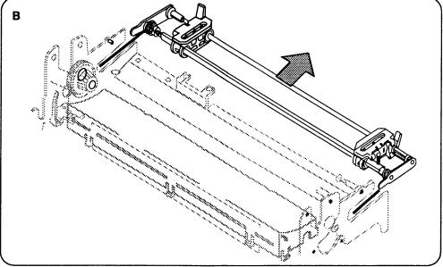
Figure 2-21 Tractor Assembly
