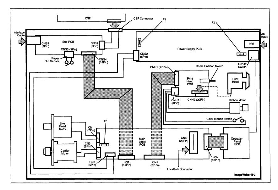
Figure 1-13 Block Diagram
