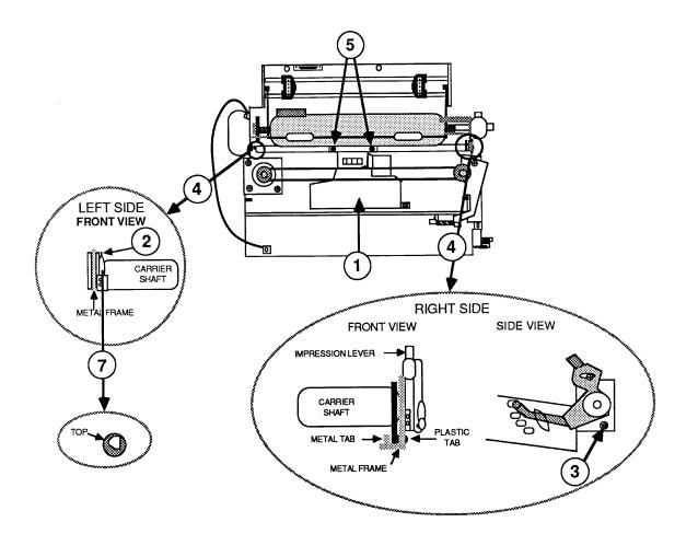
6. Place the carrier cam on the left side of the carrier shaft. Be sure to position it as shown in Figure 33, #7, with the smaller section as the top of the cam. The wrong position will produce uneven printing.
