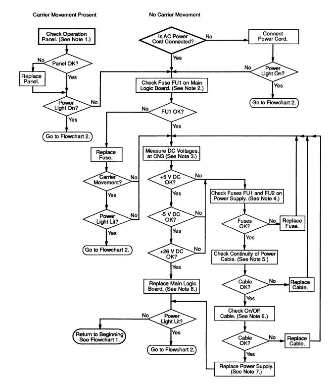
Notes for Flowchart 2: Power Light On, No Printing, Does Not Run Self-Test
