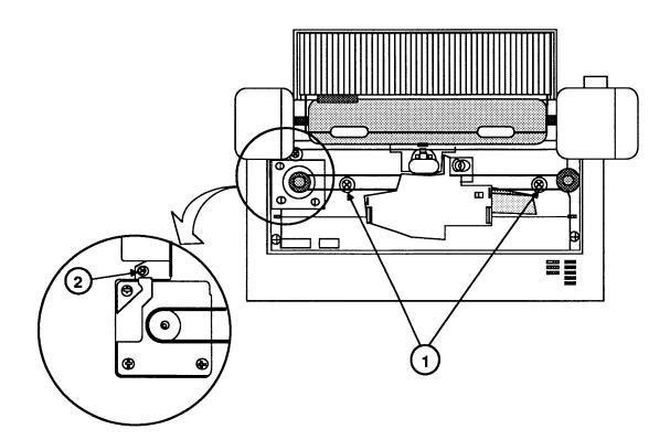
7. If there is a screw (Figure 46, #2) between the stepper motor and carrier motor housing, remove it.
