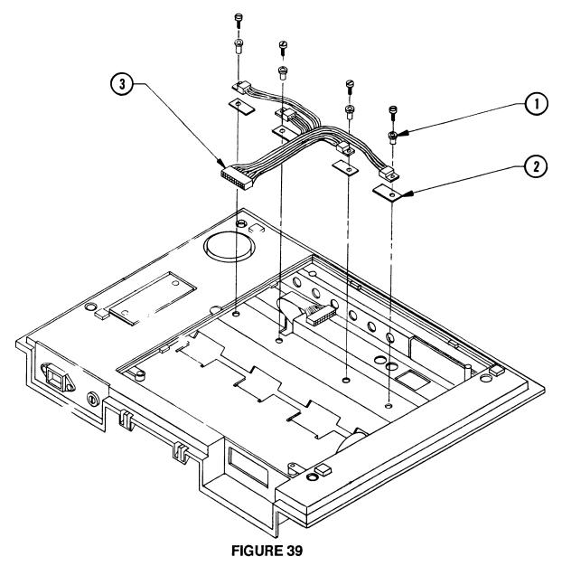
3. Use the Phillips screwdriver to remove the four carrier drive transistors.
