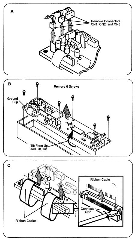
Figure 2-5 Main Logic Board
