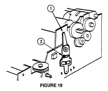
2. If the print darkness is uneven, loosen the impression control lever adjustment screw (Figure 19, #2), and move the impression control lever (Figure 19, #1) until the print darkness is equal at the top and bottom of characters. Tighten the screw when the adjustment is complete.
