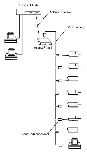
Figure 2-7 Example of a 10BaseT Ethernet configuration
