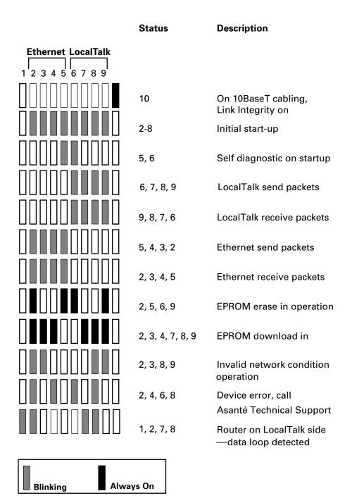
Figure 2-9 Display status LEDs
