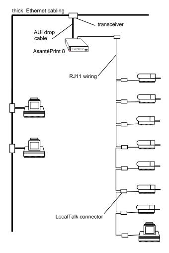
Figure 2-3 Example of a thick Ethernet configuration
