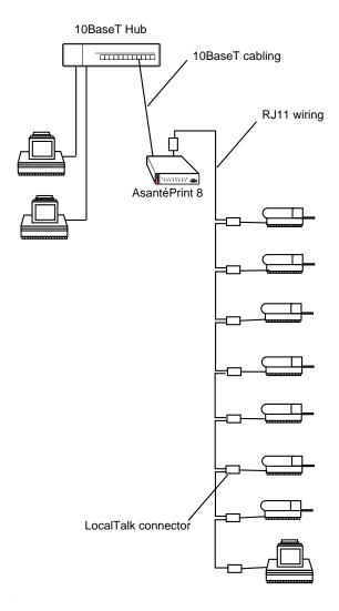
Figure 1-1 Example of a 10BaseT Ethernet configuration
