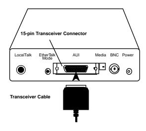
Figure 2-2 Connecting the 15-pin transceiver to the AsantéPrint unit
