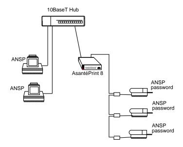
Figure 4-1 Example of two Macintosh computers on the Ethernet with ANSP installed
