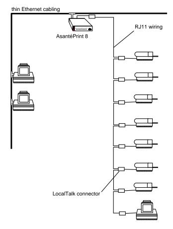
Figure 2-5 Example of a thin Ethernet configuration
