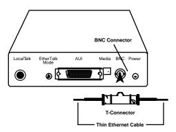
Figure 2-4 Installing the T-connector onto the AsantéPrint BNC connector
