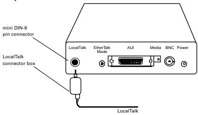
Figure 2-8 Connecting the LocalTalk connection box
