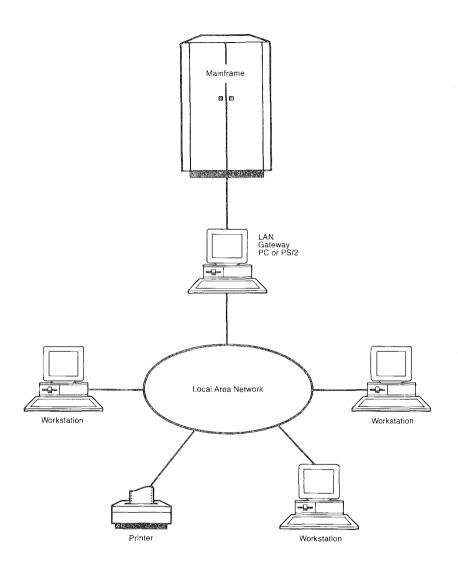
With the gateway, the PC workstation is connected to the mainframe and performs the functions of a 3X74 control unit.
