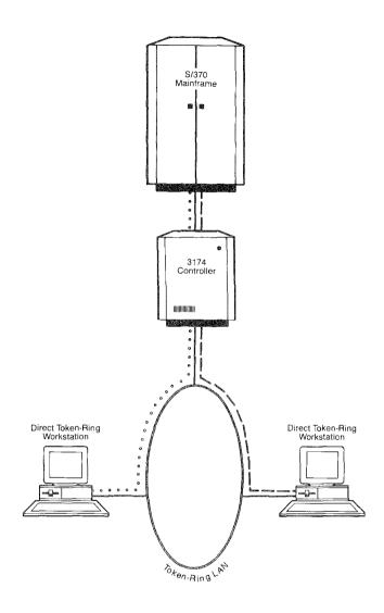
Direct token-ring workstations can be connected to the mainframe through a 3174 Controller.
