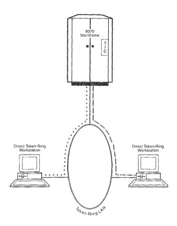
Direct token-ring workstations can be connected directly to a 9370 mainframe.
