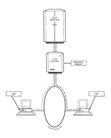
Direct token-ring workstations are identified through LAAs. The destination address you enter at the workstation identifies the LAA of the mainframe communications device.
