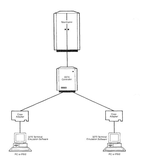
The 3270 coax connection links a PC or PS/2 to a 3X74 control unit.
