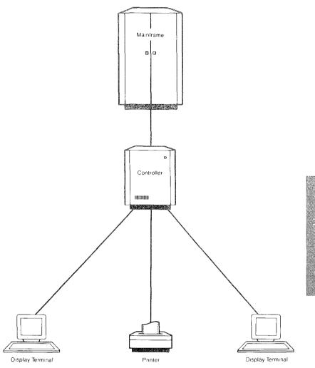
Display terminals, printers, control units, and mainframes are the major components of a 3270 network.
