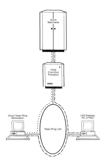
This token-ring workstation can communicate with the mainframe both as a LAN workstation and as a token-ring DLC workstation.
