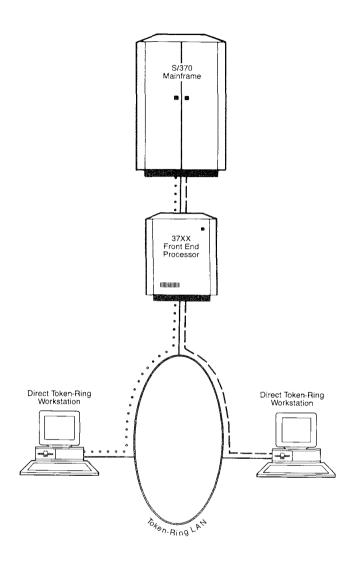
Direct token-ring workstations can be connected to the mainframe through a 37XX Front End Processor.
