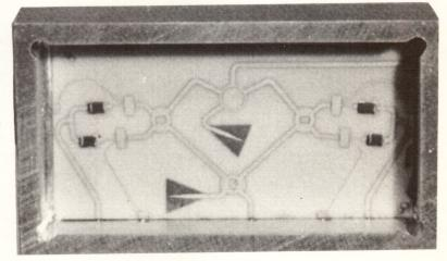
\*Extremely narrow deposited metal "stripline" conductors, especially useful in microwave applications, where the relationship of physical dimensions of circuitry vs wavelength becomes meaningful to circuit performance.
