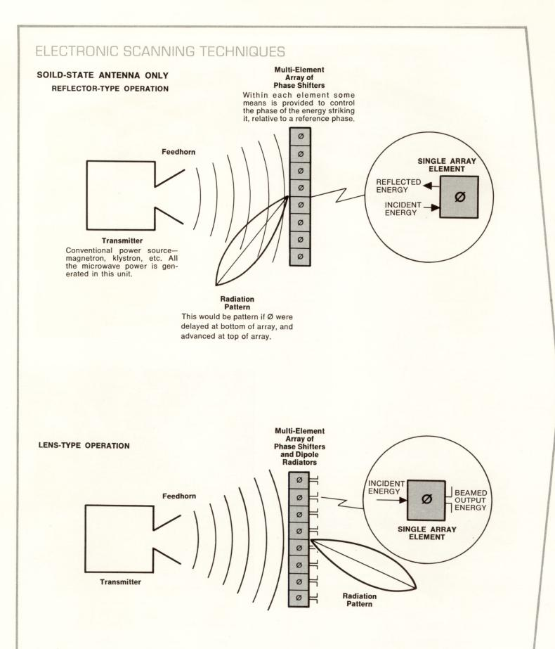
Lens-type operation has advantage in that the transmitter does not shadow or block the antenna array, and the entire surface of the array is available for radiating the beam.
