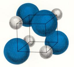
positively charged cores of the atoms (black). In a solid with ionic bonds, typified here by sodium chloride (right), the binding electrons are outermost electrons of both the positively charged sodium ions (black) and the negatively charged chlorine ions (color).
