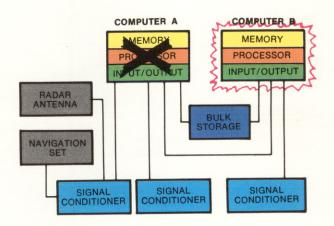
The system still continues to operate, but in a degraded mode. Further degradation of the system can occur with the mission objectives still being accomplished as long as Computer B continues to operate.
