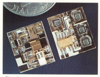
Films of inactive material are deposited on glass to make up a thin-film circuit's conductors, resistors, and capacitors. Separate "discrete" transistors, diodes, and even whole uncased IC's are bonded to the deposited network.
