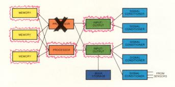
If a processor should cease operating, a new path is selected, and the system continues to perform its tasks.
