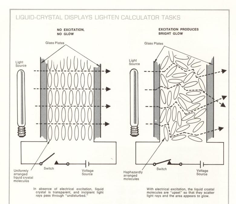
In LCD's being mass-produced by Rockwell International for MOS/LSI calculators, 7-segment digits are used. Each digit is  $\frac{1}{2}$ -inch high and is formed by applying tin oxide—a transparent electrical conductor—on the insides of two glass plates. The two plates are separated by a space of only around one-third the thickness of a human hair (about 1/1000 inch), and this space is filled with liquid crystal.
