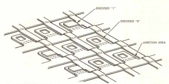
The lower set of conductors is silicon, the upper aluminum. Tabs in silicon contain diodes; contact is made through similar tabs on the aluminum layer.
