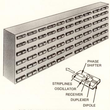
ONE CONCEPT OF A SOLID-STATE, PHASED-ARRAY, MULTIPURPOSE RADAR
