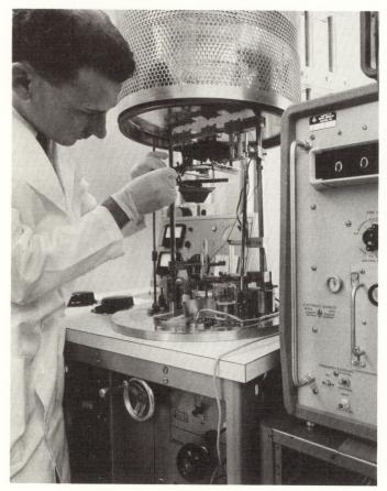
Hood of vacuum chamber raised, engineer puts masked thin-film substrate into place. Monitoring equipment (right) gives vacuum, temperature, and deposition data, as vapor from heated metals rises to form circuit.
