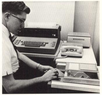
**Computers "Talk Back" to Questioning Engineers** A Rockwell engineer uses a SCAN-TRAC "conversational" computer terminal for high-speed remote entry of his circuit design problems. If he's not in a hurry, the engineer can input his problem at the end of the work day and pick up the answer next morning. For urgent situations, access via the terminal to the central computer, as well as the computer's response, can be immediate. SCAN-TRAC terminals are located throughout prîncipal design areas.
