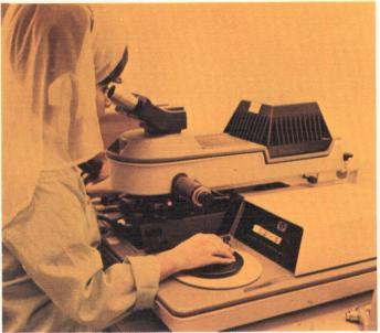
Oxide is selectively removed for each diffusion by exposing the photo-resist-coated slice to ultraviolet light through the appropriate mask from the device mask set, desealing the unpolymerized photo-resist, and selectively etching the oxide exposed by the "windows" thus opened. Position of each mask is precisely aligned relative to others in the set by means of a microscope and electromechanical alignment system.
