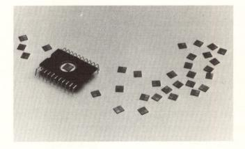
Rockwell International Has Designed Basic One-Chip Calculator Circuits which it "micro-programs" to produce varieties of unique machines. Millions of these circuits, which include "electronic sliderule" versions, have been delivered.
