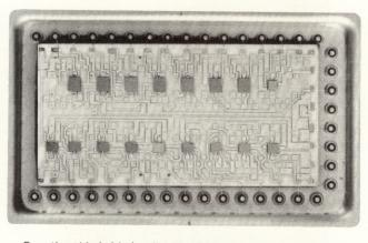
Functional hybrid circuit with 17 flip-chip bonded devices
