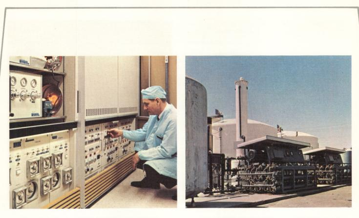
Manufacturing engineer adjusts power levels for diffusion furnaces. Other adjustments set furnace temperature, pressure, and gaseous flow-rates.
