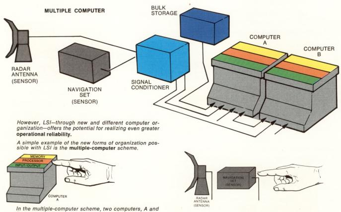
In the multiple-computer scheme, two computers, A and B, have separate memory, processor, and input/output sections.
