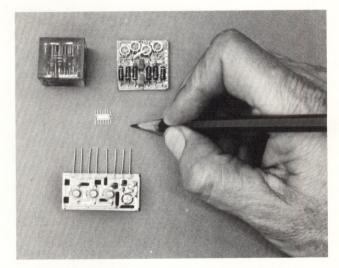
Four first-generation approaches to microminiaturizing a flip-flop circuit are grouped to give a comparison of relative sizes. At upper left is a plastic-encapsulated package of discrete components, while at upper right is a thin-film device. The ceramic printed circuit version of the flip-flop is at bottom of the picture, and the integrated circuit is at center. All four approaches perform the identical flip-flop function.
