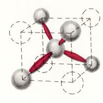
**ELECTRONS INVOLVED** in luminescence in most semiconducting solids are the binding electrons that hold the crystal lattice together. In a solid with covalent bonds, typified here by germanium (left), these binding electrons form negatively charged clouds (color), between the
