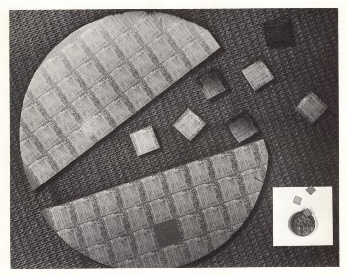
**Heart of Skid Trol** is its digital "computer" with 2,000 MOS transistors on a single "chip" of silicon about the size of a match head. The computer is encased in the Skid-Trol pneumatic valve. One valve is used on each axle of the truck, tractor, or trailer. A sensor within each wheel reads the wheel speed and gives this information
