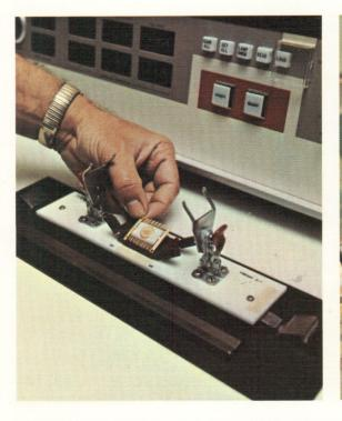
To test strength of completed-device outgoing leads, the devices are placed, with leads outward, around the periphery of a high-speed centrifuge. At full speed of the system, the leads are subjected to a centrifugal pull of thousands of g's.
