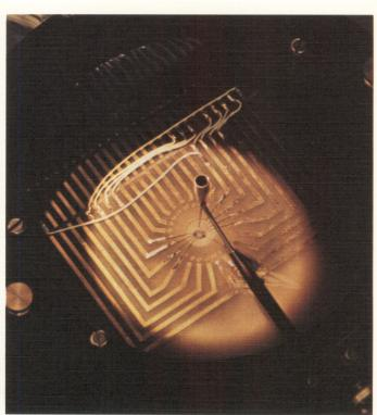
Production test probe checks every circuit on each MOS/ LSI wafer and feeds signals into a computer which compares them with those for a "perfect" circuit. (Only those arrays whose circuits check "100% perfect" when tested in this way are accepted by Rockwell's Microelectronic Device Division.)
