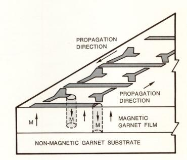
With the bubble memory approach, data are stored within magnetic domains contained in thin films of single-crystal garnet materials epitaxially grown on a nonmagnetic, singlecrystal garnet substrate.
