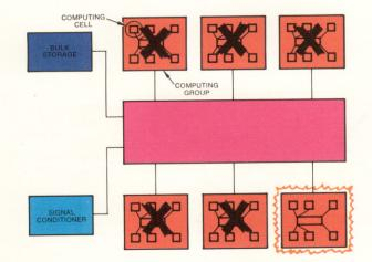
The distributed processor computer systems could be designed in such a way that, with only one computing group left operating, the system could still meet its mission objectives, although in a degraded mode.
