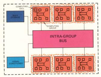
The computing groups are, in turn, connected through a "bus" to form the complete computer.
