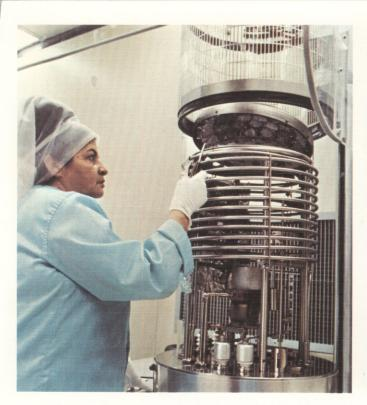
Circuit intraconnections can be made by depositing aluminum on the MOS slices, followed by selective etching to leave only the desired intraconnection pattern.
