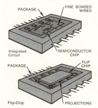
COMPARISON OF THE CONVENTIONAL METHOD FOR CONNECTING IC TO PACK-AGE AND THE FLIP-CHIP TECHNIQUE
