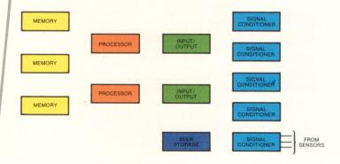
A further refinement of the multiple-computer concept is the **multiprocessor**.
