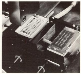
Semi-Automatic Die Placement Machine For Digital Microcircuits
