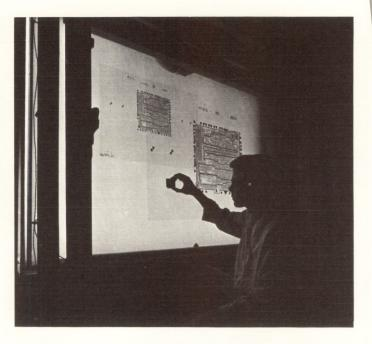
The many-times-ultimate-device-size masks made by the plotter are photographically reduced to form a 1-timessize production mask set. Each mask in the set typically contains hundreds of identical circuit patterns. MOS design engineering delivers to a MOS production facility: release drawings, mask sets and process specifications.
