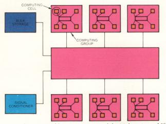
A concept with an even greater defect-tolerant capability than the multiprocessor is the **distributed processor** scheme. While such a system may involve additional cost, it offers many levels of reconfiguration to attain even greater operational reliability.
