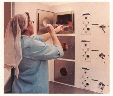
Wafers are inserted into diffusion furnaces for growth of oxides to serve as device gate and insulation, and for diffusion of source and drain.
