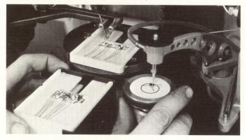
Discrete components are resistance-soldered to screened resistor-conductor networks on ceramic substrates to form ceramic printed circuits.
