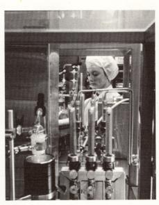
"Glass jungle"—valves, metering devices, heating elements—for mixing and distributing furnace and dopant gases.
