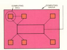
In the distributed processor scheme, one chip or computing cell performs a significant and complete subtask. Several of these cells are hooked in parallel to form a computing group.
