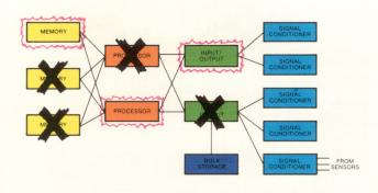
The multiprocessor system could lose many more sections than the multiple-computer scheme and still meet its mission objectives.
