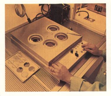
Photo resist is applied evenly over the surface of rotating wafers.
