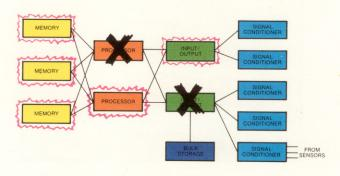
If an input/output section ceases to function, again the system is reconfigured.
