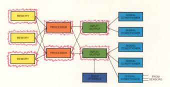
In the multiprocessor scheme, the memory units, processors, and input/output sections of the computers are all interconnected.
