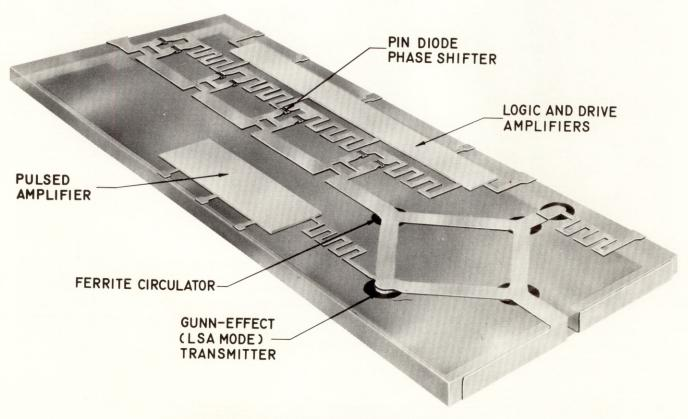
CONCEPT FOR A SINGLE-SUBSTRATE (SAPPHIRE) SOLID-STATE RADAR MODULE
