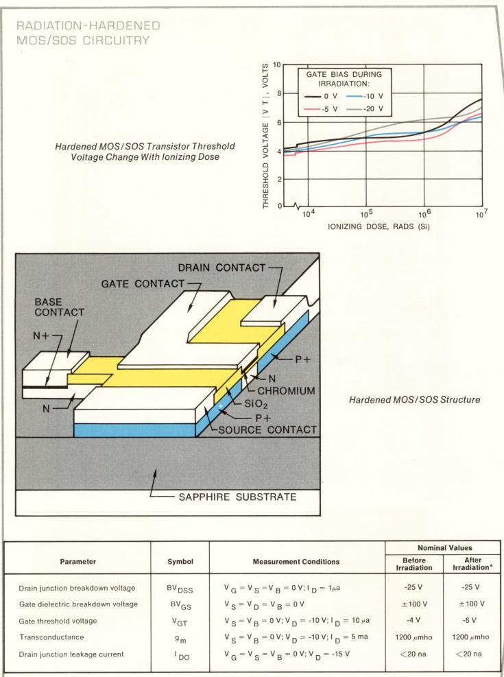
Hardened P-Channel MOS/SOS Transistor Performance Characteristics \*2 x 10 <sup>6</sup> rads (Si), 0 V bias.
