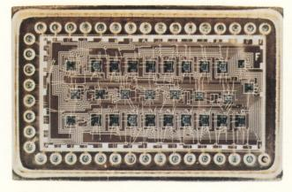
A 28-device hybrid circuit with over 700 "flying lead" (wire) bonds
