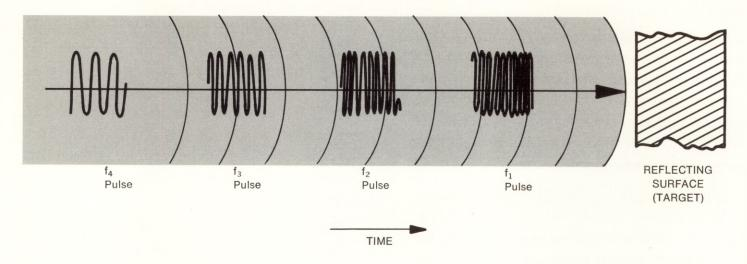
The first pulse sent out and returned (the  $f_1$  pulse) is taken from the antenna to a delay line. After, and only after, being delayed a certain amount by the delay line, the  $f_1$  pulse is permitted to enter the receiver proper.
