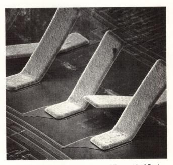
Enlargement of a Scanning Electron Micrograph of Rockwell Gold Beam Leads Applied to MOS Circuitry
