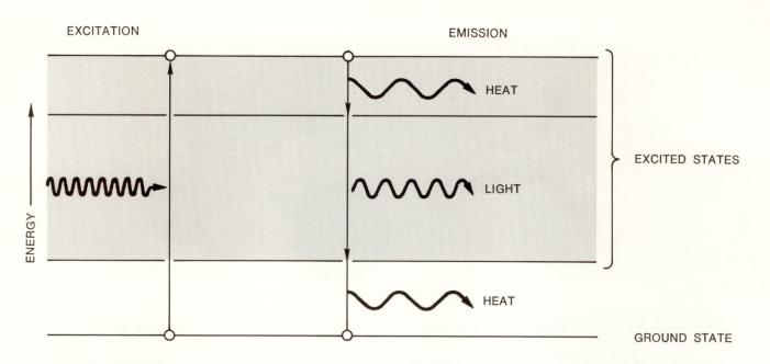
**ENERGY-LEVEL DIAGRAM** of an electron in an isolated atom (for example, in a gas) illustrates the general mechanism of luminescence. An external excitation, which can be a high-energy photon, or light quantum (left), promotes the electron from its ground state to a higher energy state. When the excited electron returns spontaneously to a lower energy
