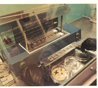
For those which require hermetic seals completed MOS devices are given a helium leak test under high-vacuum conditions.
