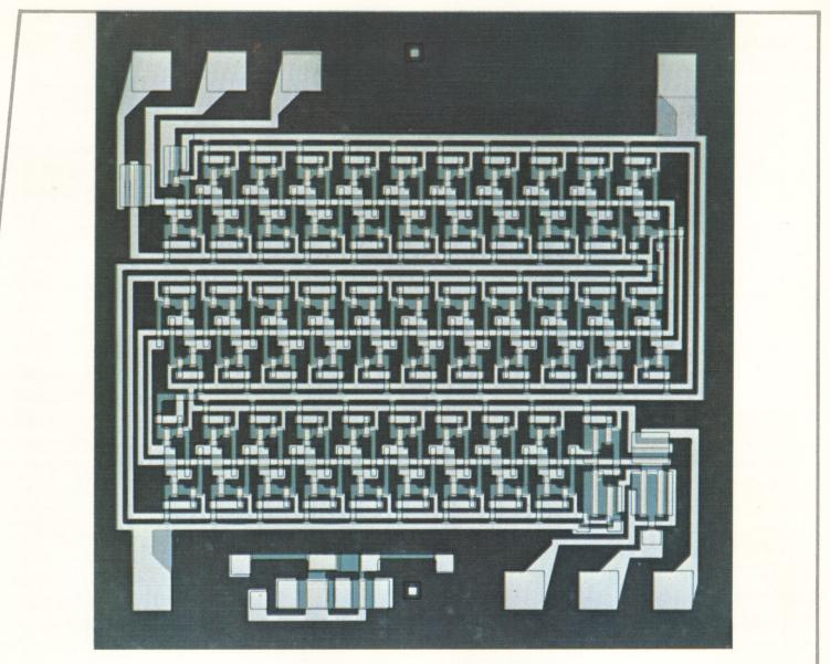
Radiation-Hardened 32-Bit, P-Channel MOS/SOS Dynamic Shift Register
