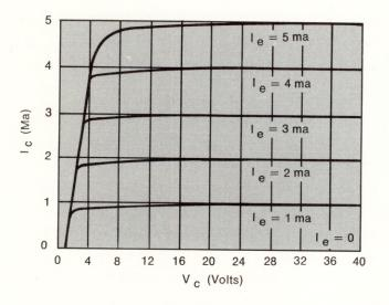
Common-base transistor collector characteristic. Collector current I<sub>e</sub> is plotted vs collector voltage V<sub>e</sub> for various values of emitter current I<sub>e</sub>.
