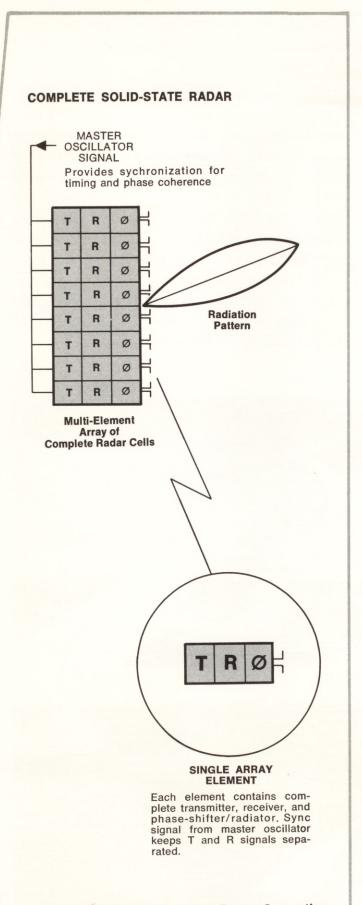
Various Means of Microwave Power Generation and Element Mechanization are employed by different designers. One version has a frequency multiplier on each cell and uses discrete components; another has a tiny bulk solid-state oscillator on each cell. Both versions have a master oscillator for timing and synchronization.
