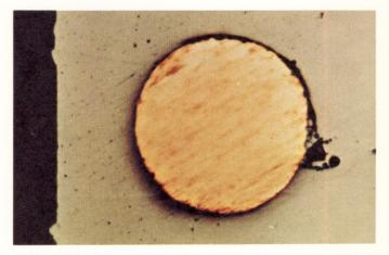
Epitaxially Grown Single-Crystal Ferrite on Magnesium Oxide, with 50-Micron Embedded Gold Wire.
