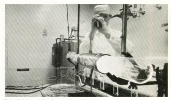
Epitaxial Deposition Temperature Check Wafer temperature is checked by means of an optical pyrometer.
