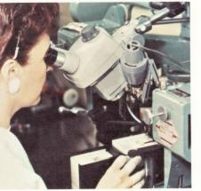
Attachment of Discrete Components Discrete components are resistance-soldered to the ceramic-printed-circuit chips.
