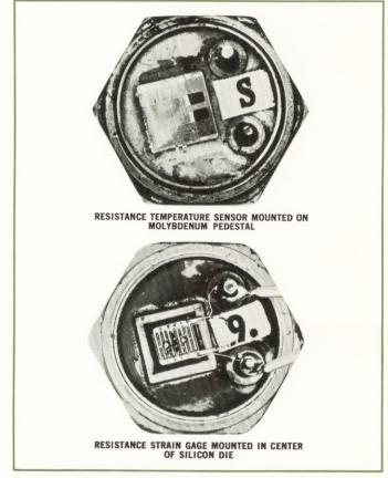
Sensing Devices Mounted on Power Transistor for Accurate Measurement of Temperature and Strain
