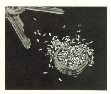
The quantity of semiconductor integrated circuits (IC's) in this wedding ring can form as much as 95% of the electronics for advanced computers.
