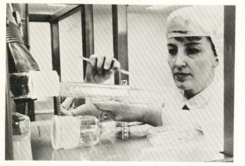
Loading diffusion furnace with "boat-load" of silicon wafers
