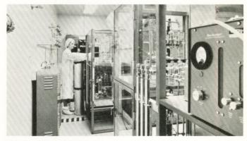
**Diffusion Flow-Rate Regulation** Flow rate of carrier gas and dopant is regulated before processing run.
