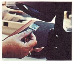
Ultraviolet Inspection of Substrates
