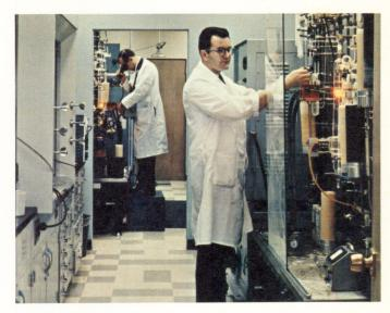
Crystals are grown heteroepitaxially by the chemical vapordeposition process in this laboratory, which is a part of the Research Center, North American Aviation /Autonetics.
