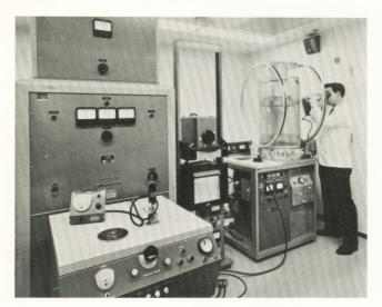
Film Deposition Film deposition is done in precisely controlled high-vacuum evaporators.
