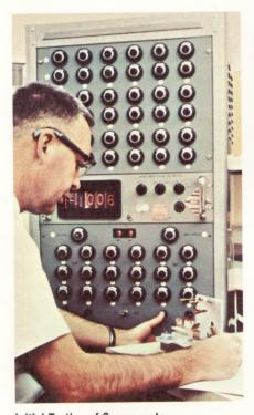
Initial Testing of Components Resistance and capacitance of individual thin-film "components" are measured by a semiautomatic testing machine.
