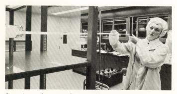
Inserting a thermocouple to run furnace temperature profile
