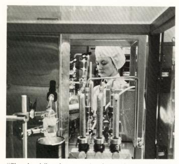
"Glass jungle"-valves, metering devices, heating elementsfor mixing and distributing furnace carrier and dopant gases
