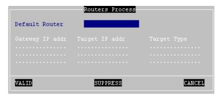
**Default Router**: to specify a default router enter its IP address. If a default router is not required, leave this field blank. If 'Default Router' is enabled in the AX3000 Interface box (see Figure 1.1), this parameter is automatically supplied by DHCP and cannot be accessed.
