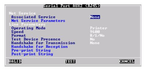
The **[TEST]** button allows communication between the AX3000 auxiliary port and the device to be tested. Whatever the auxiliary port status (TCP/IP connection established or not), when this button is 'pressed', data is sent from the AX3000 port to the device.
