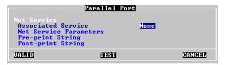
The **[TEST]** button allows communication between the AX3000 auxiliary port and the parallel device to be tested. Whatever the auxiliary port status (TCP/IP connection established or not), when this button is 'pressed', data is sent from the AX3000 port to the device.
