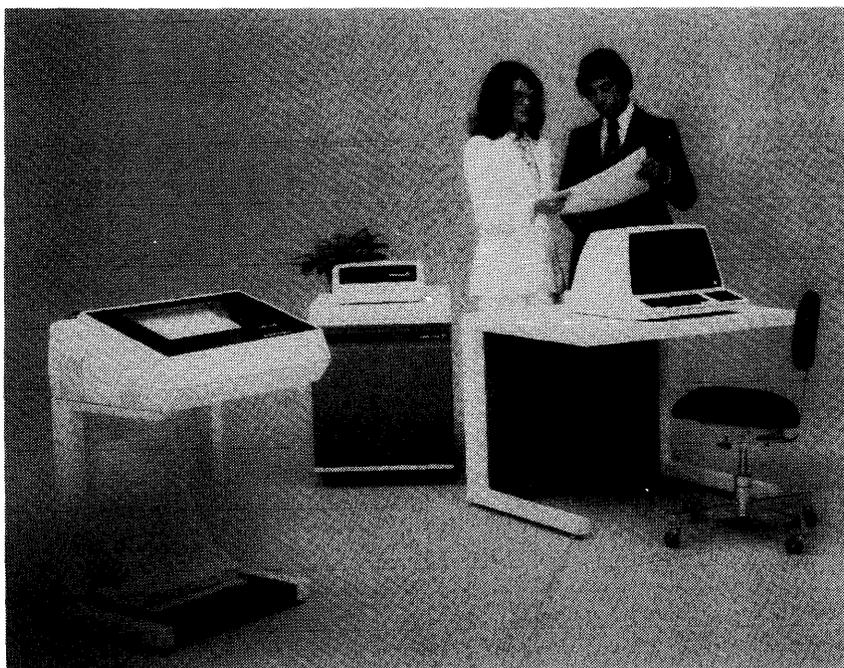
The basic System 200, the entry-level member of the Basic Four line, consists of a CPU with 32K bytes of memory, one 10-megabyte disk unit, one video display terminal, a 120-cps printer, and a 2.5-megabyte magnetic tape cartridge unit. The purchase price for this configuration is \$29,000. A System 200 can be expanded to include up to 40K bytes of memory, 20 megabytes of disk storage, and two VDT's.
