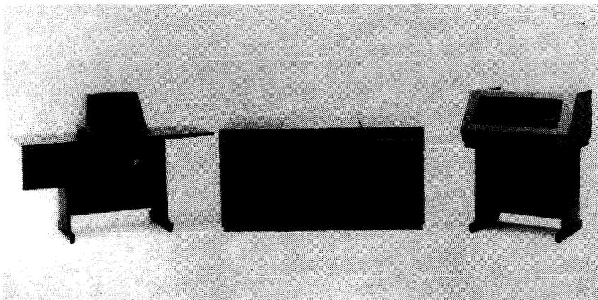
The Basic Four System 610 supports from 64K to 256K bytes of main memory, from 35 to 300 million bytes of disk storage, and up to 16 video data terminals. A basic system with 64K bytes of memory, 35 million bytes of disk storage, one VDT, and a 150-lpm printer sells for \$51,400.
