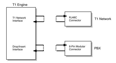
Figure B-2. Network Loopback Mode
