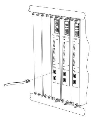
Figure 2-6. Connecting a T1 Network Interface
