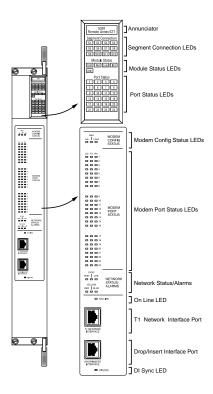
Figure 4-1. Remote Annex 5391/CT1 Front Panel Alarms and LEDs
