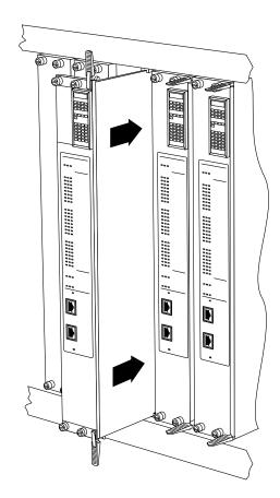
Figure 2-3. Inserting the Module
