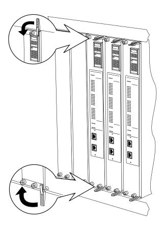
Figure 2-4. Seating Module Connectors
