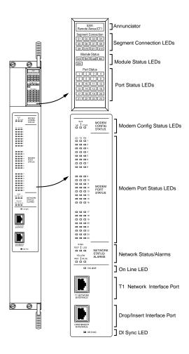
Figure 2-5. Module LED Display
