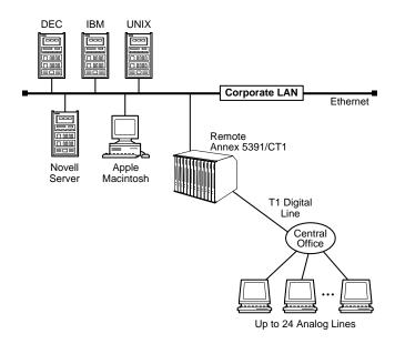
Figure 1-2. The Remote Annex 5391/CT1 as a Remote Access Server
