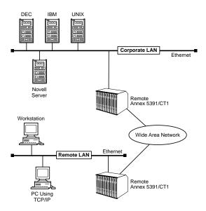
Figure 1-3. The Remote Annex 5391/CT1 as a Dial-up Router
