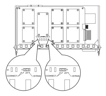
Figure B-1. Network Bypass Jumper Location
