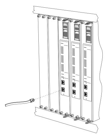
Figure 2-7. Connecting a Drop/Insert Interface
