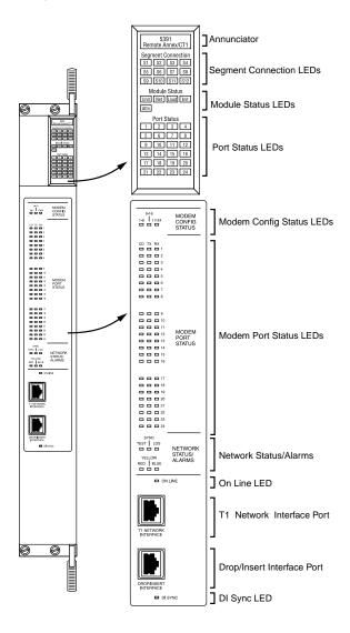
Figure 1-4. Remote Annex 5391/CT1 Front Panel
