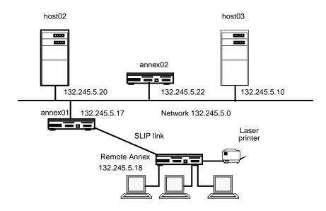
Figure A-13. Connecting a Remote Annex
