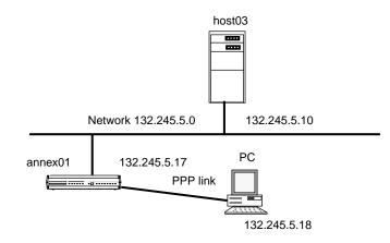
Figure A-9. Connecting a Single Host Using PPP with Fixed Addresses
