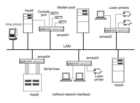
Figure A-3. Connecting Devices to a Remote Annex
