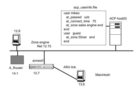
Figure A-28. Connecting a Macintosh Using ARA
