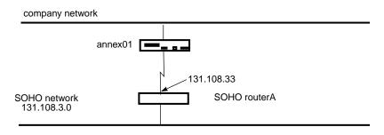
Figure A-30. Sample Configuration for a route Entry in acp\_userinfo
