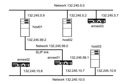
Figure A-10. SLIP Link with Separate Network Address
