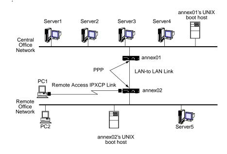
Figure A-25. Sample IPXCP Network Configuration
