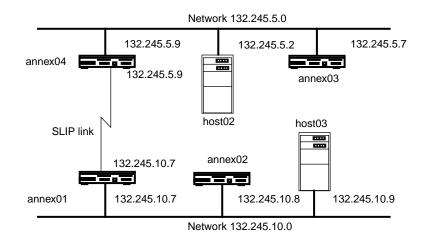
Figure A-11. SLIP Link with Two IP Addresses
