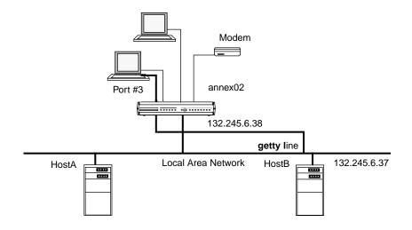
Figure A-2. Host Applications Accessing a Terminal
