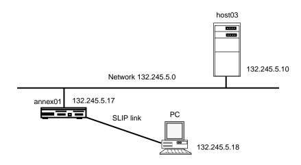
Figure A-12. Connecting a Single Host Using SLIP
