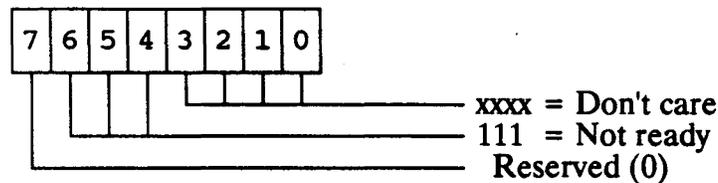
An EISA adapter may report not ready on an attempt to access its EISA Product ID Register (0zC80h) for up to 100 milliseconds before it must return a valid Product ID (see preceding section). This time is measured from the first attempt to read the Product ID Register. The EISA adapter must be ready to accept the configuration information stored in the system's nonvolatile memory as soon as it reports a valid Product ID.
