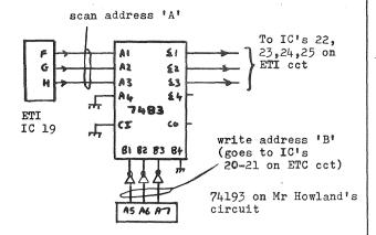
Fig 1 n.b. the links between IC19 and IC1's 22,23, 24,25 should be cut before this cct is added
