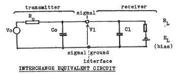
In the above diagram, if Vl is more negative than -3V there is said to be a 'marking' condition, and if Vl is more positive than +3V there is a 'spacing' condition. Voltages in between these are undefined.
