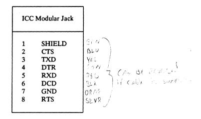
TABLE 7. Connector Pinout: ICC Modular Jack
