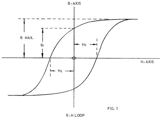
Shown in Figure 1 is a B-H Loop (Hysteresis Loop) with the H axis now called an ampere or current axis, since H is related to current by a constant:
