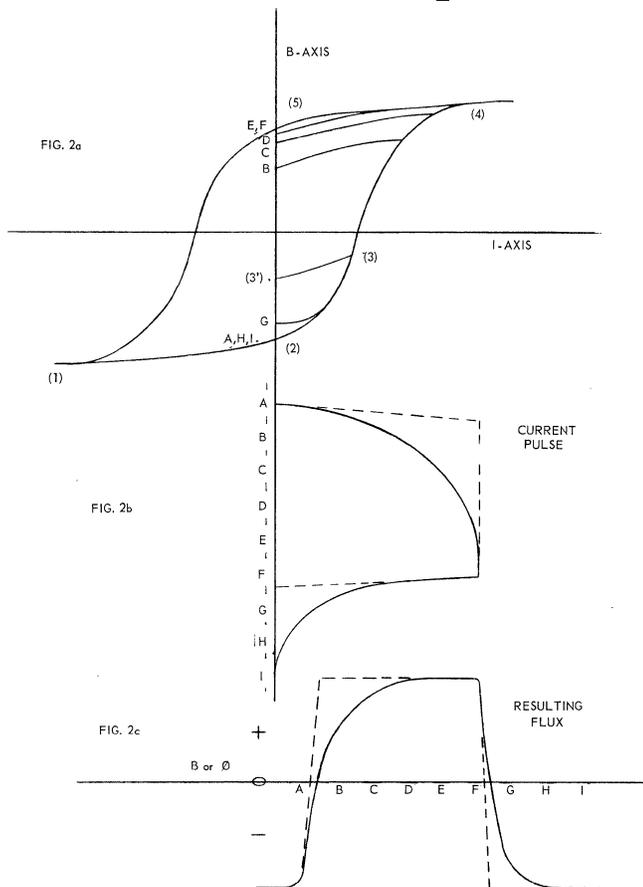
If the B-H Loop shown in Figure 2a represents that of the coating, then the current pulse shown in Figure 2b represents the H field presented to the coating by the gap in the head.
