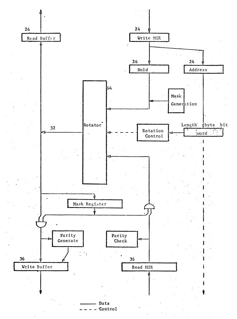
Figure 6. Field Isolation Unit (Memory/Requestor Interface)
