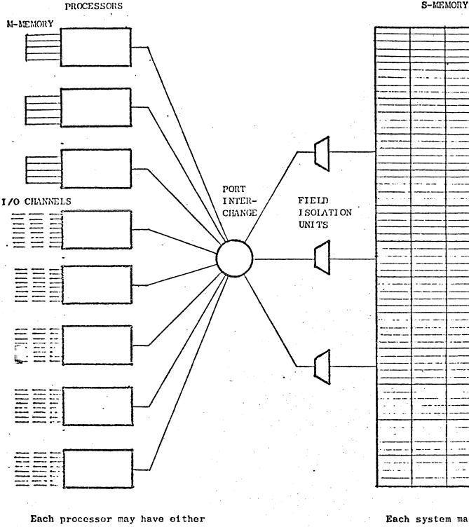
1-8 I/O channels or 1-4 microprogram memory modules of 16,384 bits each.
