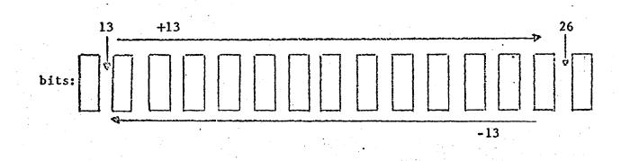
Figure 7. Defined-field addresses labelling between-bit positions.
