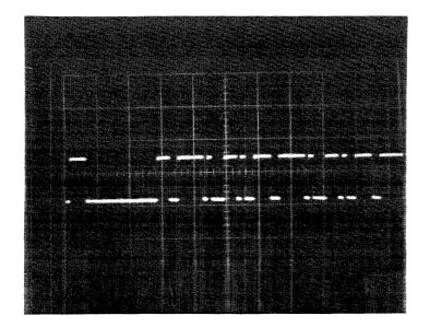
Scope Set Up External Sync on index (TP Cd 3 #HX) Channel 1 – Read Data (TP Cd 3 #NX) A delayed by B Timebase Delay Time Set to .5ms/cm Sweeptime Set to 5us/cm Vertical Set to 2v/cm
