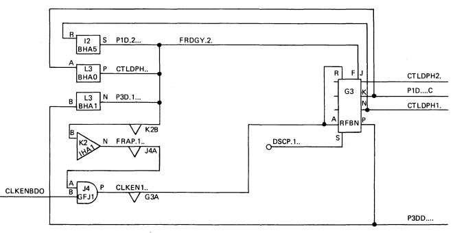
Fig. II-17 BUFFER D CLOCK LOGIC
