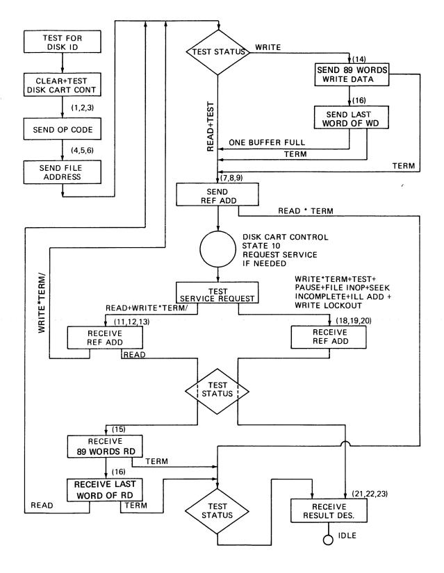
Fig. V-1 PROCESSOR TO DISK CARTRIDGE CONTROL FLOW
