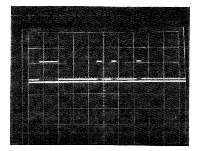
Scope Setup External Sync on index (TP CD 3 #HX) Channel 1 – Write Data (TP CD 3 #YX) A delayed by B Timebase Delay Time Set to 1ms/cm Sweeptime Set to 2us/cm Vertical Set to 2V/cm
