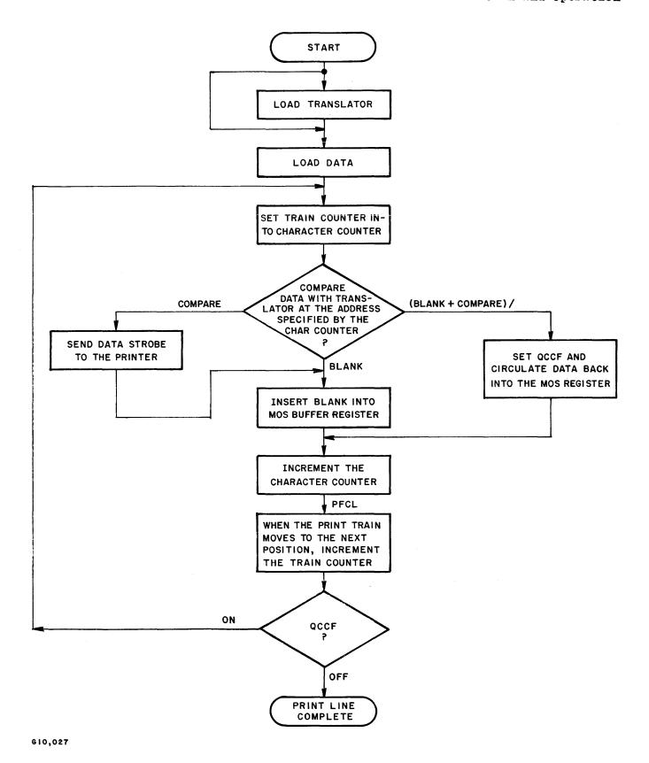
Figure I-5. Soft Translator Flow Diagram
