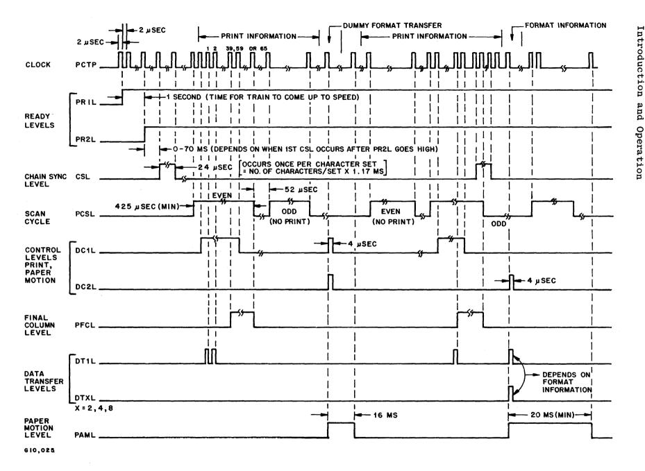
Figure I-2. Timing Diagram for 400 LPM Printer
