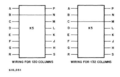
Figure VI-4. Column Length Identifier Wiring
