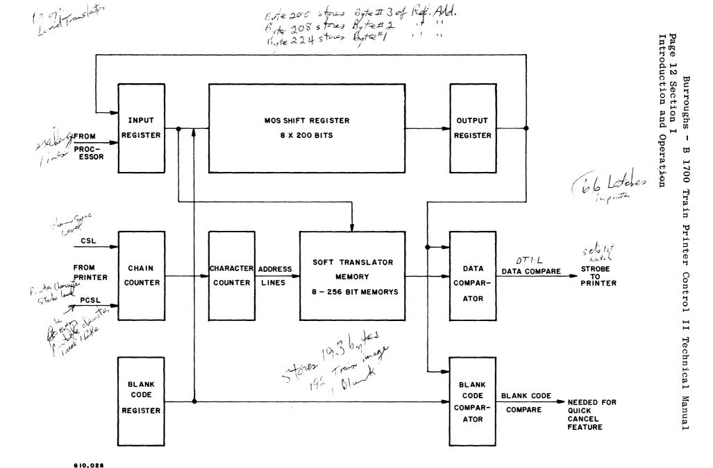
Figure I-4. Soft Translator Basic Block Diagram
