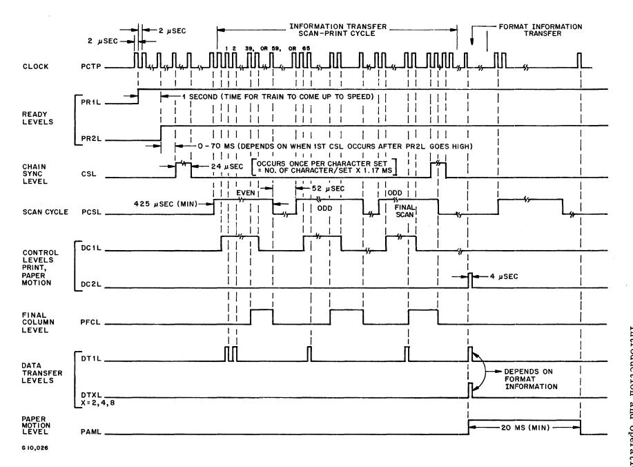
Figure I-3. Timing Diagram for 750 LPM Printer
