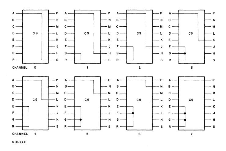
Figure VI-2. Channel Designate Wiring (Channels 0 through 7)
