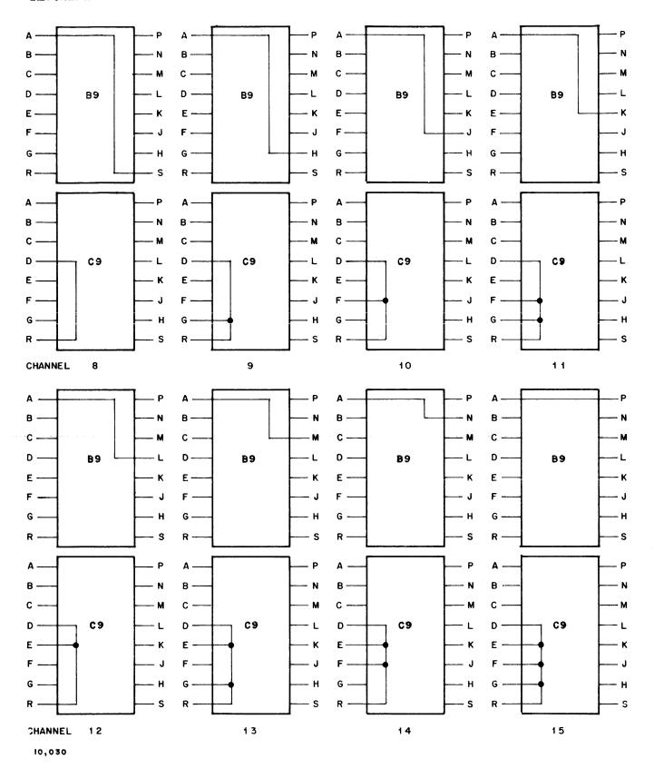
Figure VI-3. Channel Designate Wiring (Channels 8 through 15)
