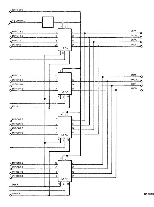
Figure 5-1. Electronic Control Input Register (ECIR)
