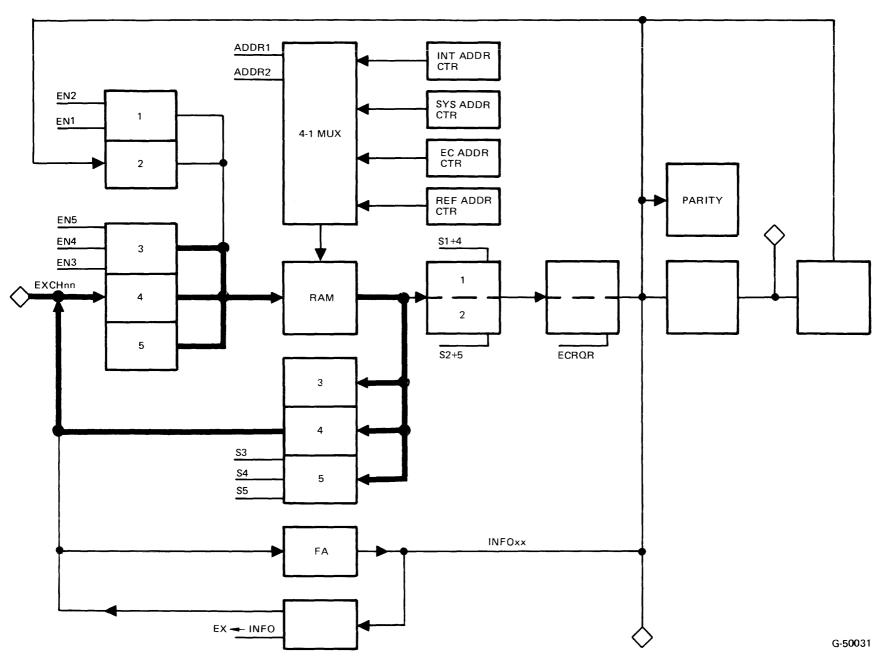
Figure 5-22. Diagnostic RAM Test Data Path
