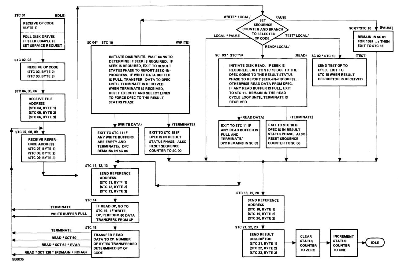
Figure 5-26. Disk Pack Control-II Flow (Detailed)
