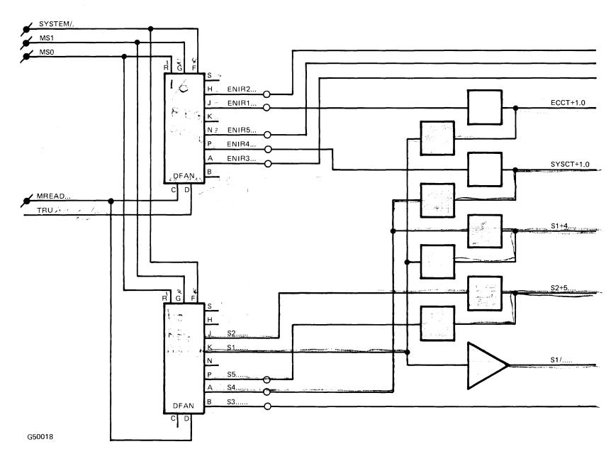
Figure 5-9. Memory Control (Sheet 2 of 2)
