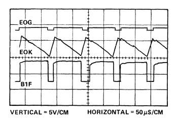
Figure 5-34. VCO Comparator Waveforms (Measured at Comparator EO and B1 on VCO Card)
