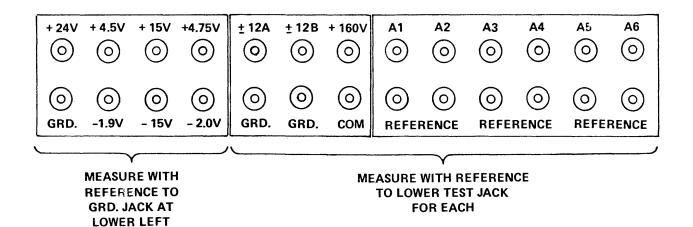
Figure 4-8. Logic Power Supply Test Jacks
