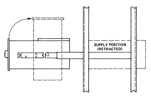
Figure 6-8. Supply Movement Range (Logic Power Supply – 1)
