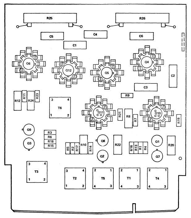
Figure 5-24. Gate Driver Card Component Locations
