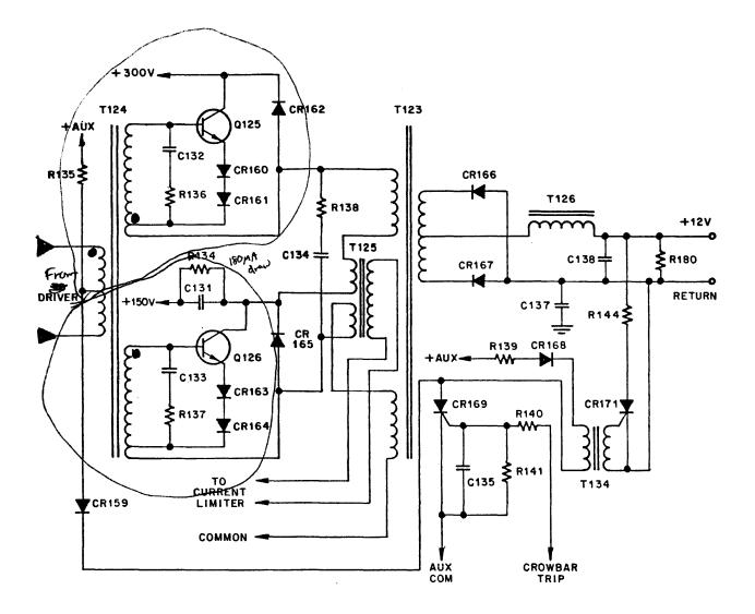
Figure 3-17. +12 Volt Inverter Output Stage
