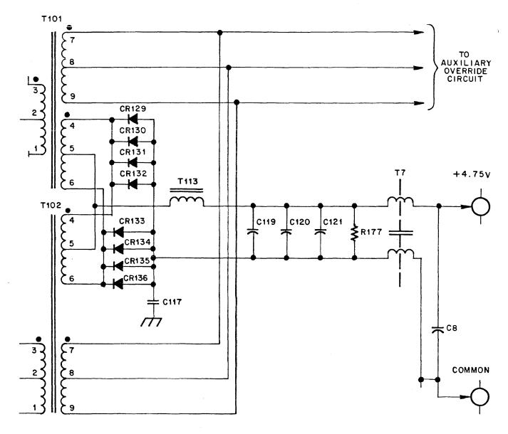
Figure 3-23. +4.75 Volt Rectifier and Filter
