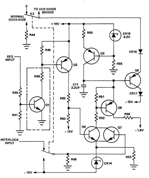
Figure 3-55. Sequencing/Interlock Circuit (Master/Slave Supplies)
