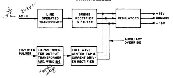
Figure 2-5. ± 15 Volt Auxiliary Supply Block Diagram
