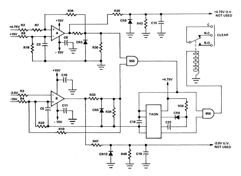
Figure 3-38. Undervoltage Detectors and Clear Circuit
