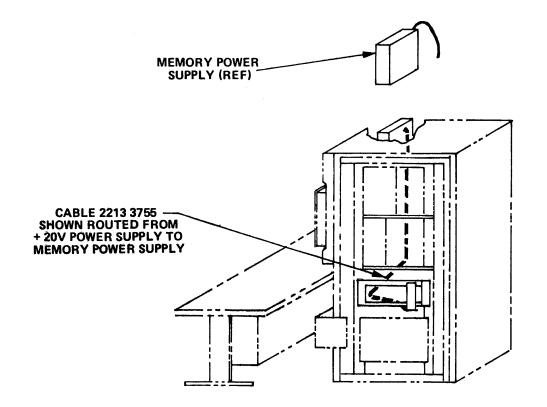
Figure 6-18. + 20 Volt Power Supply AC Cable Routing (B 1710 Series Systems)
