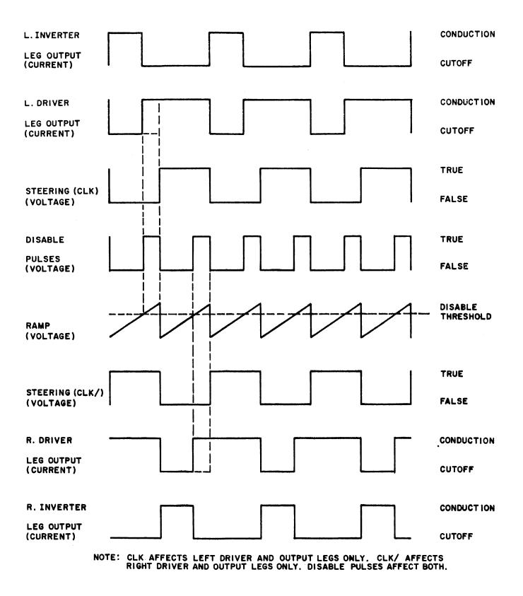
Figure 2-10. Inverter Timing
