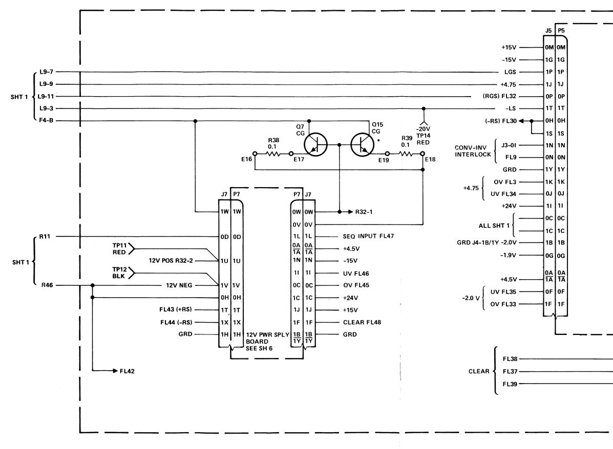
Figure 5-13. Logic Power Supply-1 & -3 Main Schematic (Sheet 4 of 4)
