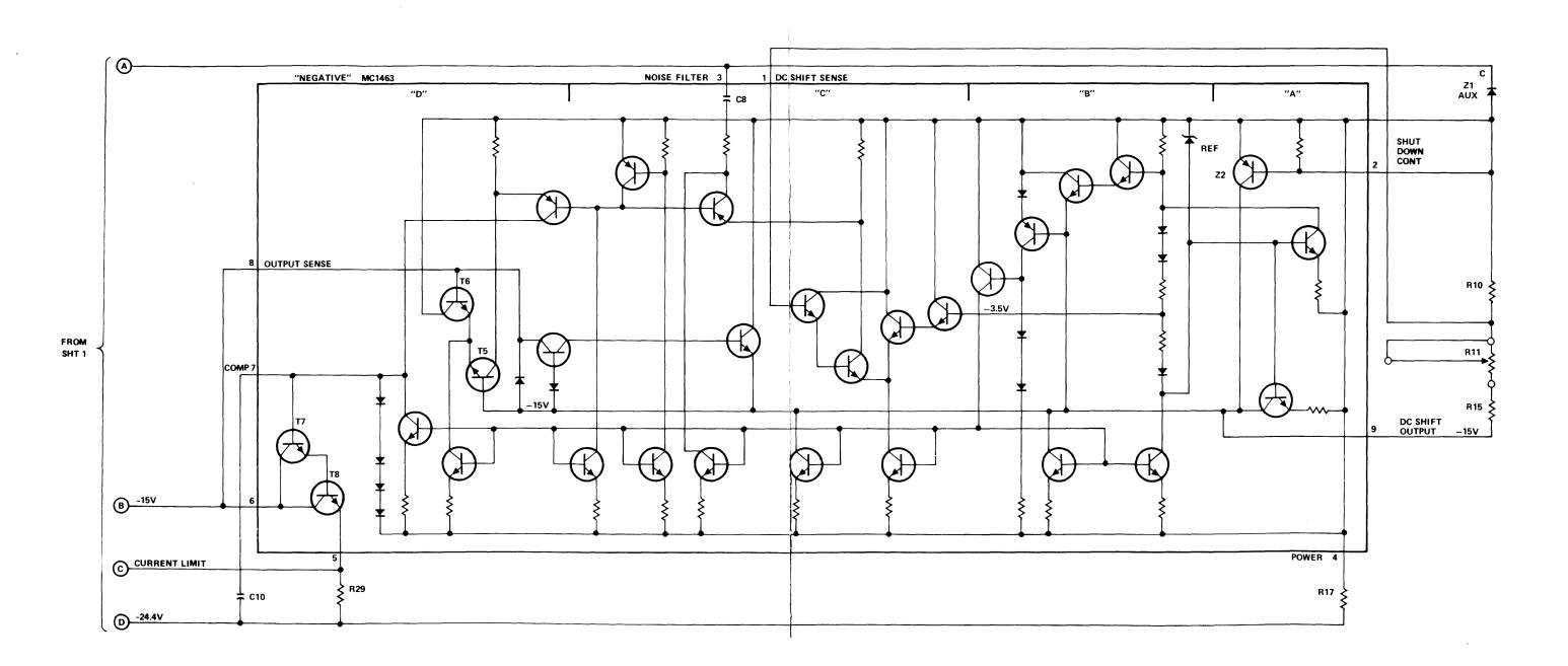
Figure 3-61. +15 Volt Complementary Tracking Supply (Sheet 2 of 2)
