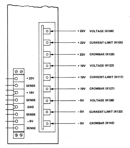
Figure 4-14. Memory Power Supply Controls (Earlier Version, P/N 2201 4229)
