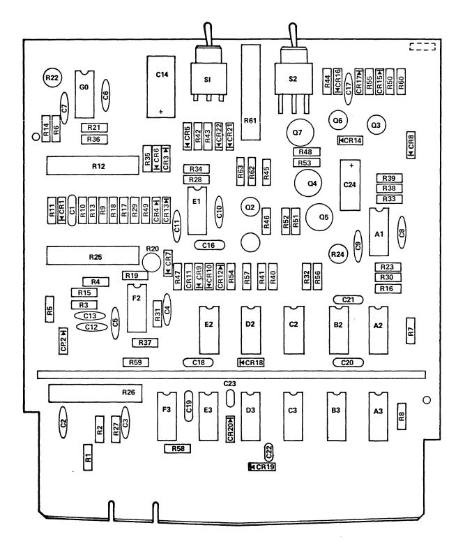
Figure 5-28. VCO Card Component Locations (Logic Power Supply -4)
