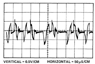
Figure 5-41. Ripple On +160 Volt Output (Measured Across C6 at Output of +160 Volt Supply)
