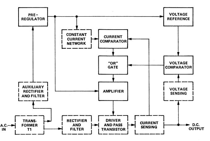
Figure 3-68. IC Regulator Block Diagram (Showing Relationship to External Supply Sections)
