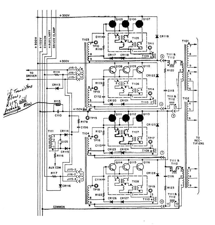
Figure 3-22. +4.75 Volt Inverter Output (Less Rectifiers and Filter)
