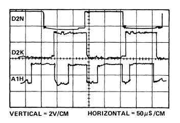
Figure 5-36. VCO Output Waveforms (Measured at Outputs of Flip-Flop D2 and Multivibrator A1 on VCO Card)
