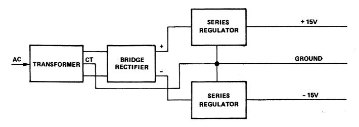
Figure 2-18. ±15 Volt Section of Control Supply
