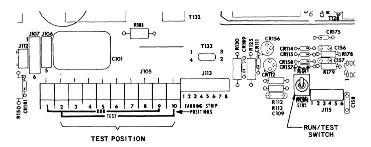
Figure 5-4. RUN/TEST Mode Selection
