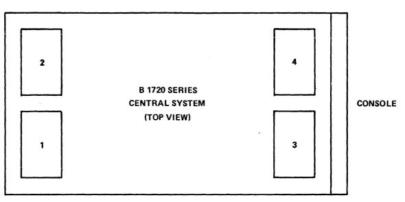
Figure 6-11. Memory Supply Locations in B 1720 Series Systems
