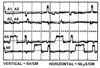
Figure 5-37. VCO Card Output Waveforms (Measured from Pins OK, OH, OD and OG to Ground on VCO Card)
