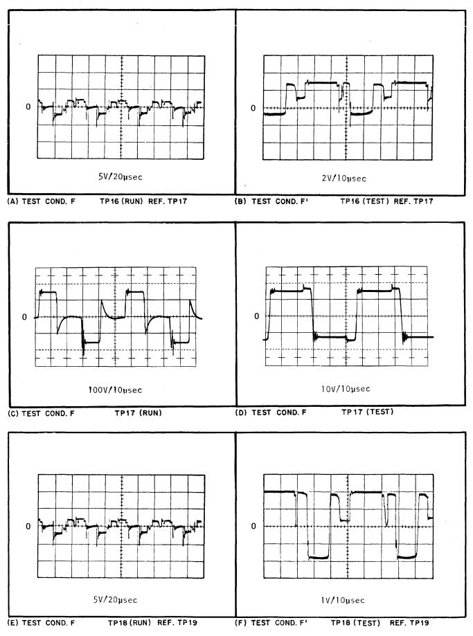
Figure 5-10. Power Board Voltage and Waveform References (Sheet 4 of 13)
