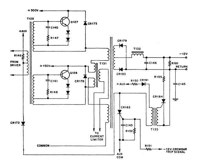
Figure 3-34. -12 Volt Inverter Output
