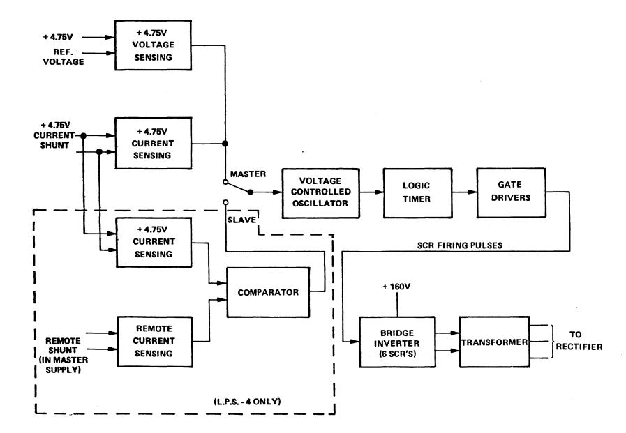
Figure 2-15. Inverter Block Diagram
