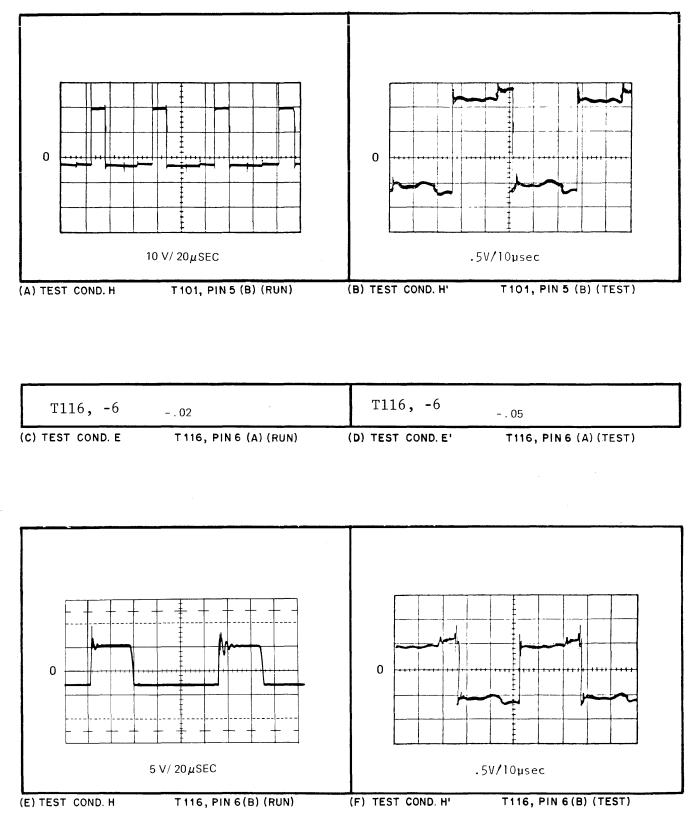
Figure 5-10. Power Board Voltage and Waveform References (Sheet 12 of 13)
