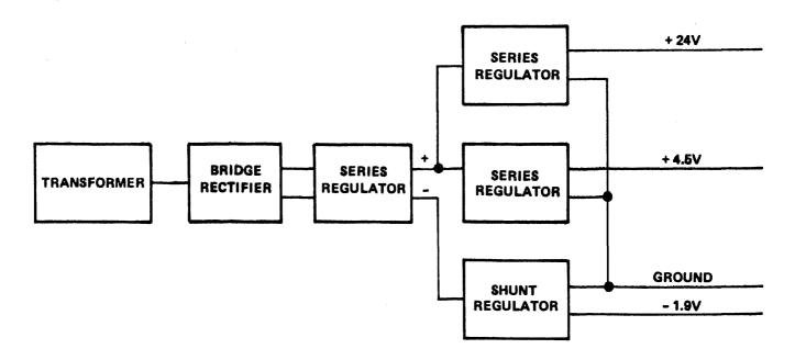
Figure 2-19. +24V, +4.5V and -1.9V Section of Control Supply
