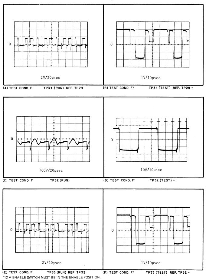
Figure 5-10. Power Board Voltage and Waveform References (Sheet 9 of 13)
