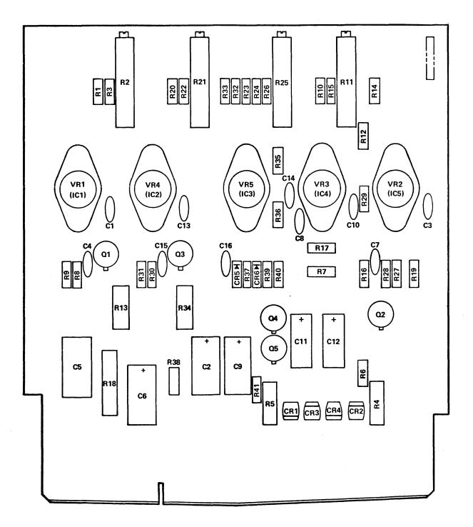
Figure 5-23. Control Supply Card Component Locations
