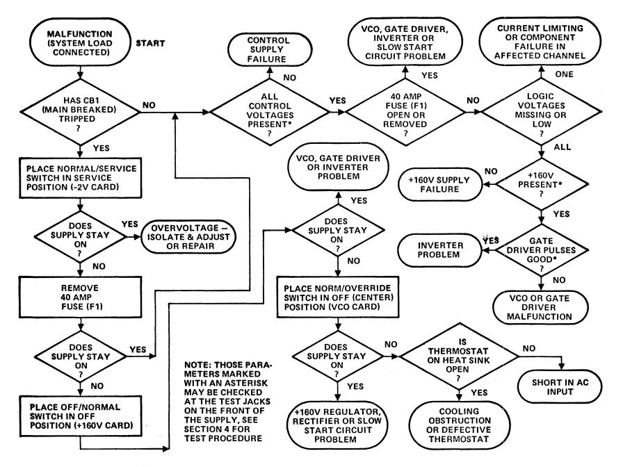
Figure 5-12. Logic Power Supply - 1 Troubleshooting Flow
