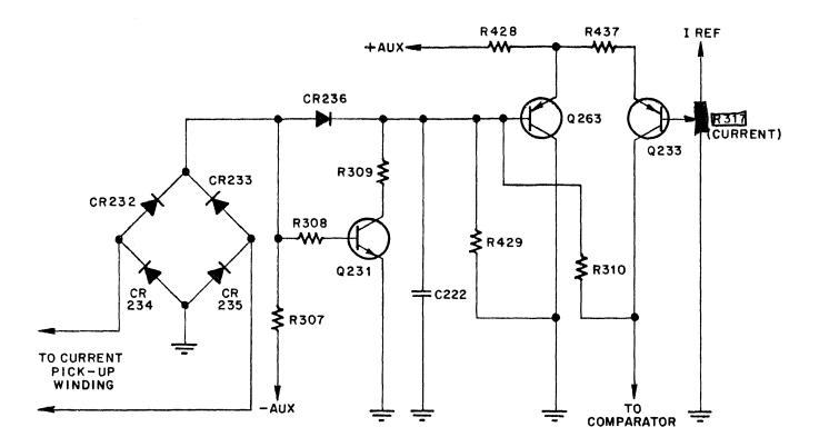
Figure 3-19. +4.75 Volt Current Limiter
