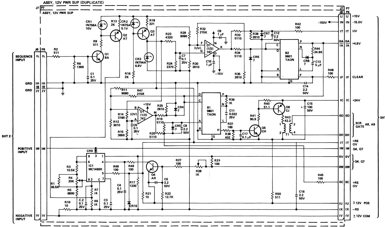
Figure 5-21. Logic Power Supply-1, -3, & -4, 12 Volt Regulator Card Schematic
