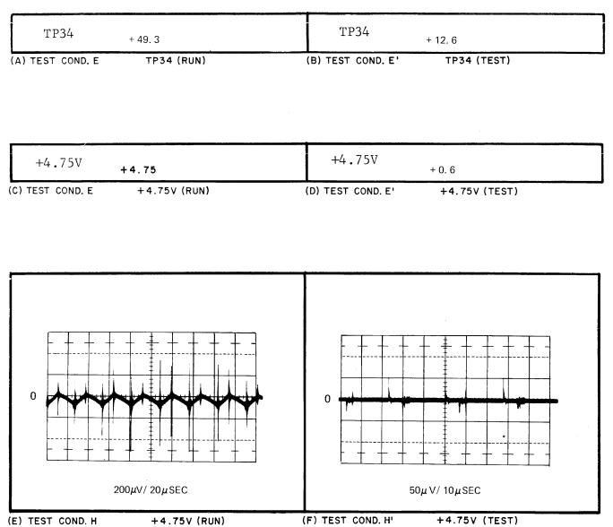
Figure 5-10. Power Board Voltage and Waveform References (Sheet 10 of 13)
