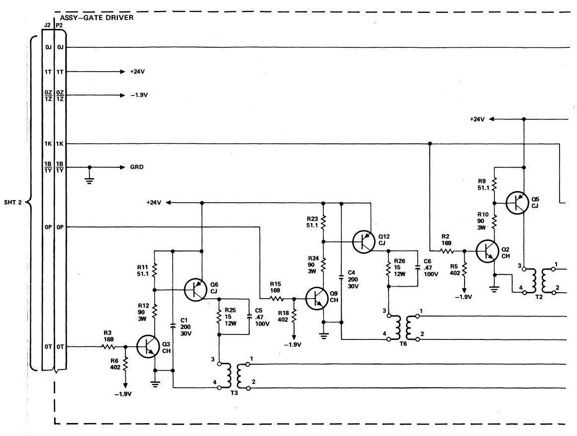
Figure 5-20 Logic Power Supply -1, -3, -4 Gate Driver Card Schematic
