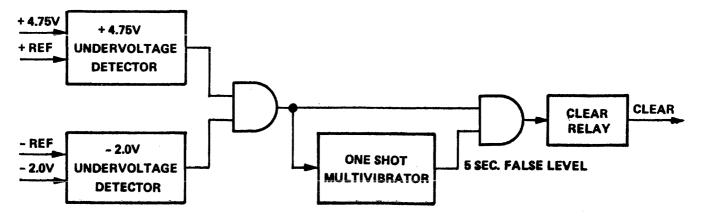
Figure 2-13. Undervoltage Detectors and Clear Signal Generator
