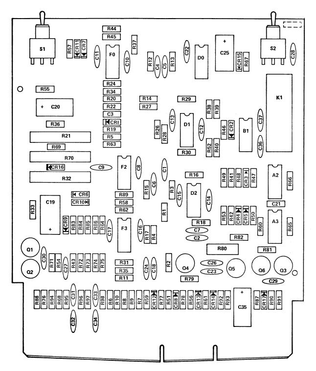
Figure 5-26. -2 Volt Shunt Regulator Component Locations (Logic Power Supply -4)
