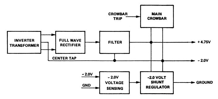
Figure 2-16. High Current Supply Block Diagram
