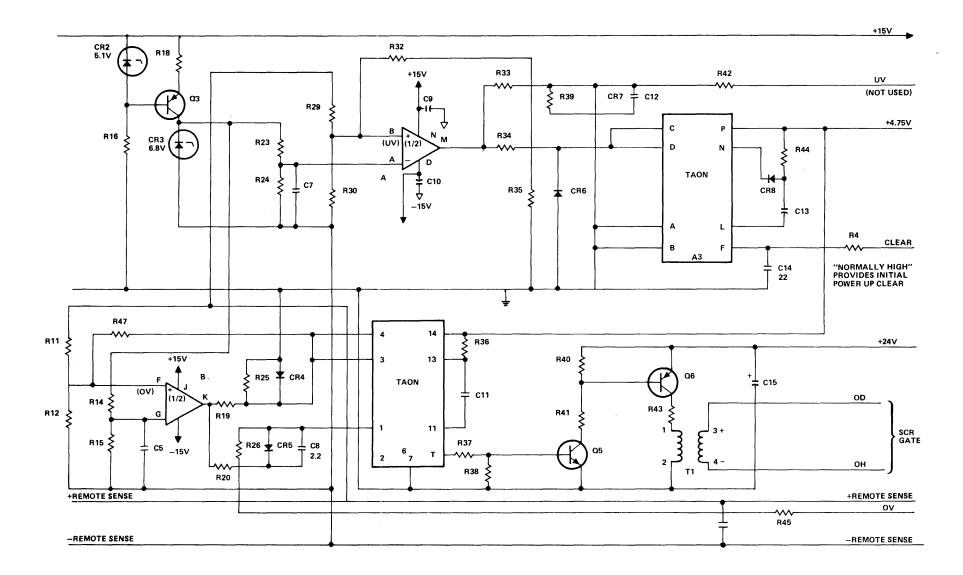
c. DC Level Shift The DC Level Shift circuit amplifies the reference voltage generated by the bias circuit to a level which can be used as the final or output reference voltage for the output regulator.
