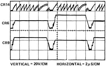
Figure 5-32. 160 Volt Regulator Card Internal Waveforms (Measured From Cathodes of CR6, CR9 & CR14 to +160V)
