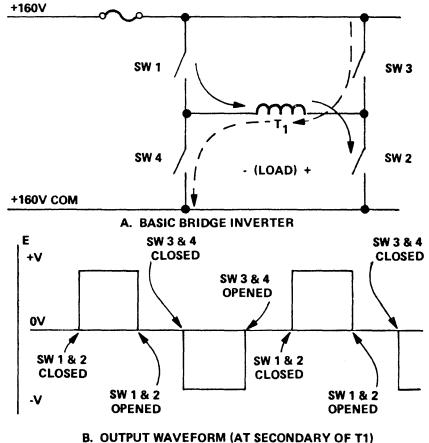
Figure 3-41. Bridge Inverter Operation
