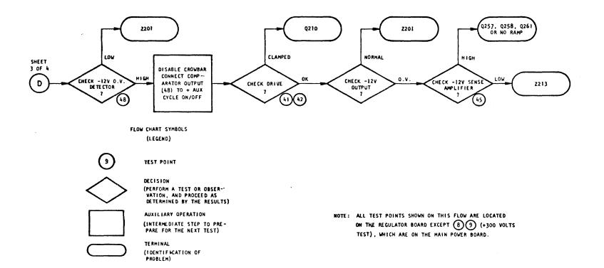
Figure 5-1. Logic Power Supply Main Troubleshooting Flow (Sheet 4 of 4)
