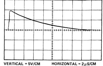
Figure 5-33. +160 Volt Regulator Gate Driver Pulse (Measured at Pins OP/OR and OP/OK of Connector U3)
