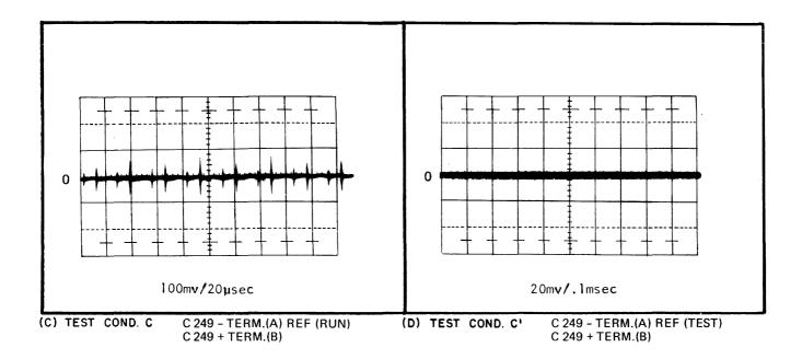
Figure 5-9. Regulator Board Voltage and Waveform References (Sheet 16 of 17)
