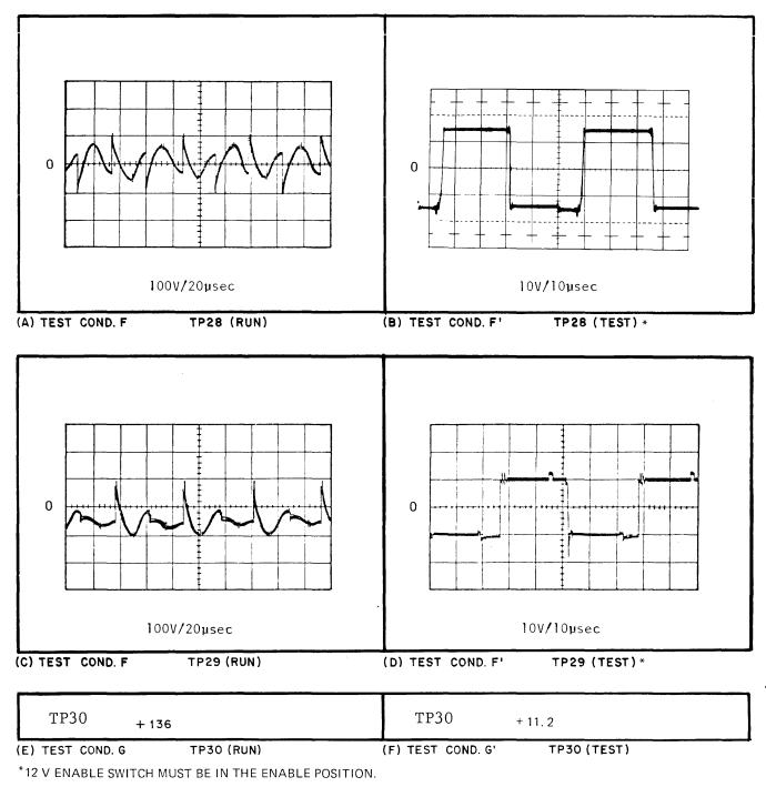
Figure 5-10. Power Board Voltage and Waveform References (Sheet 8 of 13)
