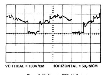
Figure 5-42. Inverter SCR A1 Output (Measured at A1 Test Jacks on Supply Front Panel)
