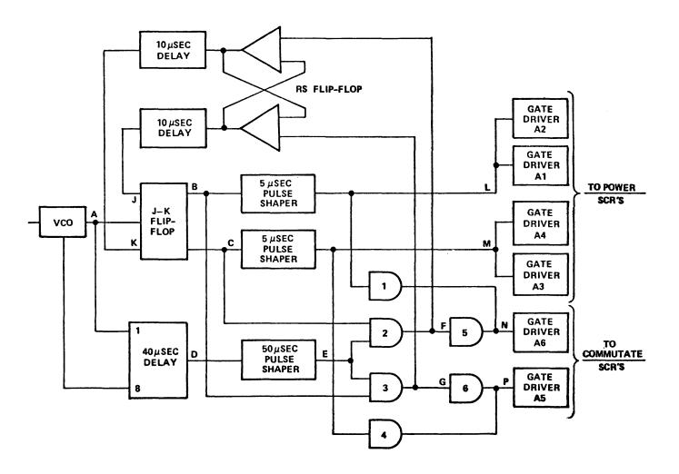
Figure 3-48. Inverter Timing Circuit Block Diagram
