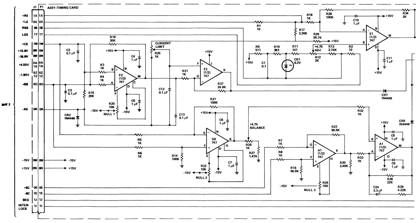
Figure 5-17 Logic Power Supply -4 VCO Card Schematic (Sheet 1 of 2)
