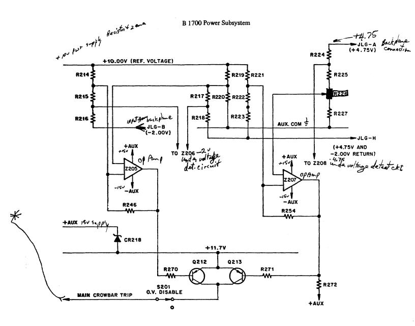
Figure 3-6. +4.75 Volt and -2.0 Volt Overvoltage Detectors
