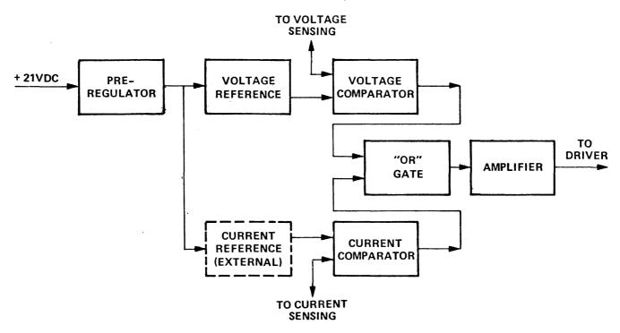
Figure 3-72. Integrated Circuit Regulator Block Diagram
