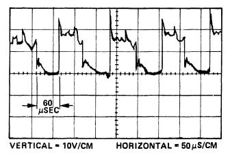
Figure 5-47. High Current Rectifier Output (Measured Across Pins 1 & 4 of Choke L10)
