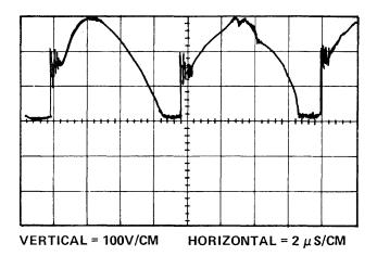
Figure 5-40. Diode/SCR Bridge Rectifier Output (Measured Between Pins 2 and 3 of Choke L1)
