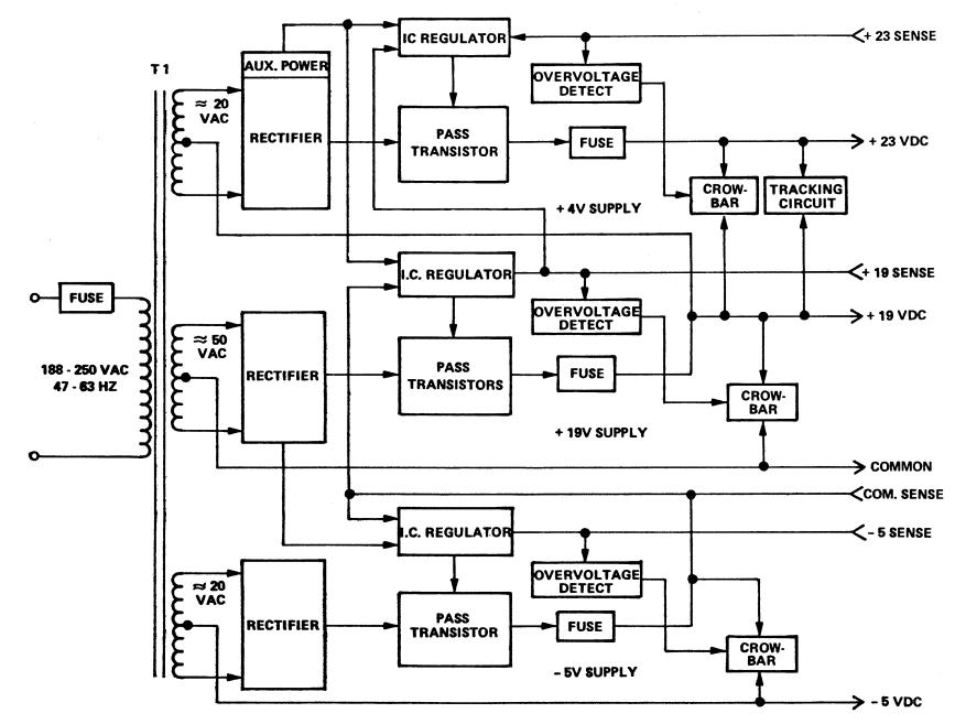
Figure 2-20. Memory Power Supply Block Diagram
