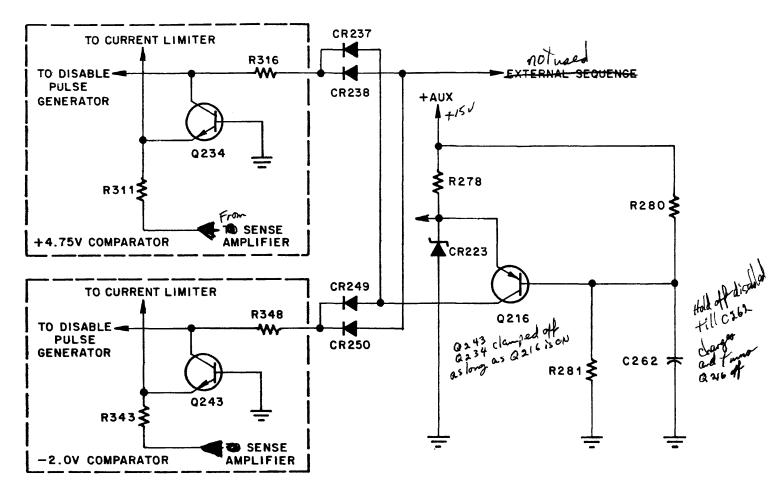
Figure 3-11. +4.75/-2.0 Volt Hold-Off Circuit
