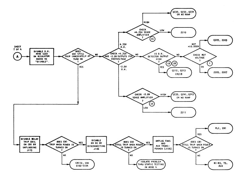
Figure 5-1. Logic Power Supply Main Troubleshooting Flow (Sheet 2 of 4)
