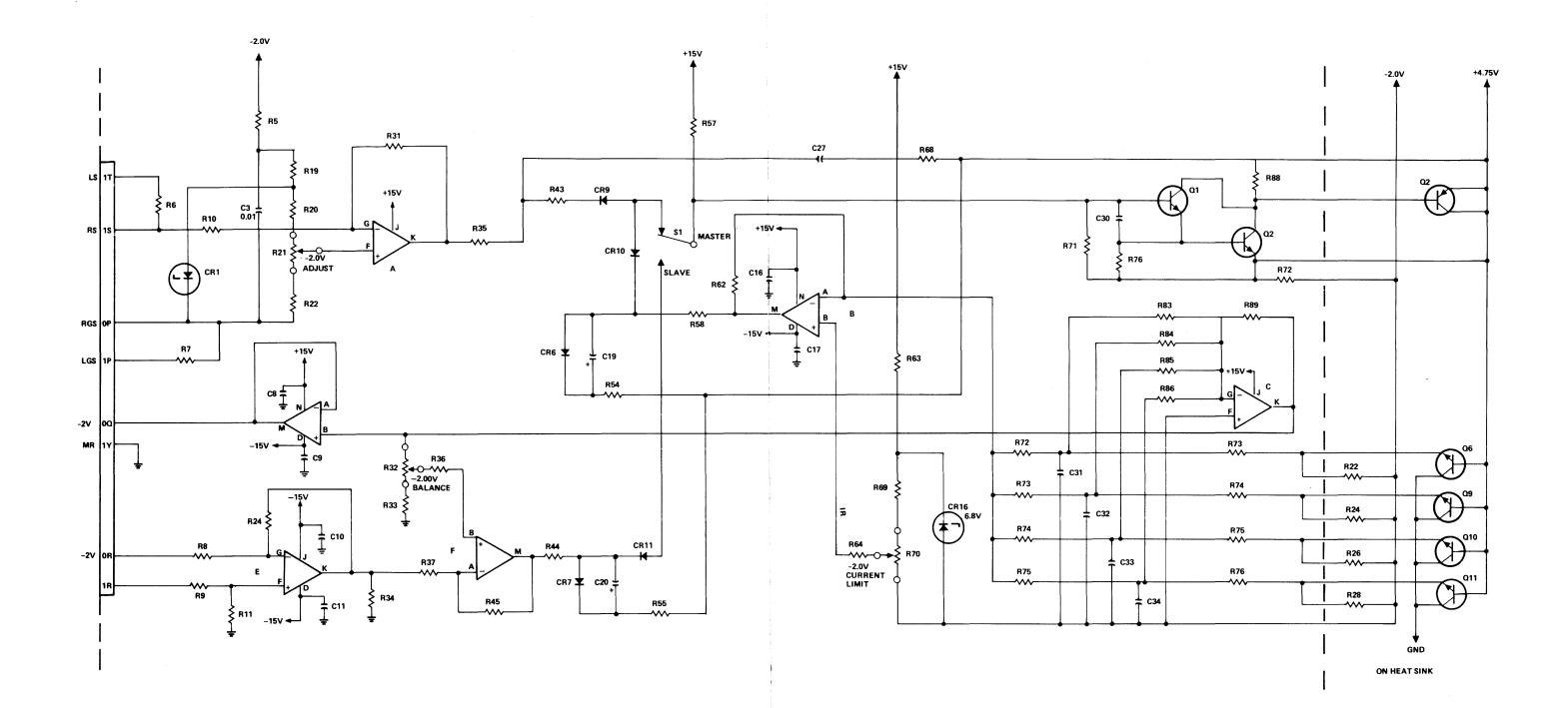
Figure 3-57. -2.0 Volt Shunt Regulator (Master/Slave Version)
