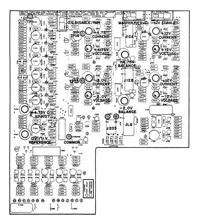
Figure 4-2. Regulator Board Control and Test Point Locations
