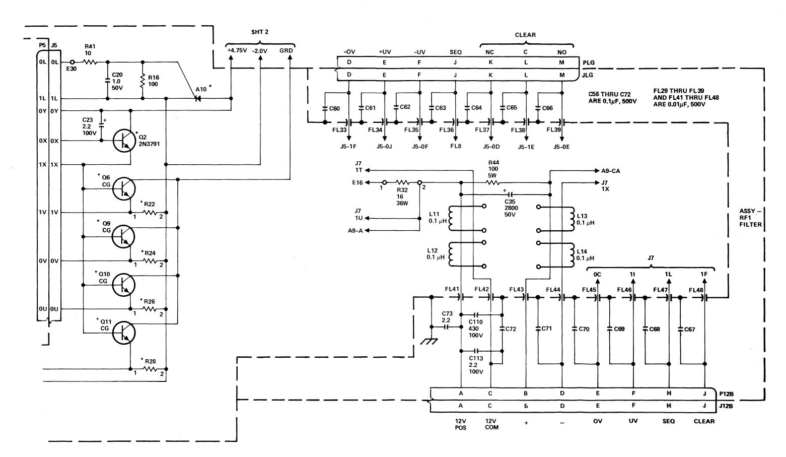
Figure 5-13 Logic Power Supply - 1 & 3 Main Schematic (Sheet 4 of 4 continued)
