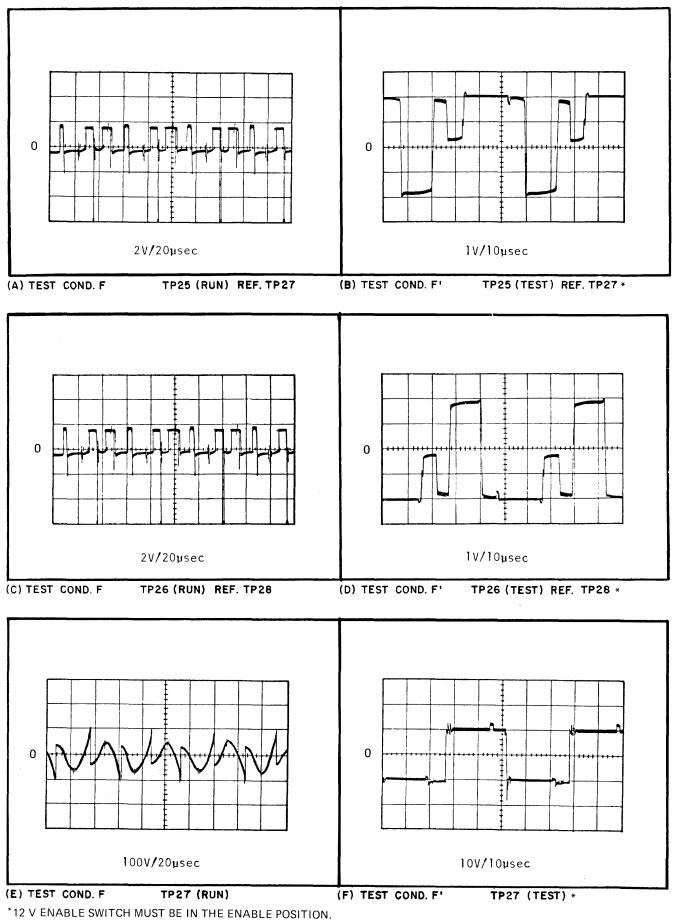
Figure 5-10. Power Board Voltage and Waveform References (Sheet 7 of 13)
