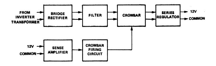
Figure 2-17. 12 Volt Power Supply Block Diagram
