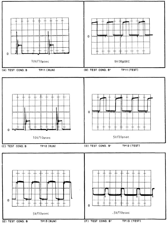
Figure 5-9. Regulator Board Voltage and Waveform References (Sheet 4 of 17)
