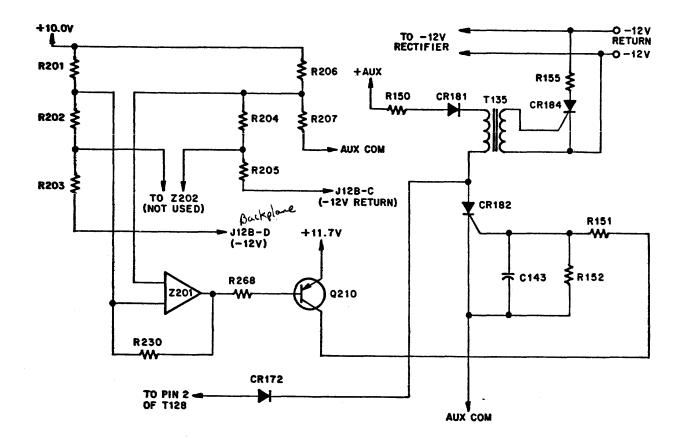
Figure 3-8. -12 Volt Overvoltage Detector and Crowbar
