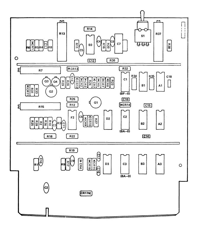
Figure 5-27. VCO Card Component Locations (Logic Power Supply -1 & -3)
