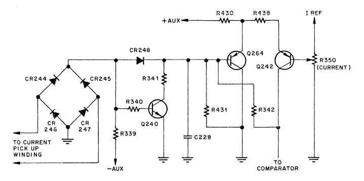
Figure 3-25. -2.00 Volt Current Limiter
