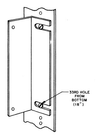
Figure 6-5. Regulator Board Bracket Installation
