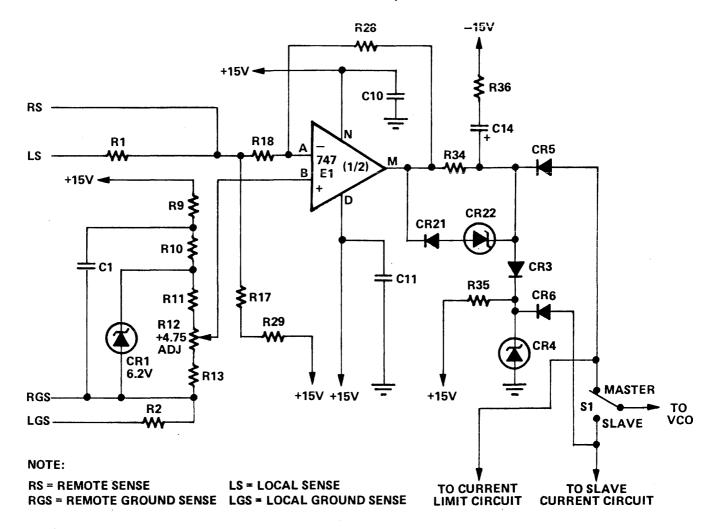
Figure 3-47. +2.75V Comparator (Master/Slave Supplies)
