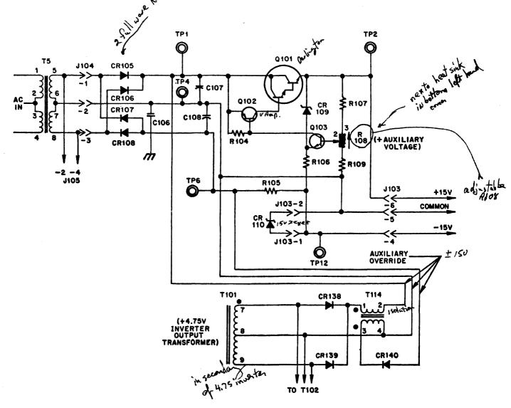
Figure 3-3. ±15 Volt Auxiliary Supply
