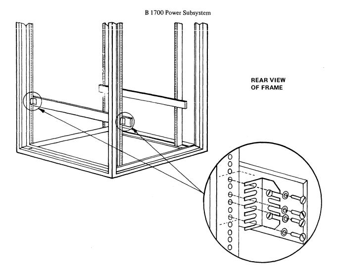
Figure 6-6. Installation of Logic Power Supply - 1 Slides in B 1700 Frame
