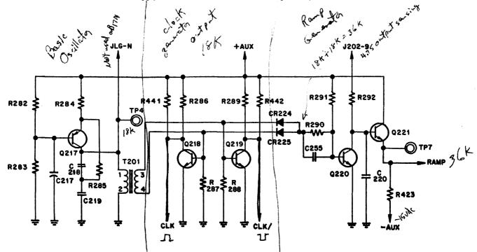
Figure 34. Master Oscillator, Clock and Ramp Generator
