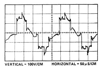
Figure 5-46. Waveform at Primary of Transformer T2 (Measured Across T2 Primary)
