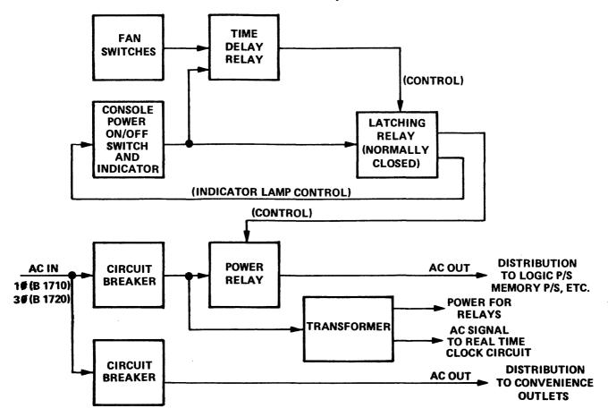
Figure 2-22. System AC Control Block Diagram
