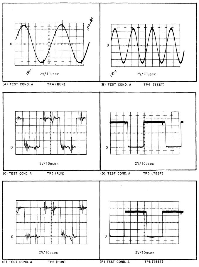
Figure 5-9. Regulator Board Voltage and Waveform References (Sheet 2 of 17)
