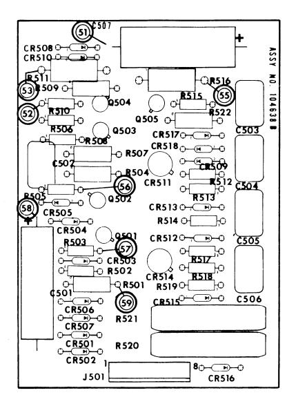
Figure 5-7. Test Point Location on Inrush Control Board (Component Side)
