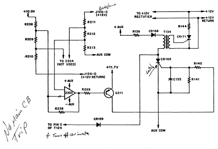
Figure 3-7. +12 Volt Overvoltage Detector and Crowbar
