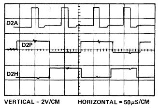
Figure 5-35. VCO Internal Waveforms (Measured at Inputs of Flip-Flop D2 on VCO Card)
