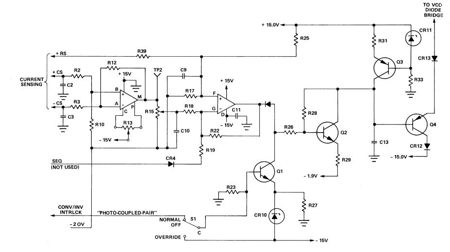
Figure 3-52. +4.75 Volt Current Limiter (Stand Alone Supply)
