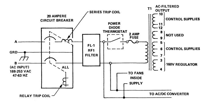
Figure 3-35. Logic Supply AC Control
