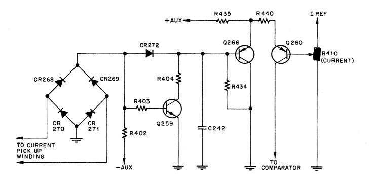
Figure 3-31. -12 Volt Current Limiter
