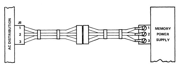
Figure 6-12. Memory Supply AC Connections
