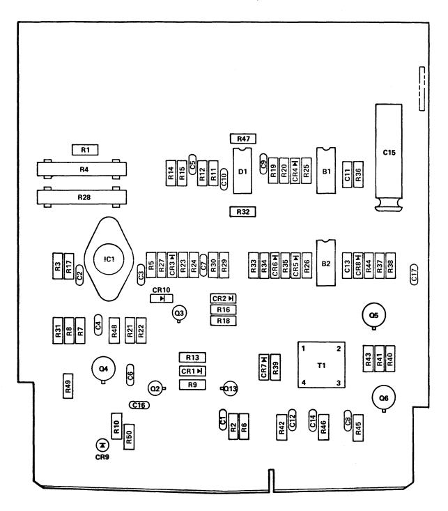
Figure 5-29. 12 Volt Supply Card Component Locations
