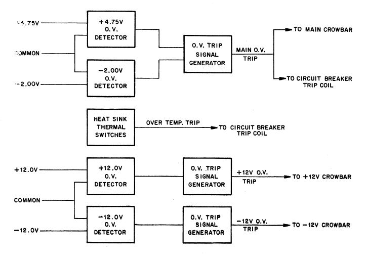
Figure 2-2. Overvoltage Protective Circuit Block Diagram
