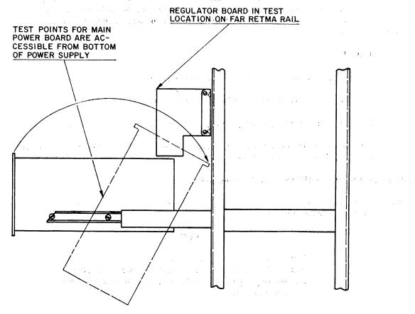
Figure 4-1. Supply in Test Configuration
