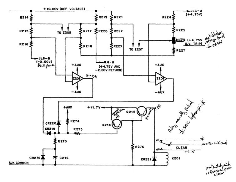
Figure 3-9. +4.75 Volt and -2.00 Volt Undervoltage Detectors and Clear Detector
