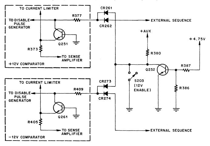
Figure 3-12. 12-Volt Hold-Off Circuit
