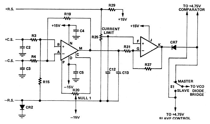
Figure 3-54. +4.75 Volt Current Limiter (Master/Slave Supplies)
