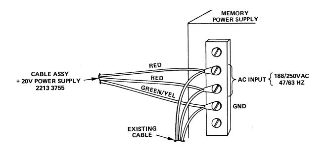
Figure 6-17. + 20 Volt Power Supply AC Wiring
