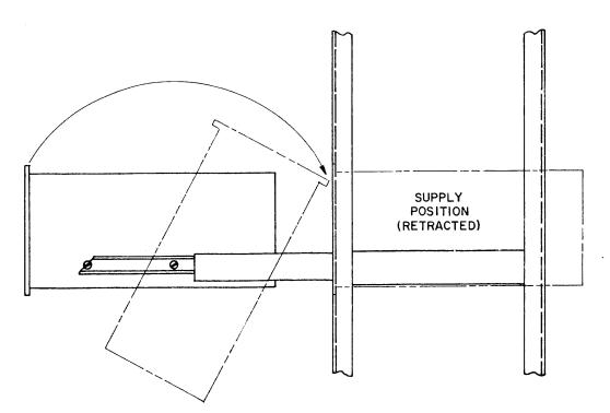
Figure 6-4. Supply Movement Range (Logic Power Supply - 2)
