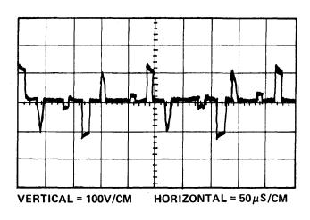
Figure 5-43. Inverter SCR's A5 & A6 Output (Measured at A5 & A6 Test Jacks on Supply Front Panel)
