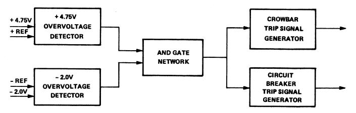
Figure 2-12. Overvoltage Protection Circuit (+4.75V and -2.0V Outputs Only)
