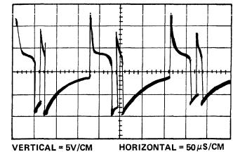
Figure 5-39. Gate Driver Outputs A5 & A6 (Measured Across Secondary of Pulse Transformers T3 and T6 on Gate Driver Card)
