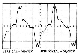
Figure 5-44. Waveform at Commutating Capacitors (Measured Across Capacitors C1 & C2 in Inverter)
