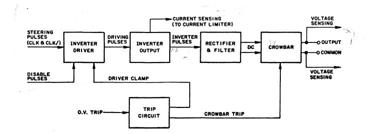
Figure 2-9. Inverter Block Diagram (One Channel Only is Shown)
