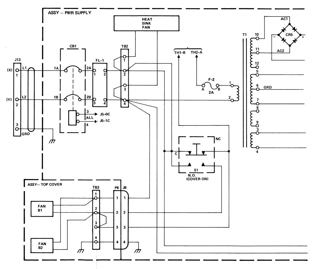
Figure 5-16 Logic Power Supply -4 Main Schematic (Sheet 3 of 4)
