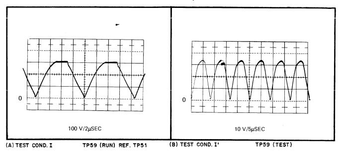
Figure 5-11. Inrush Control Board Voltage and Waveform References (Sheet 3 of 3)
