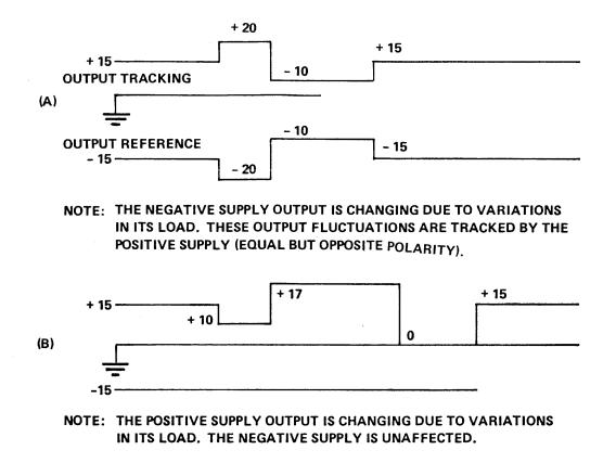
Figure 3-62. ±15 Volt Supply Tracking
