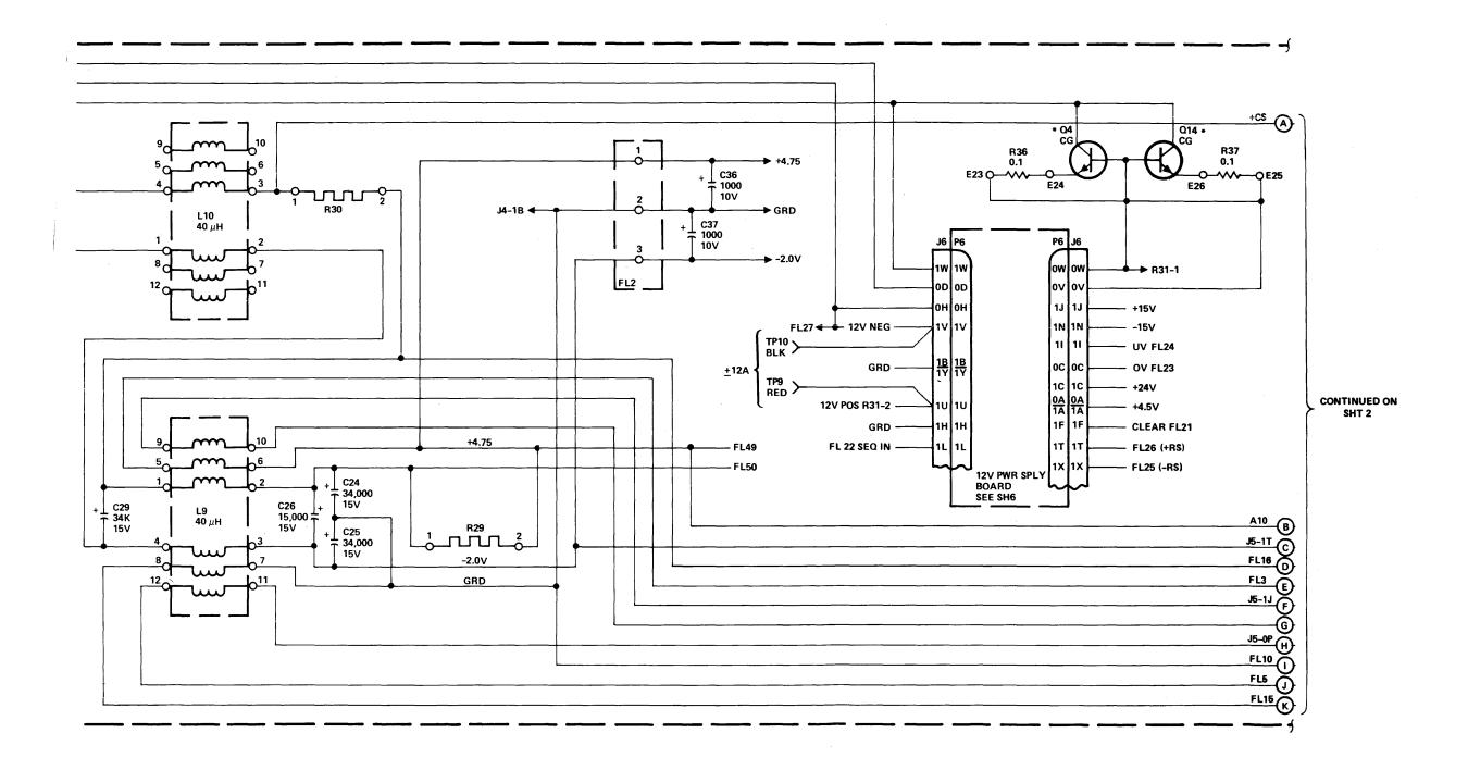
Figure 5-13 Logic Power Supply - 1 & 3 Main Schematic
