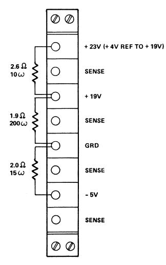
Figure 4-15. Memory Supply Dummy Load Connections
