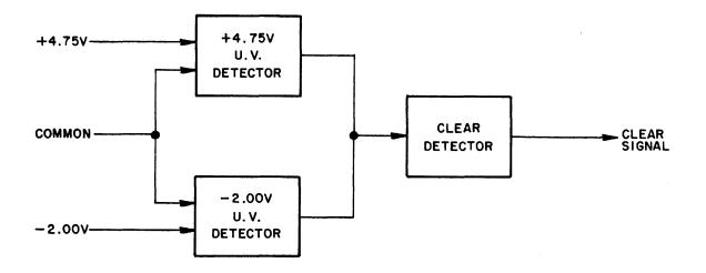
Figure 2-3. Clear Detector Block Diagram
