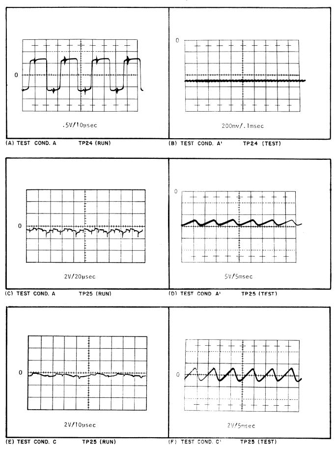
Figure 5-9. Regulator Board Voltage and Waveform References (Sheet 8 of 17)
