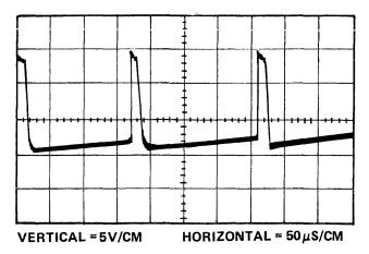
Figure 5-38. Gate Driver Outputs A1-A4 (Measured Across Secondary of Pulse Transformers T1, T2, T4 and T5 on Gate Driver Card)
