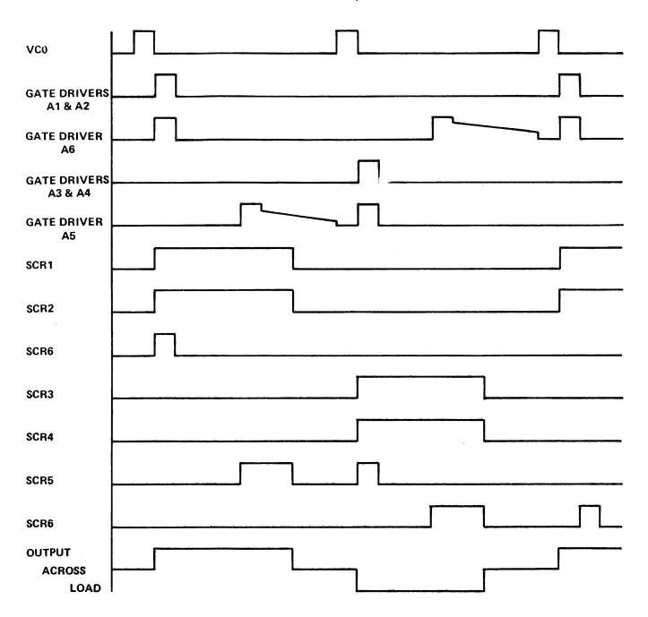
Figure 3-49. Inverter Timing
