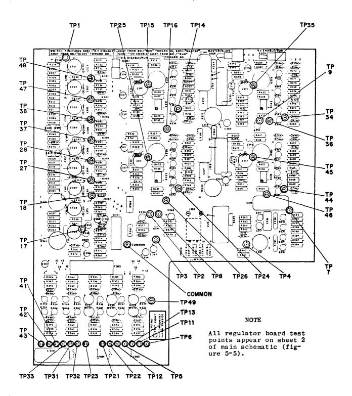
Figure 5-6. Test Point Locations on Regulator Board (Component Side)
