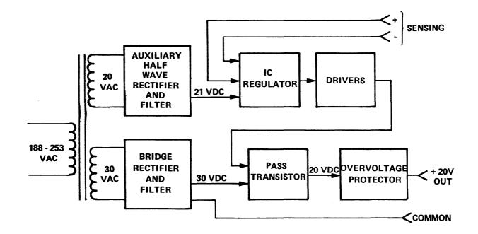
Figure 2-21. +20 Volt Paper Tape Power Supply Block Diagram
