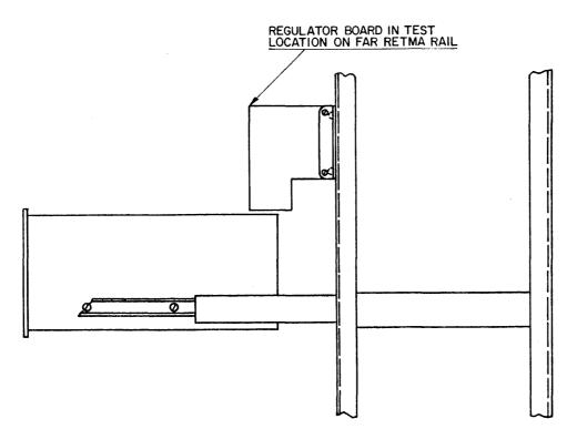
Figure 5-3. Regulator Board Test Location
