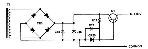
Figure 3-63. Bridge Rectifier and Pre-Regulator
