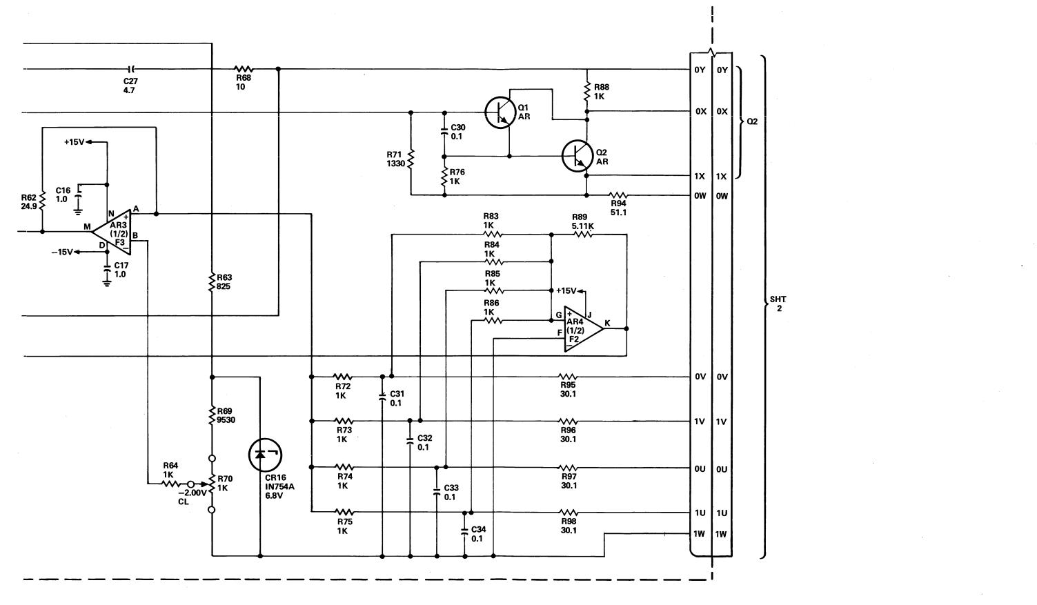
Figure 5-18 Logic Power Supply 4, -2.0 Volt Shunt Regulator Card Schematic (Sheet 2 of 2 continued)
