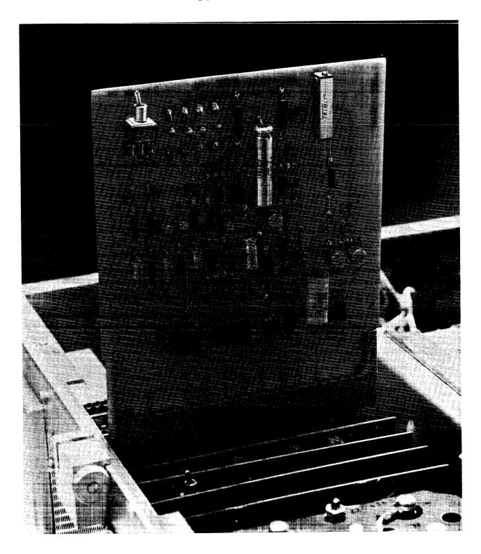
Figure 5-30. Logic Power Supply Card Extension
