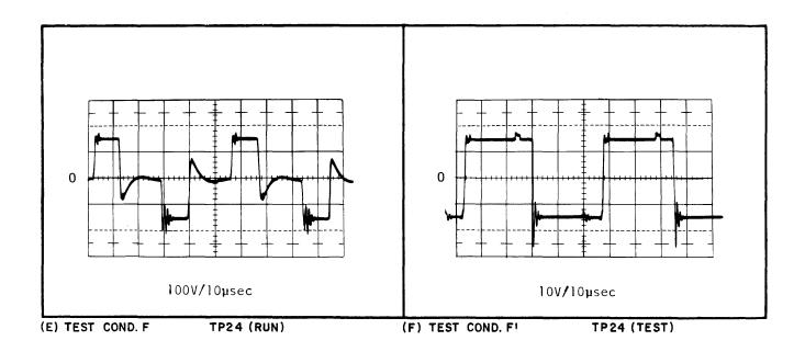
Figure 5-10. Power Board Voltage and Waveform References (Sheet 6 of 13)
