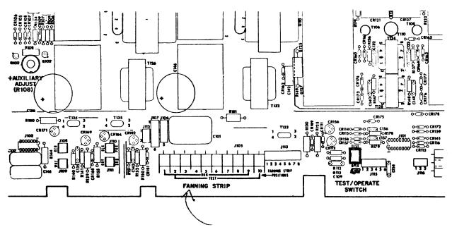
Figure 4-3. Power Board Controls
