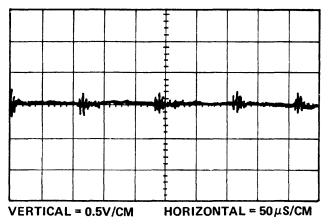
Figure 5-49. High Current Supply Ripple (Measured Across Capacitor C26)
