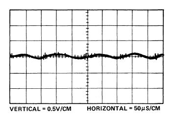
Figure 5-48. High Current Supply Ripple (Measured Across Capacitor C29)
