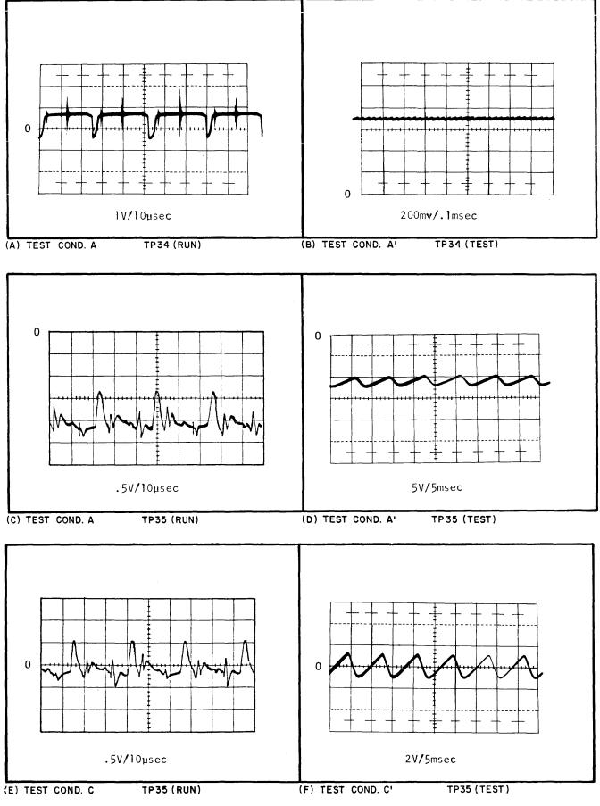
Figure 5-9. Regulator Board Voltage and Waveform References (Sheet 11 of 17)
