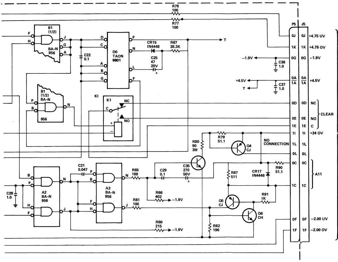
Figure 5-15 Logic Power Supply - 1 & 3, -2.0 Volt Shunt Regulator Card Schematic (Sheet 1 of 2 continued)
