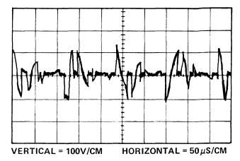
Figure 5-45. Waveform at Commutating Inductor (Measured Across Inductor L2 in Inverter)
