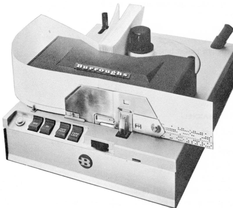
Figure 9.02.13-2 Punching Unit Edge Punched Cards
