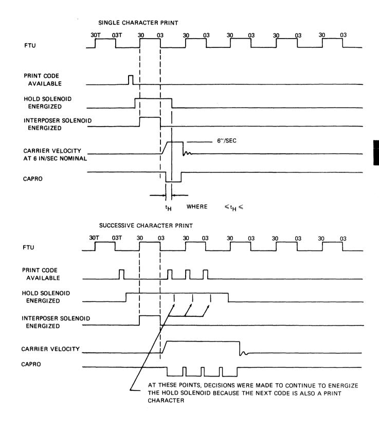
FIG. IIC-138 RELATION OF CARRIER PORT SOLENOIDS TO FTU DURING PRINTING
