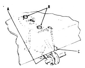
Fig. IV-25 30 CPS PULSE GENERATOR BELT TENSION
