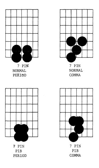
FIG. IIC-130 7 PIN PRINT HEAD PERIODS & COMMAS
