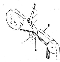
Fig. IV-23 60 CPS CARRIAGE DRIVE BELT TENSION ADJUSTMENT
