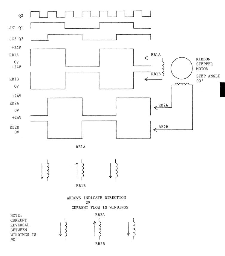
FIG. IIC-121 RIBBON STEPPER MOTOR CONTROL TIMING
