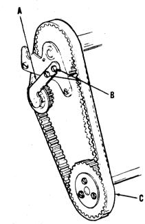
Fig. IV-24 60 CPS PRINT SHAFT BELT TENSION
