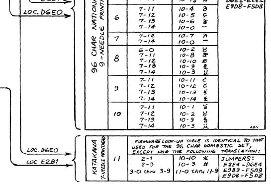
FIG. IIC-126 CHARACTER GENERATOR CODE SETS
