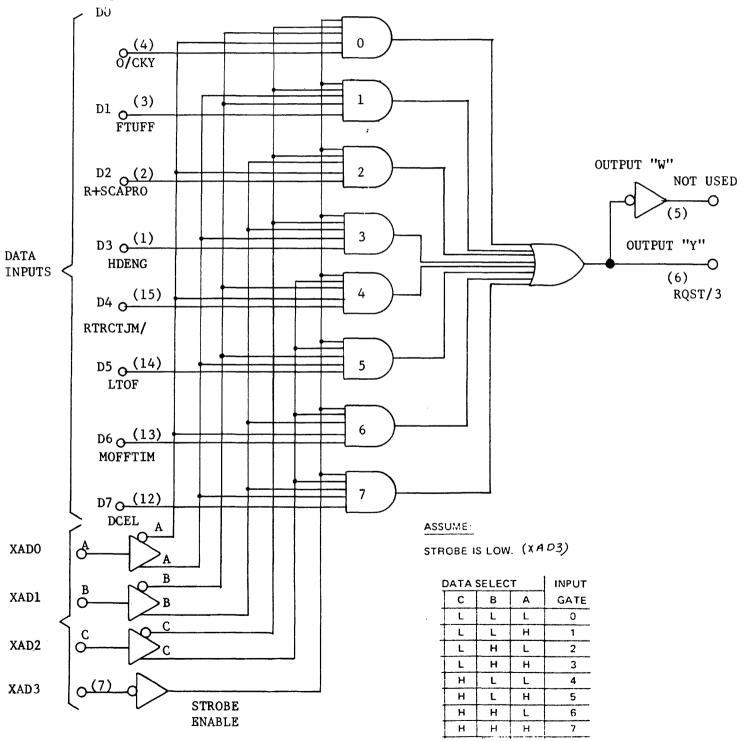
FIG. IIC-108 DATA SELECTOR MULTIPLEXER
