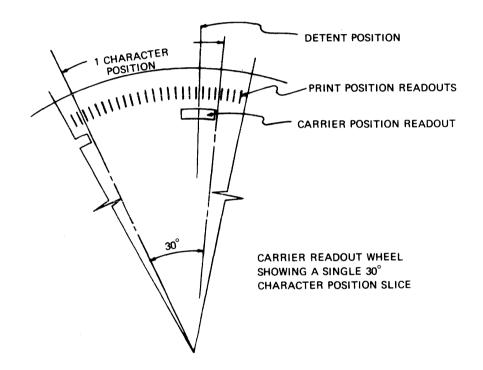
FIG. IIC-136 RELATION OF CAPRO AND PPRO ON CARRIER READOUT ASSEMBLY
