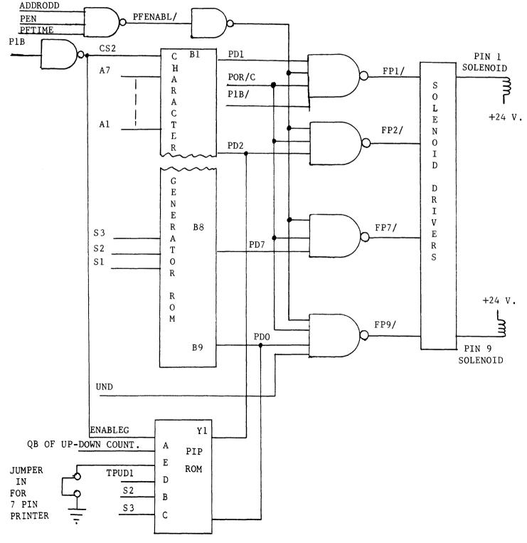
FIG. IIC-133 PRINT FIRE ENABLE GATING & PIP LOGIC
