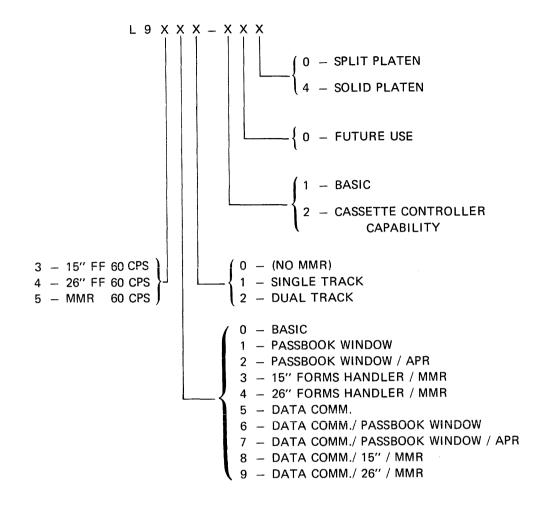
FIG. IIC-92 L9000 STYLE CONFIGURATOR
