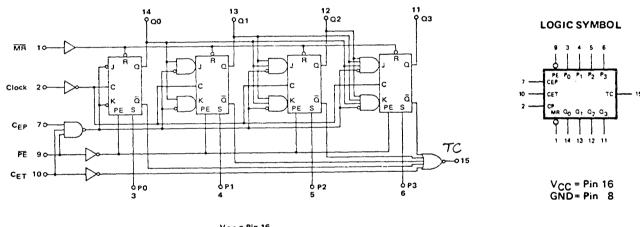
V<sub>CC</sub> = Pin 16 GND = Pin 8
