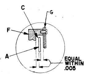
Fig. IV-29 CARRIER POSITION READOUT ADJUSTMENT
