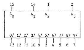
FIG. IIC-106 ONE OF TEN DECODER
