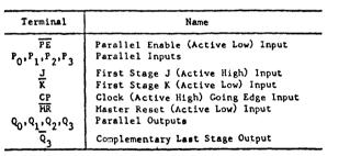
FIG. IIC-112 FOUR BIT SHIFT REGISTER
