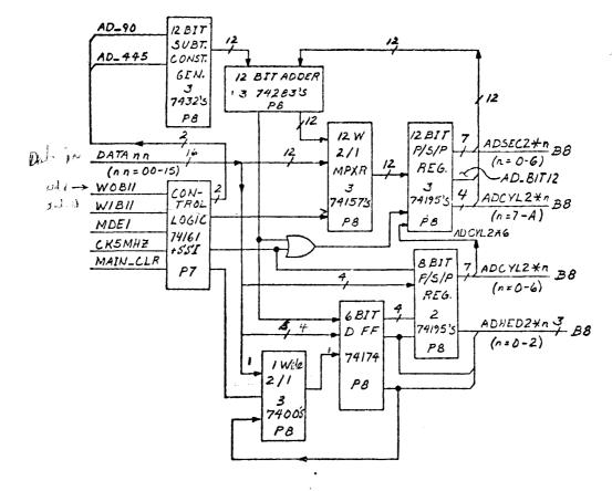
Figure 1-7. Address Decoder
