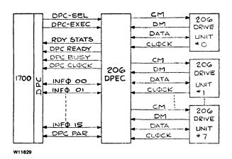
Figure 1-2. System Block Diagram
