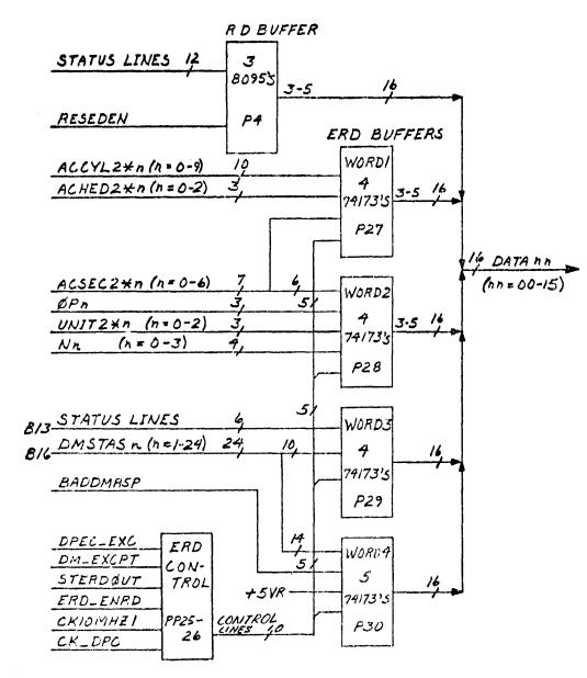
Figure 1-18. RD and ERD Logic
