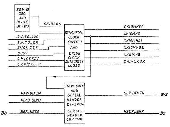
Figure 1-13. Main Clock and Data Sync Logic
