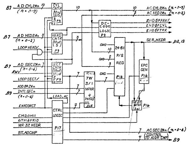
Figure 1-8. Address Counter, Register and EPC Generator
