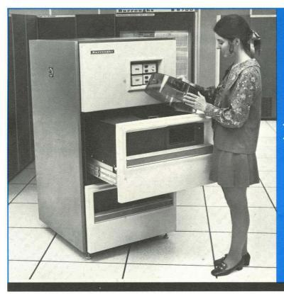
Burroughs B 9484-3 Disk-Pack Memory System Single Data Access, Dual Drive, Magnetic Actuator
