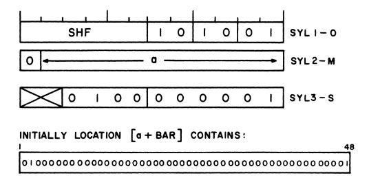
Single, right, arithmetic, end-around shift the contents of the location specified by [a + BAR] 1 position, and store the result (0110  $\iff$  0) in the top of the stack.
