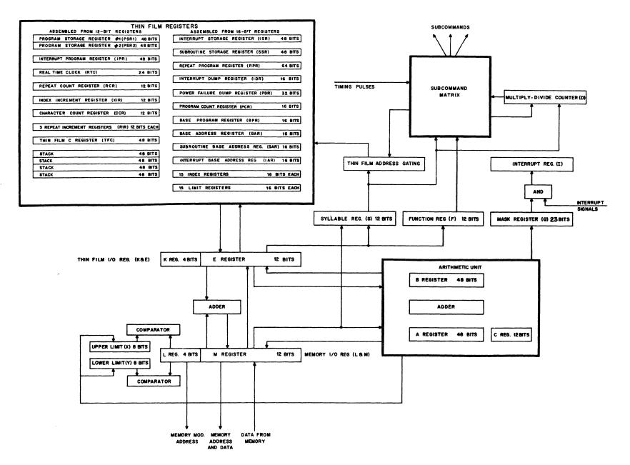
Figure 1-2. Computer Module Block Diagram
