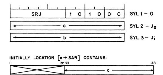
First save the contents of the BAR, BPR, and PCR in the thin film SSR register, then load the BPR and PCR with "C". The next instruction executed will be the contents of the location specified by C, since the PCR now contains "C". Increment the BAR by "b", and load index register #15 with "C" - (BAR + "b").
