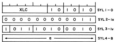
Decrease the contents of index register #10 by 3; compare the new contents of index register #10 with the contents of limit register #2, and if the contents of the index register are  $\geq$  to the contents of the limit register, take the next instruction from (unconditional transfer to) the location specified by [a + BPR]; otherwise, continue in sequence. SER - Store External Requests - 21
