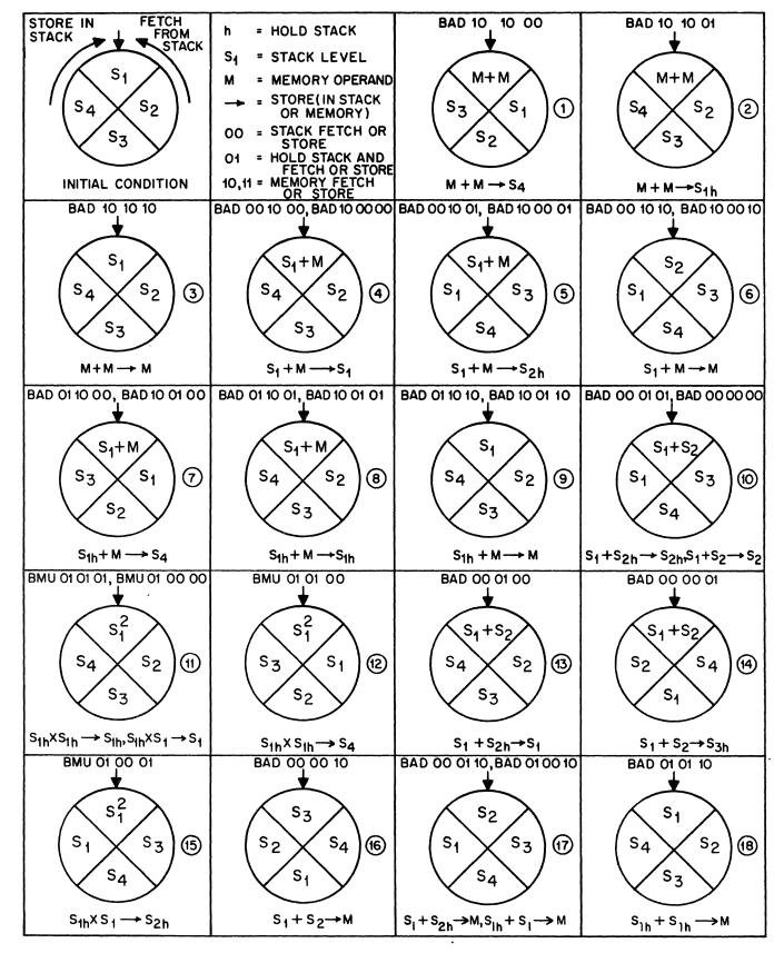
Figure 2-1. Operation of the D825 Operand Stack
