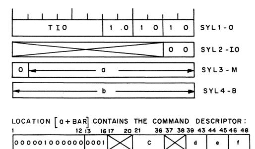
Transmit the Command Descriptor found in memory location [a + BAR] to the lowest-numbered non-busy I/O Control Module. If no I/O Control Modules are available, take the next instruction from the location specified by [b + BPR]. Otherwise, continue in sequence, while the I/O Control Module takes over execution of the command as follows:
