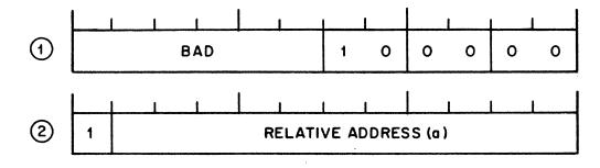
Second level (and subsequent level) absolute addresses are stored in bits 33 through 48 of the 48-bit memory word, and bit 32 is the  $I_A$  bit.
