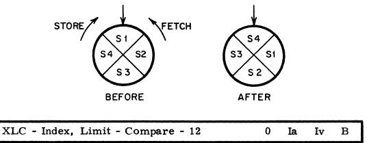
Increase or decrease the contents of the index register specified by bits 5 thru 8 of  $A_2$ , by the amount specified in  $A_1$ . Then compare the contents of this index register with the contents of the limit register specified by bits 9 thru 12 of  $A_2$  for the condition(s) indicated by bits 2 thru 4 of  $A_2$ . If the condition(s) is (are) true, take the next instruction from the location specified by  $A_3$ ; otherwise, continue in sequence.
