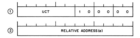
In all cases where a branch is used, the first syllable of the 48-bit memory location thus addressed <u>must</u> be the operator syllable of the next instruction to be performed. When a branch is made, the program count register (PCR) is automatically loaded with the address of the branch. **T-THIN FILM ADDRESS SYLLABLE**
