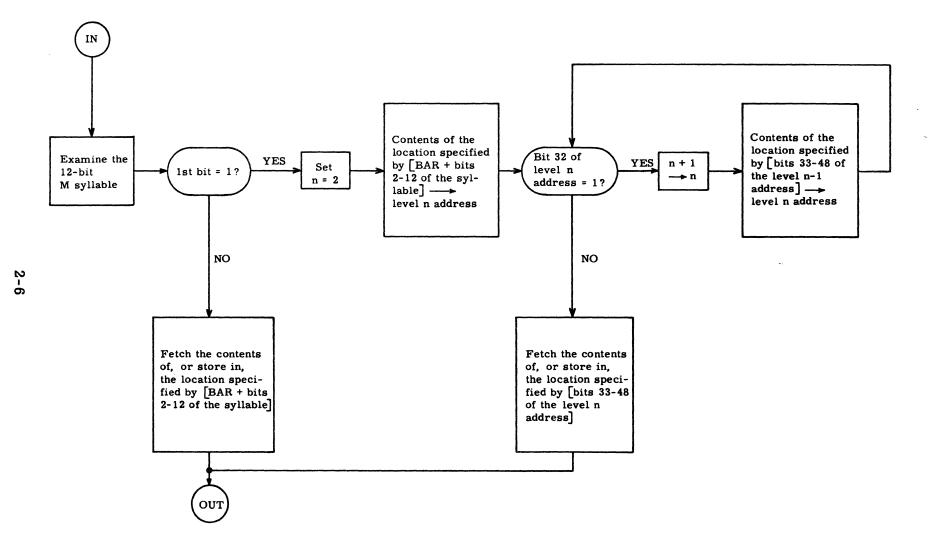
Figure 2-2. Flow Chart of Indirect Addressing
