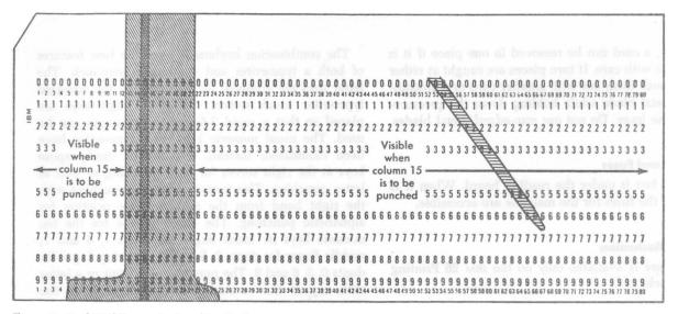
Figure 6. Card Visibility at the Punching Station
