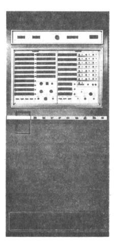
Figure 4-15. Controller-Comparator-Message Processor C-7122/GYK-10 (Message Processor Module On Right Side of Cabinet)
