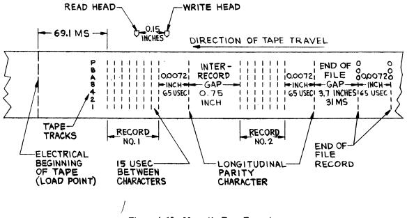
Figure 4-13. Magnetic Tape Format
