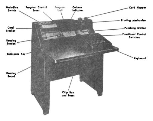
Figure 4. IBM 26 Operating Features
