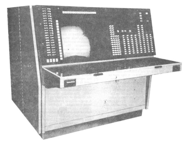
Figure 4-23. Data Display Console OJ-5/GSA-51A
