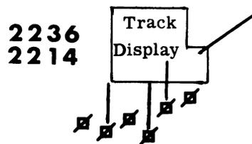
The Assigned SIF code (if any) is displayed in the D characters of a Track SIF Display. The Computer SIF code (if any) is displayed in the E characters. The meaning of these terms is discussed below.
