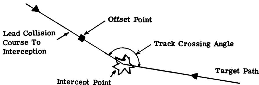
Figure 10-12. Front Lead Collision and Cutoff Attacks
