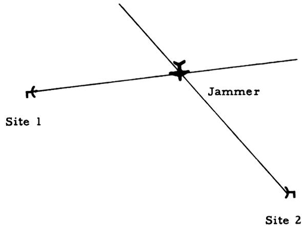
However, when there are two or more jamming aircraft in the system, not all strobe intersections actually represent locations of jammers. One strobe may be from one aircraft and the other from a second aircraft. The intersections of the strobes in such cases are called ghosts. Should the SATCUop incorrectly distinguish the azimuth at which a jammer is located, a false strobe will result. The illustration below shows an example of valid and ghost intersections and a false strobe.
