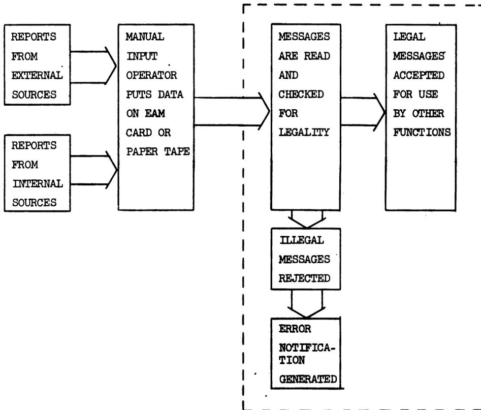
**NOTE:** The manual inputs function is shown enclosed by the broken line. Specific reports and uses are identified in Table 2-1.
