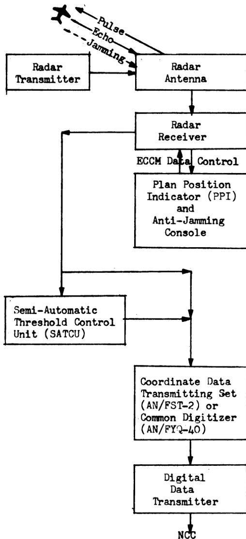
Search radar transmits pulse and picks up reflected signal from target. Also picks up jamming signal, if aircraft is using ECM.
