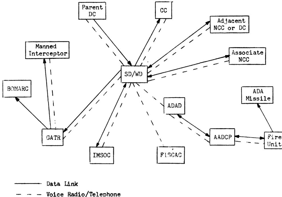
Figure 10-28. Weapons Communication Interface Diagram
