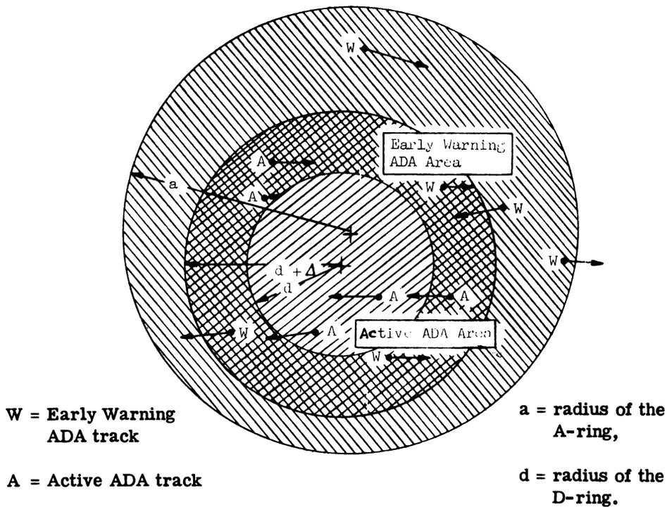
Figure 10-29. Examples of Early Warning ADA and Active ADA Tracks
