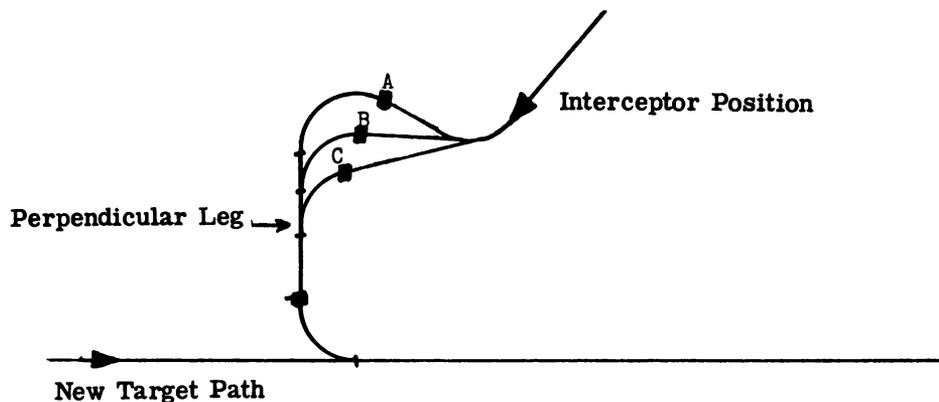
Figure 10-11. Turn Restriction for the Double-Offset Attack
