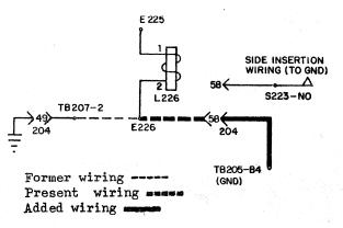
INSTALLATION REQUIREMENTS: This change should be made at the next P.M. attention or must be made whenever the component unit is replaced with one containing the new wiring. (The machine should be marked indicating that this change has been made.)
