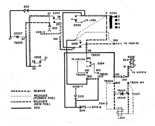
INSTALLATION REQUIREMENTS: This correction should be made when excessive failures of the lane switches are encountered. This correction requires installation of CI1008. (Note step 8 of procedure.) Installation of CI1024 is recommended for improved operation.
