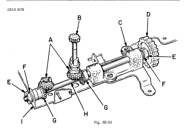
The F2000 gear box is basically the same as the F1000 with the following exceptions. The Tab and Return spindles are mounted on the back plate of the gear box and each is individually driven from a common drive shaft. The Tab and Return spindles are supported by needle bearings. Pulley D is belt driven from the magnetic clutch. Rotation of pulley D results is rotation of gears G through their common shaft H. Gears G drive gears A.
