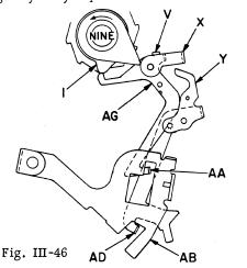
When an amount greater than nine 1s accumulated during the add portion of the cycle, follower arm AG will ride over the high point of carry cam I, releasing carry latch Y as before to position lip AD forward to align with the cutout in the lower side of hatchet AB. Since follower arm
