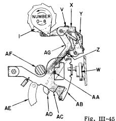
If the amount on a pinion has not exceeded eight (8) during the add portion of the cycle, hatchet AB will be limited at point AC by ear AD on carry latch Y. In this position the "A" pads of the printed circuit board are bridged by the carry wiper in this column.
