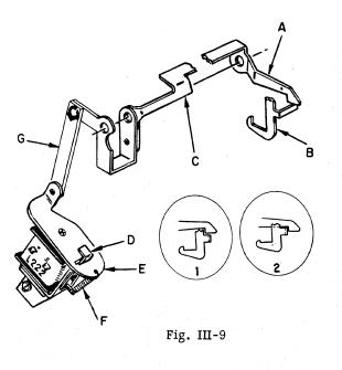
When solenoid L222 is de-energized, spring F urges clapper E against link G which rocks bail C to position hook A over the ear of trip bail B and thereby prevents drive trip. When solenoid L222 is energized, clapper E through link G and bail C raises hook A to allow drive trip bail B to move forward and release the clutch dog release arm.
