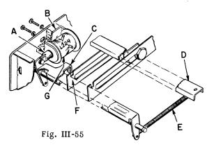
To Adjust, loosen mounting screws and position guide brace D laterally as required. Reason: To ensure a full hold of add rack extensions F with the product accumulator pinions.
