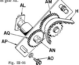
Coupler member AL supplies constant power to the components unit clutch drive shaft. The coupler member is pinned to shaft AN which is turned by gear AQ from gear AM. Gear AM is driven by belt H from pulley I.
