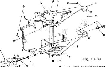
(NOTE: In some cases it may be necessary to reposition the right hand disks slightly). Retighten screws K and recheck alignment. (b) Loosen screws H and turn eccentric I on the left hand clutch assemblies to align left hand disks B with the pins in platen P.
