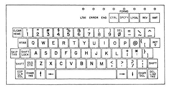
Figure 4-1. U.S. Typewriter Keyboard, ASCII
