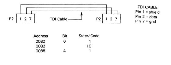
For data set interface use two data set cables and a data set bypass cable as shown below:
