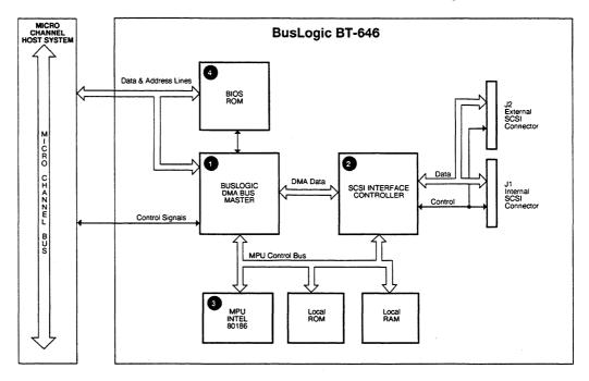
Figure 1-2. Host Adapter Architecture
