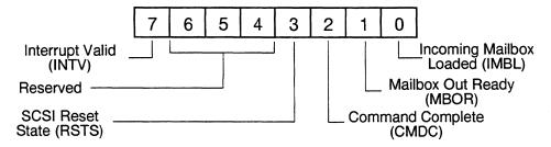
Figure 4-5. Interrupt Register (Read Only)
