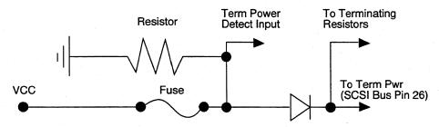
Figure 3-2. Terminator Power Schematic
