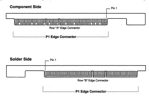
Figure 3-1. Connector Rows on the BT-646 Board Edge
