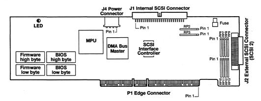
Figure 2-1. The BT-646 Host Adapter Board
