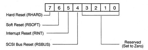
Figure 4-1. Control Register (Write)
