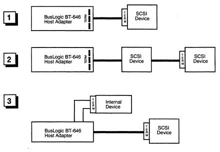
Figure 2-2. SCSI Terminator Configurations
