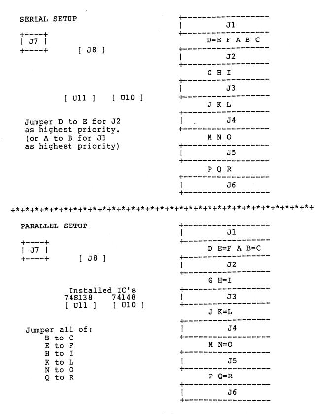
Figure 9-1 Motherboard Bus Arbitration Examples
