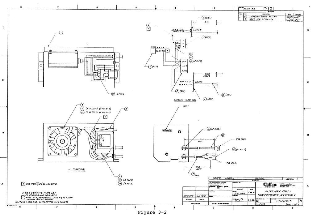
Auxiliary Fan/Transformer Assembly
