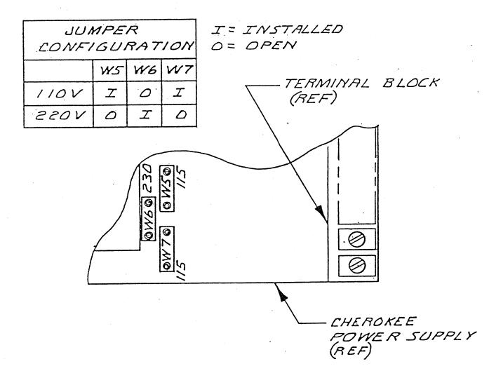
Figure 3-4 Power Supply 110V/220V Jumper Configuration
