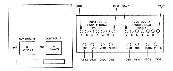
Figure 8-1. 362X Equipment Number Switch and Indicator Panel
