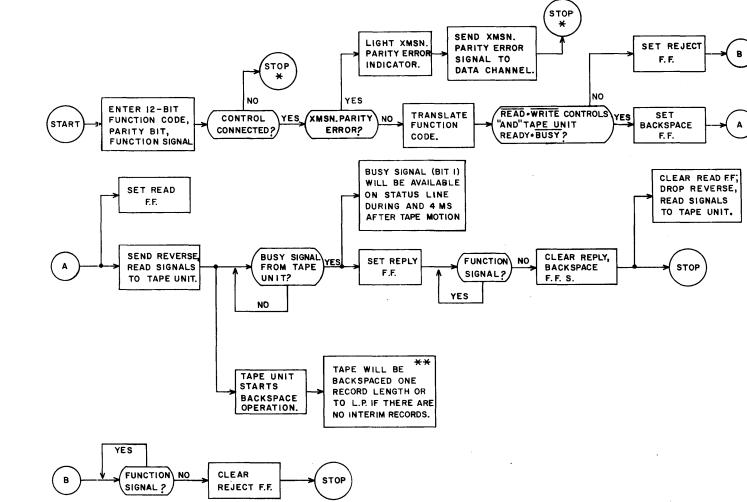
★ INTERNAL REJECT BY COMPUTERXX IF THE BACKWARD FF (JX38/X39)IS SET,<br/>TAPE IS MOVED IN A FORWARD DIRECTION.AFTER 100 µSEC.TAPE IS MOVED IN A FORWARD DIRECTION.
