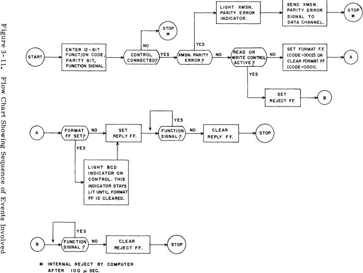
Figure 3-11. Flow Chart Showing Sequence of Events Involved in a Format (0001 or 0002) Operation.
