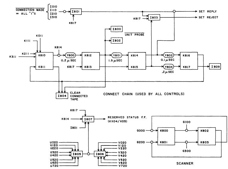
Figure 2-4. Connect Chain, Scanner
