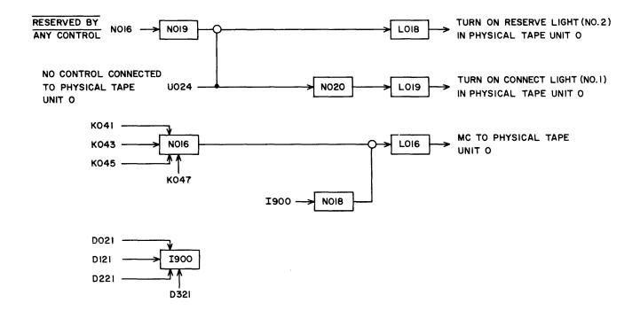
Figure 2-7. MC, Reserve, Connect Light Outputs to Physical Tape Unit 0 (Bank 0).
