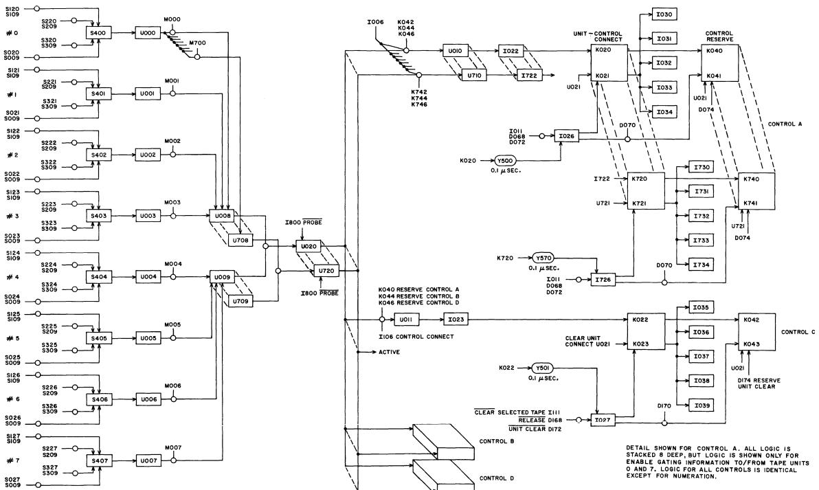
Figure 2-5a. Connect Enable Logic for Bank O
