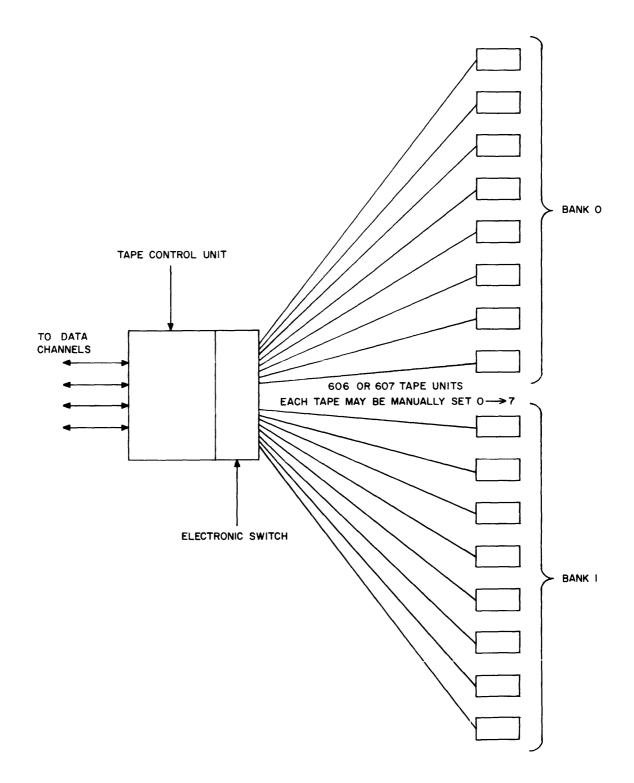
Figure 1-1. 362X Magnetic Tape Controller
