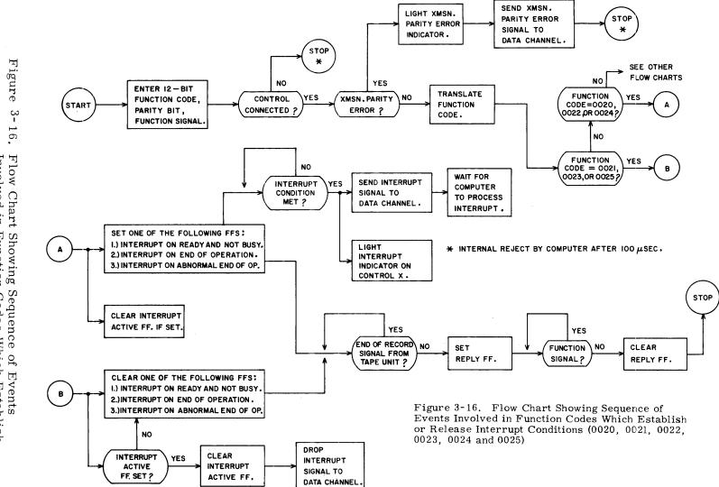
are 3-16. Flow Chart Showing Sequence of Events Involved in Function Codes Which Establish or Release Interrupt Conditions (0020, 0021, 0022, 0023, 0024 and 0025)
