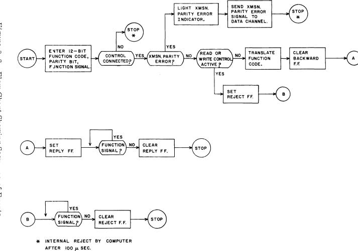
Figure 3-8. Flow Chart Showing Sequence of Events Involved in a Clear Reverse (0040) Operation
