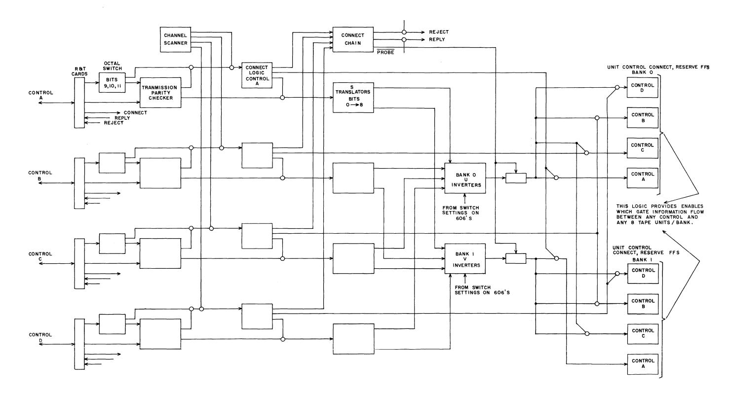
Figure 2-2. Simplified Block Diagram Connect Logic
