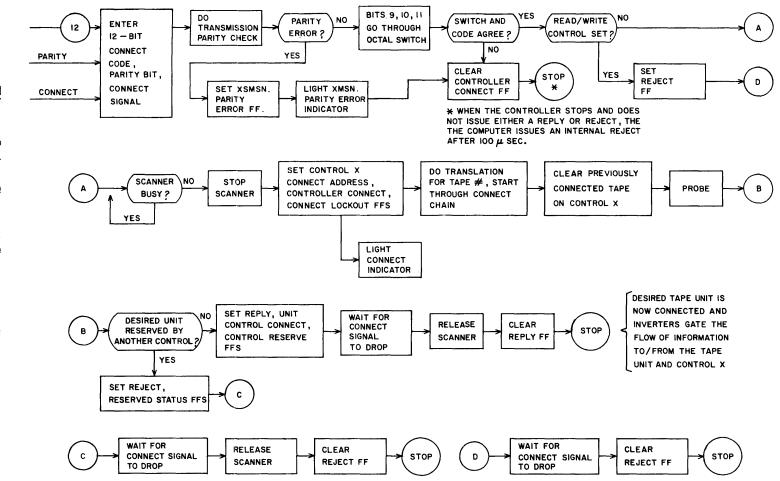
Figure 2-1. Connect Sequence, Control X
