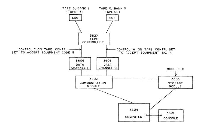
$100_8$  words are stored in storage module 0 at locations 00100-00177. Write them on tape 0, bank 0 (556 density, BCD). Tape 00 is at load point. Also, a record of  $300_8$  words is stored on tape 13 (written in BCD, 556 density). Store the record in storage module 0. starting at location 00200. Tape 13 is also at load point. Rewind both tapes to load point sometime after the Write and Read operations are complete. Halt the program if any of the above operations cannot be executed.
