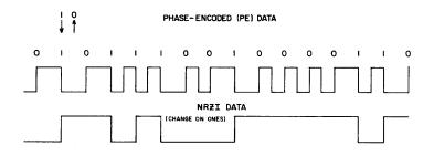
Figure 1-3. NRZI and Phase Bits
