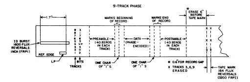
Figure 1-5. Phase Encoded Format
