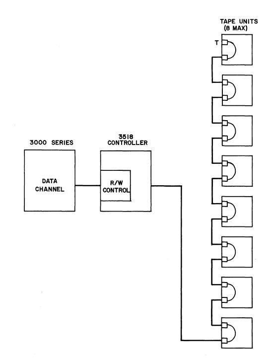
Figure 1-1. Typical Single Channel Configuration
