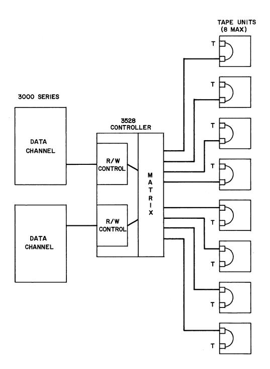
Figure 1-2. Typical Dual Channel Configuration
