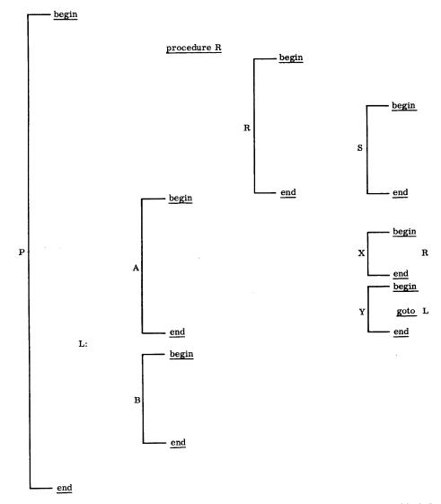
Block P is the program itself; blocks A and B and procedure R are at the same level within P; block S is contained in procedure R; blocks X and Y are at the same level within block A. Block X contains a call to procedure R; block Y contains a jump to label L within the outermost block (the program itself). The changes in the stack and display entries can be visualized as follows:
