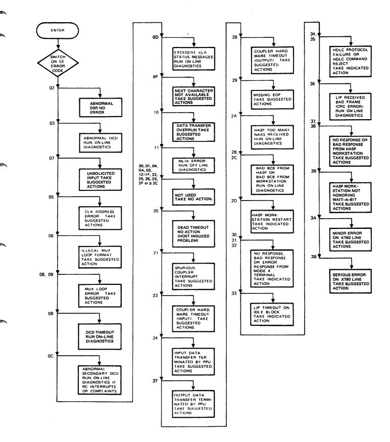
Figure 2-1. Flowchart for CE Error Code DDLT
