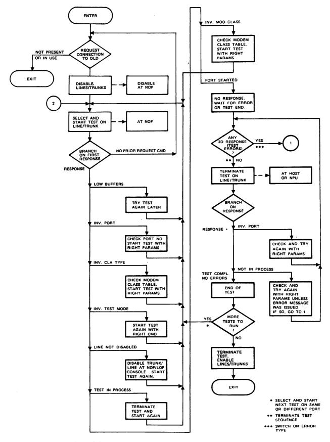
Figure 4-2. Flowchart for On-Line Diagnostic DDLT (Sheet 1 of 2)
