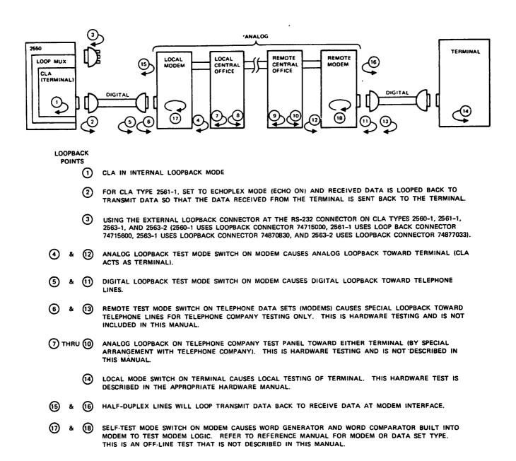
Figure 4-3. Loopback Points for Test Selection
