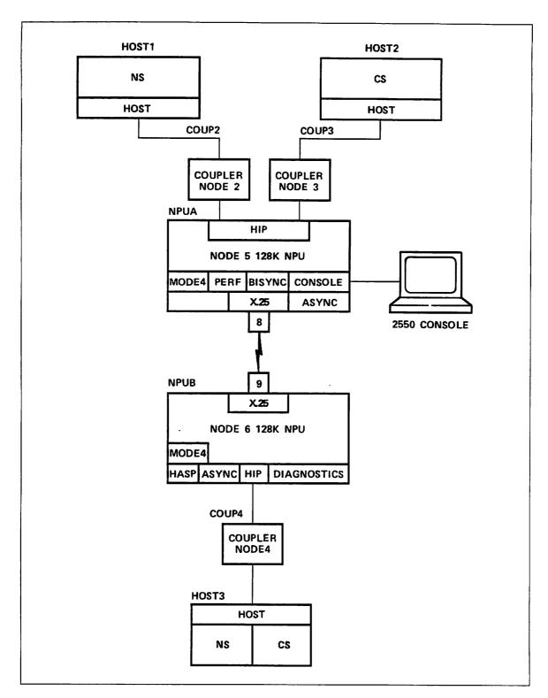
Figure 7-6. Network Configuration - Example 2
