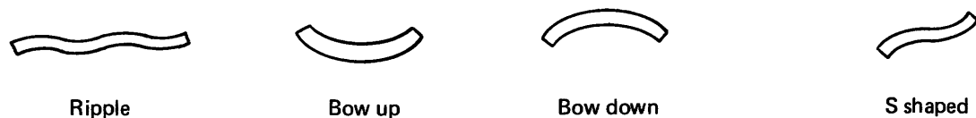
Figure 9-8. Aerodynamic effects on disk
