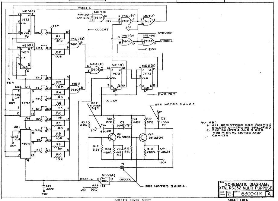
Figure 7. Schematic Diagram (Sheet 1)
