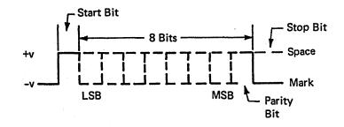
Figure 3. Serial Input Data
