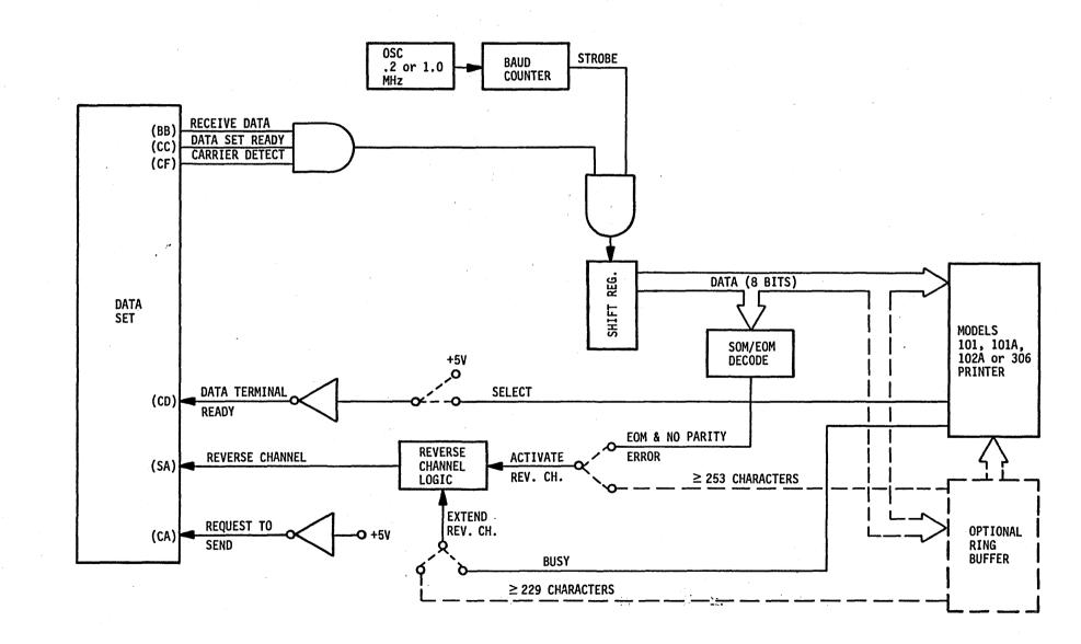
Figure 1. RS232 Interface Data Flow Diagram
