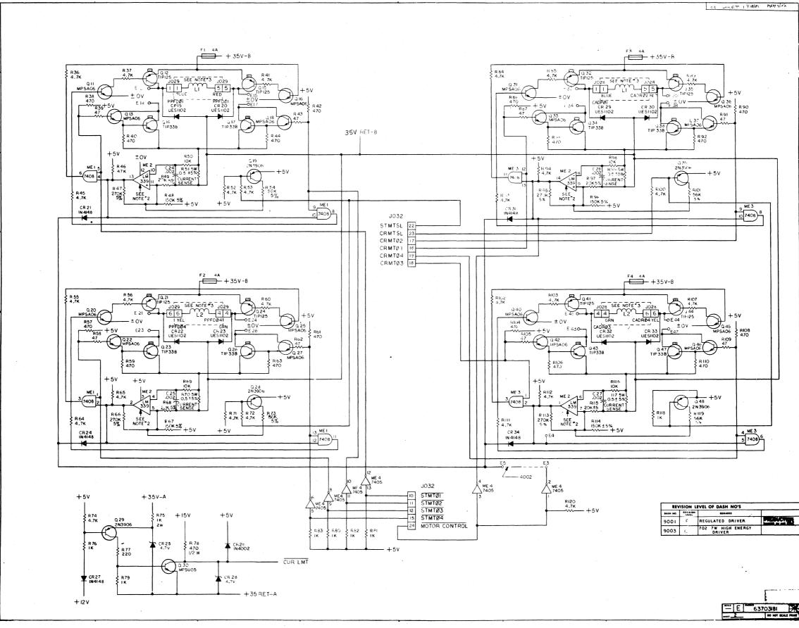
Figure A-4 Schematic Diagram, Power Driver Board (Sheet 2 of 2)
