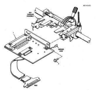
Figure 7-6 Removal/Replacement, Video Amplifier Assembly
