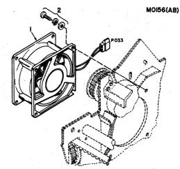
Figure 7-14 Removal/Replacement, Fan Assembly
