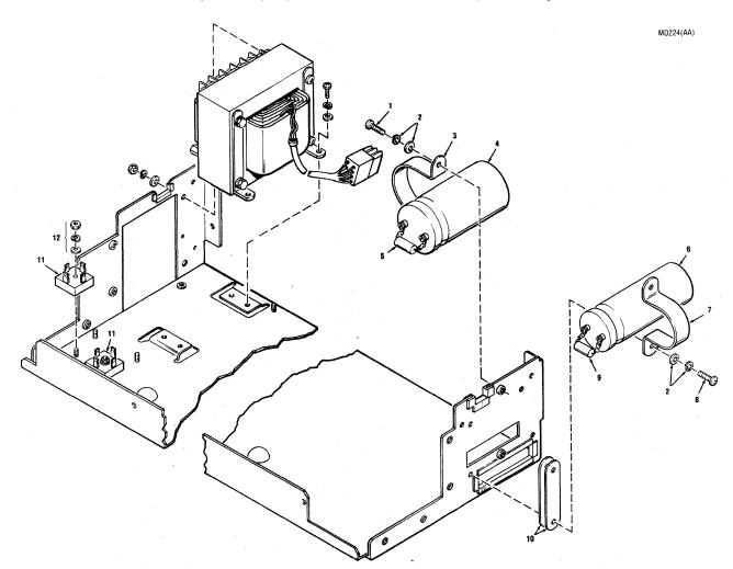
Figure 7-13 Removal/Replacement, Capacitor/Diode Bridges
