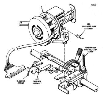
Figure 7-2 Removal/Replacement, Print Head Assembly
