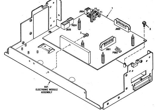
Figure 7-15 Removal/Replacement, Logic Board Assembly
