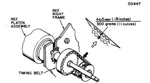
Figure 6-5 Paper Feed Timing Belt Adjustment
