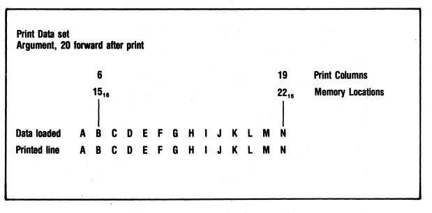
Figure 2-7 Printing Simple Line of Characters, Example 1
