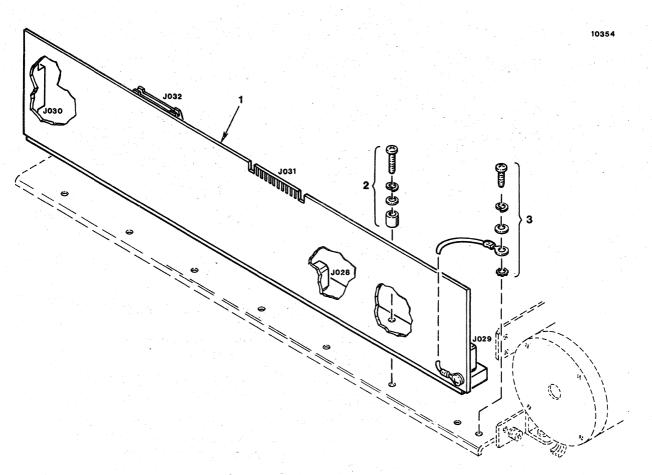
Figure 7-4 Removal/Replacement, Power Driver Board Assembly
