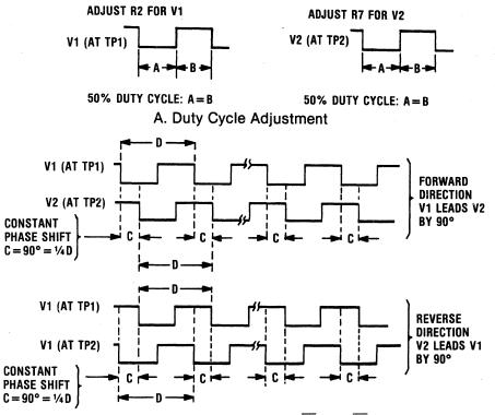
B. Phase Adjustment of  $\overline{V1}$  and  $\overline{V2}$
