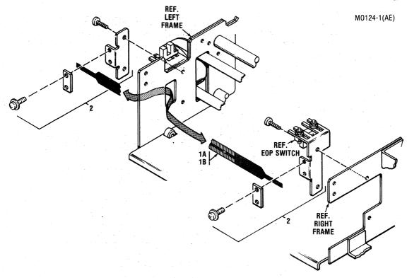
Figure 7-5 Removal/Replacement, Timing Fence Assembly
