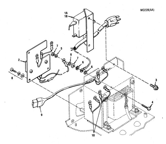
Figure 7-12 Removal/Replacement, Primary Voltage Assembly
