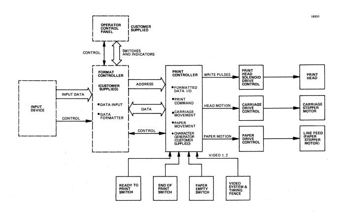
Figure 1-3 Basic Printer Block Diagram
