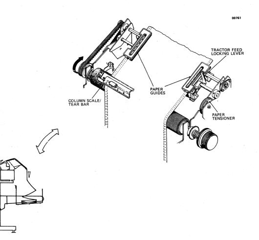
Figure 3-6 Loading paper, Bottom Tractor Feed
