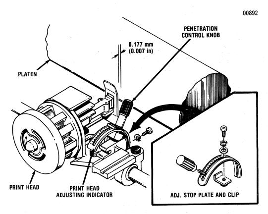
Figure 6-1 Penetration Adjustment
