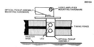
Figure 6-9 Vertical Alignment Optical Pickup
