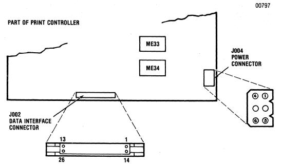
Figure 2-2 Data Interface and Power Connector Location
