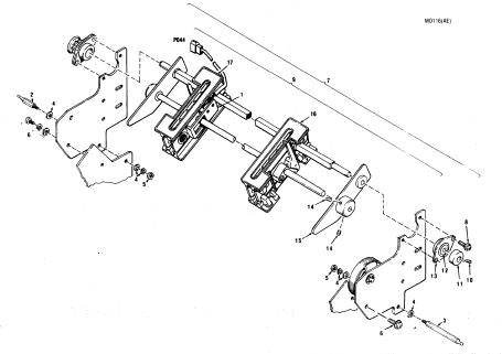
Figure 7-11 Removal/Replacement, Tractor Drive Assembly and Left/Right, Pin Feed Tractors
