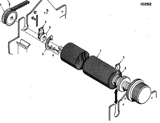
Figure 7-10 Removal/Replacement, Platen Assembly
