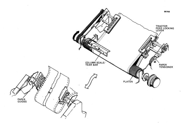
Figure 3-5 Loading Paper, Rear Tractor Feed
