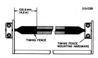
Figure 6-2 Timing Fence Adjustment
