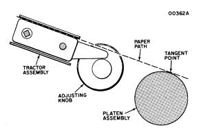
Figure 6-8 Paper Tension Adjustment
