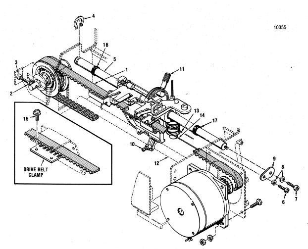
Figure 7-7 Removal/Replacement, Carriage Assembly
