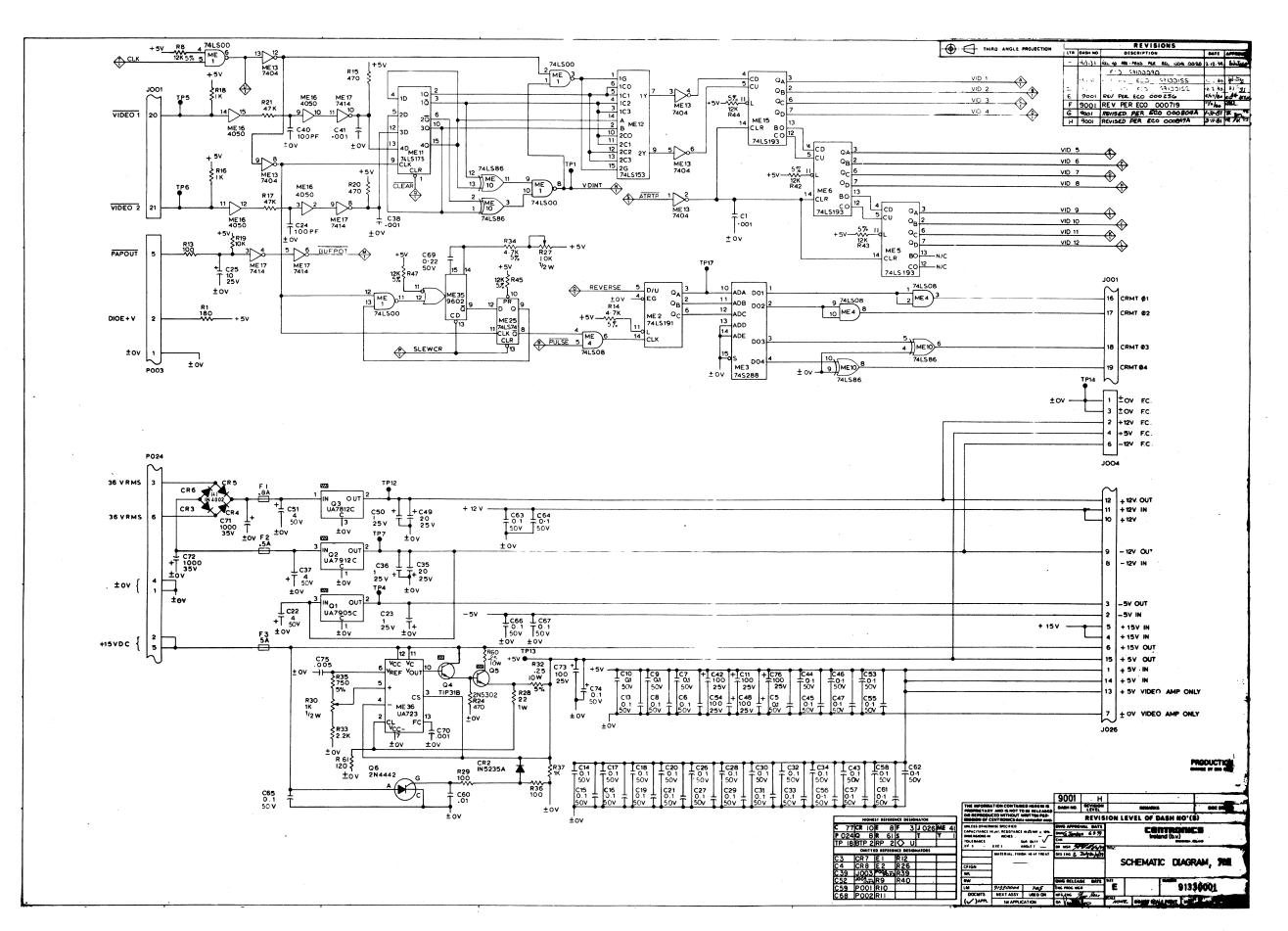
Figure A-2 Schematic Diagram, Model 705 Logic Board (Revision E, Sheet 2 of 2)
