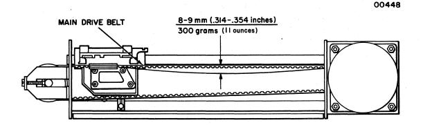
Figure 6-4 Main Drive Belt Adjustment
