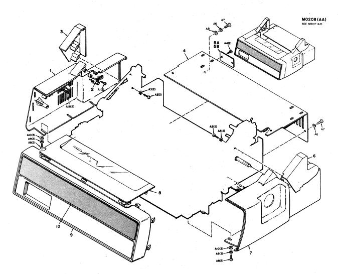
Figure 7-1 Removal/Replacement, Cover Assemblies
