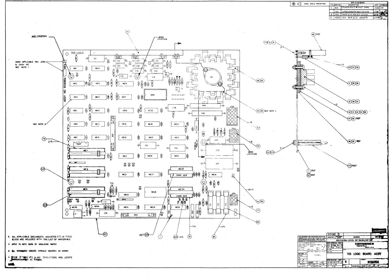
Figure A-8 Assembly Drawing, Model 705 Logic Board (Revision B, -4001)
