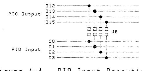
Figure 4-4. PIO Input Rerouting
