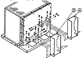
Figure 1-13 Power Supply Mounting
