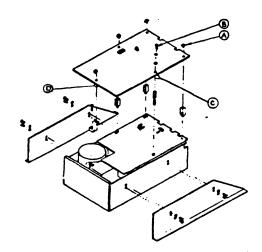
Figure 1-7 Disk Controller with Hard Disk
