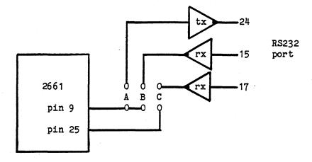
"tx" represents an RS232 transmitter, and "rx" is an RS232 receiver. 24, 15, and 17 are the RS232 connector pin numbers. A, B and C are the locations where jumpers may be installed. This configuration is repeated for each of the four SPC ports, so each port can be jumpered differently.
