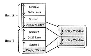
Figure 3-3. Segmented Memory - Dual Host Split Screen Mode
