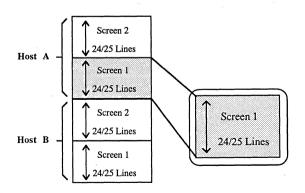
Figure 3-2. Segmented Memory - Dual Host Independent Mode
