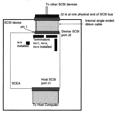
Figure 3-9: Device SCSI port termination
