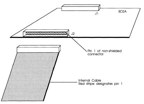
Figure 3-7: Device SCSI port (J2) cable connection
