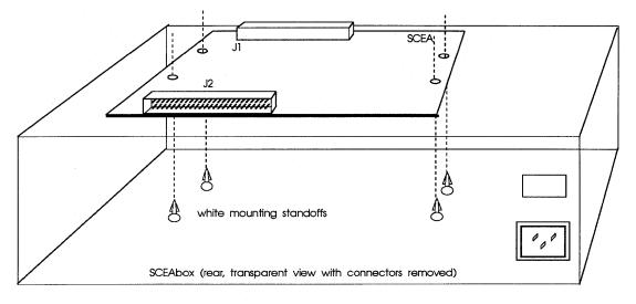
Figure 3-11: Installing the SCEA into the SCEAbox
