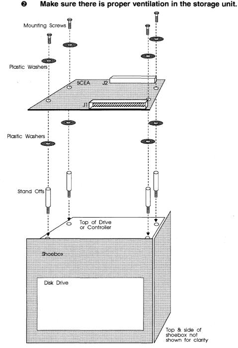
Figure 3-1: Shoebox installation example
