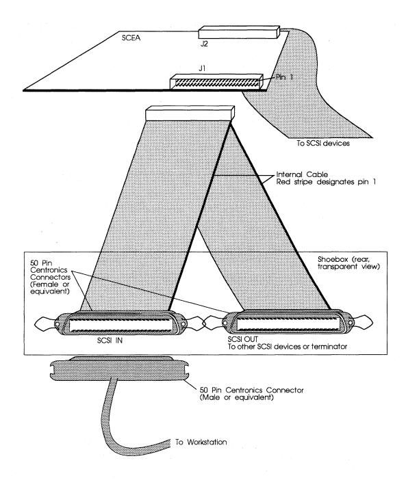
Figure 3-4: Shoebox or Storage Box J1 SCSI connection
