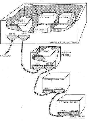
Figure 5: Cabling example from inside Subsystem
