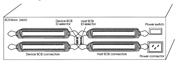
Figure 3-12: Device and Host ID selectors
