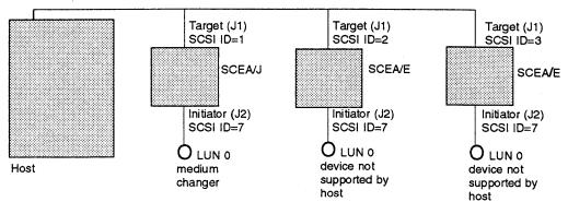
This diagram is for SCSI IDs and LUNs for workstations that do not support LUNs with devices supported by the host.
