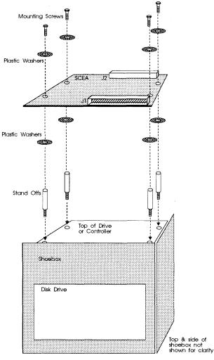
Figure 1: Shoebox installation example
