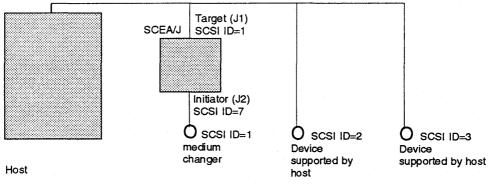
This diagram is for SCSI IDs and LUNs for workstations that do not support LUNs with devices supported by the host.
