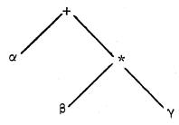
The normal precedence of Algol operators is used to determine how the tree will be constructed. In addition, the "|[]|" construction has precedence just above that of "-," (pg. 47).
