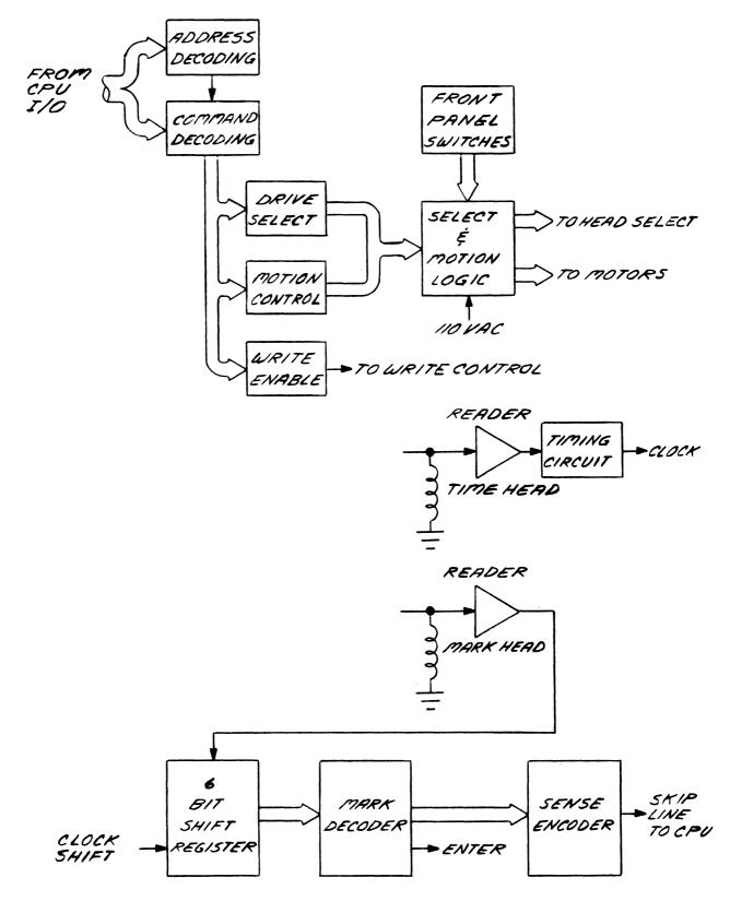
FIGURE 10.4 LINC TAPE BLOCK DIAGRAM: CONTROL, MARK, & TIMING
