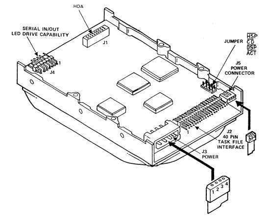
Figure 2. Connectors and Jumpers
