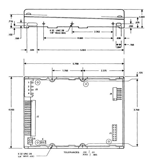
Figure 1. Mounting Configuration
