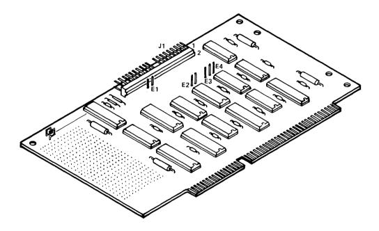
Figure A-2 AT Adapter Card Layout
