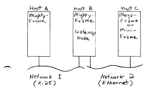
Figure 6-2. Example of An Internetwork Using a MightyFrame as a Gateway
