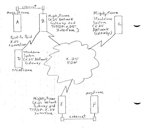
Figure 10-3. Example X.25/Ethernet Internetworking Configuration
