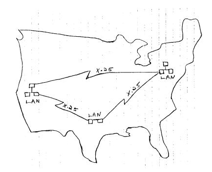
Figure 10-1. Wide Area X.25 Used to Connect LANs.
