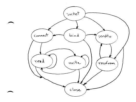
Figure 13-8. State Diagram for UDP Datagram Socket.
