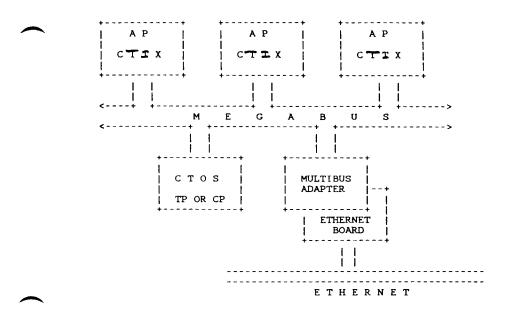
Figure 12-5. MegaFrame Bthernet Configuration Example.
