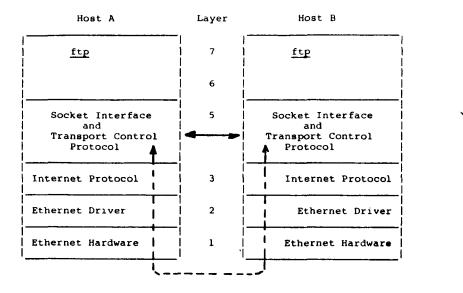
Figure 11-2. Example of How Protocols Communicate
