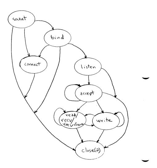
Figure 13-7. State Diagram for TCP Stream Socket. 13-50 CTIX Internetworking Manual (Preliminary) The calling program issues a socket call to AF\_INET (Address Family Internet) to get access to the net.
