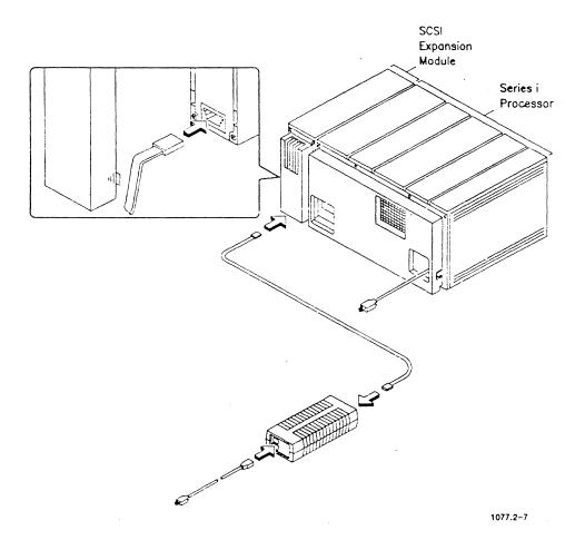
Figure 2-7. Connecting Power to a Series i System
