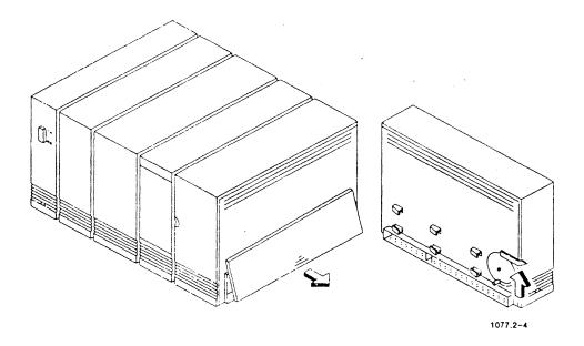
Figure 2-4. Removing the Bus Cap
