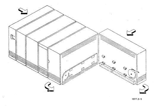
Figure 2-5. Pushing Modules Together
