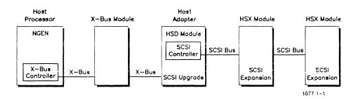
Figure 1-1. System Buses, HSX and HSD Modules
