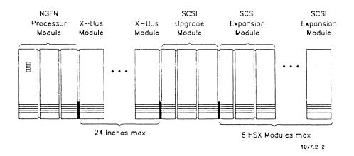
Figure 2-2. Typical NGEN SCSI Configurations
