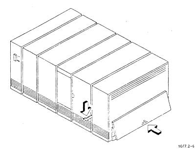
Figure 2-6. Latching Modules Together
