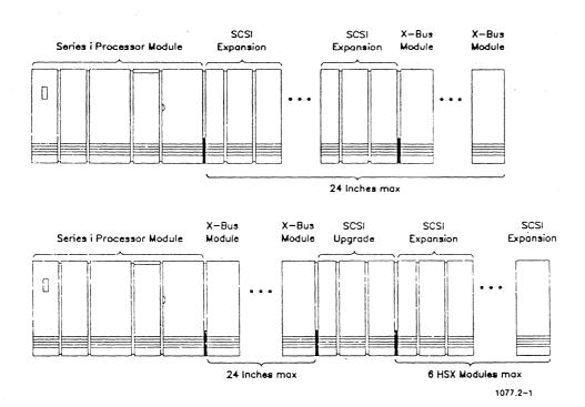
Figure 2-1. Typical Series i SCSI Configurations
